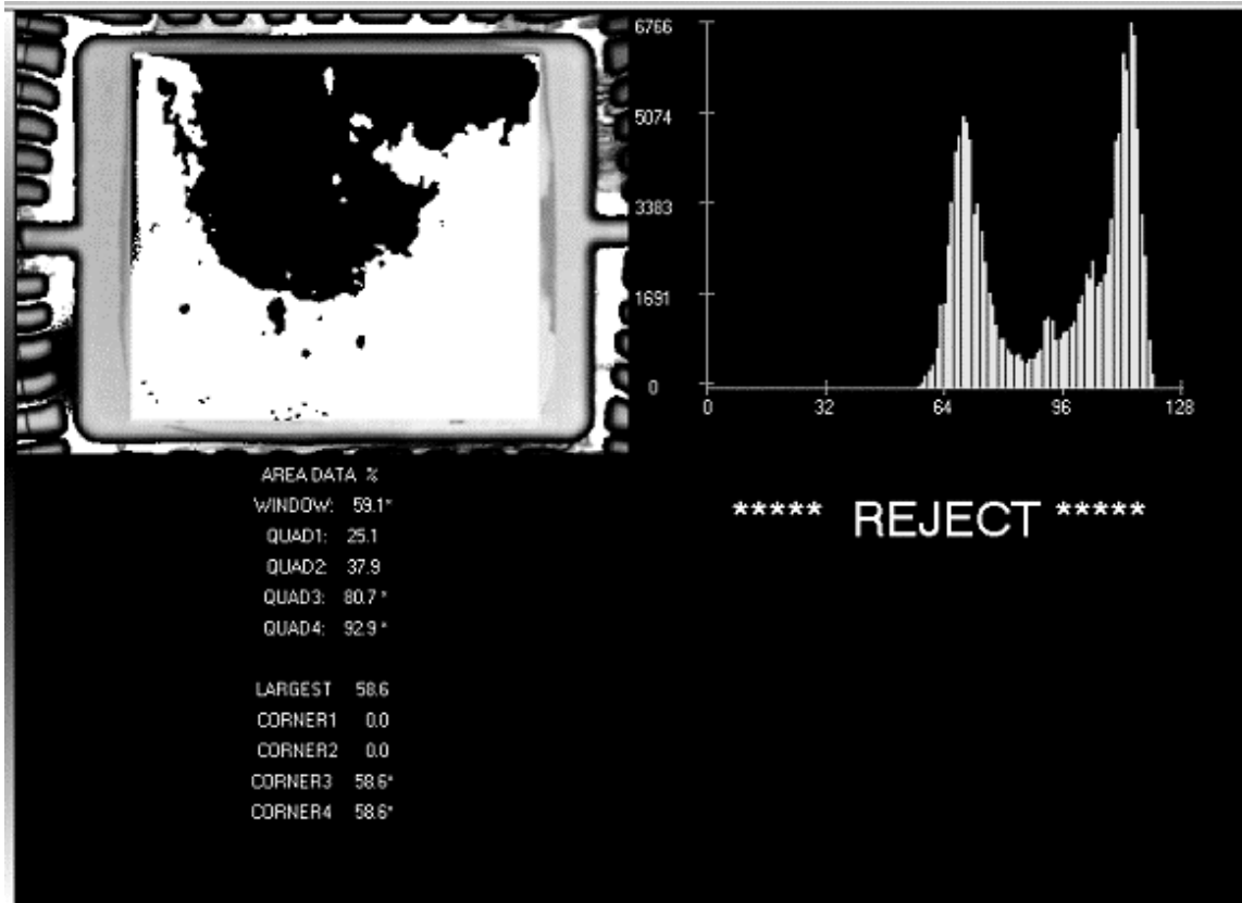
FIGURE 2030-2. Example Automated Method Analysis Report for Die Attach Interface
