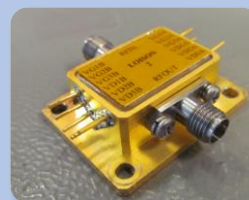
GaN Ka-band PA in a module Product CGY2650UH/C1
