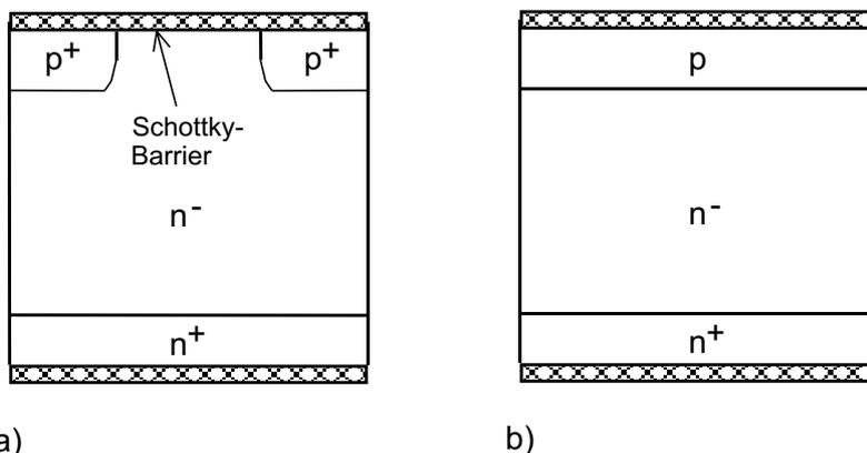
Figure 2.3.4 p-emitter to improve soft recovery behaviour:
