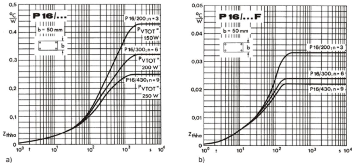
Figure 5.3.6  $Z_{th(s-a)}(t)$  characteristics for different P16 heatsink lengths/length in [mm], number of heat sources  $n$ ; a) in case of free convection with different power dissipation values; b) for forced air cooling
