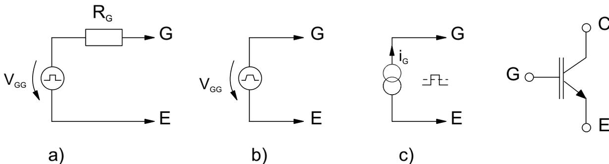
Figure 5.6.1 Gate driving process for MOSFET and IGBT [37]
