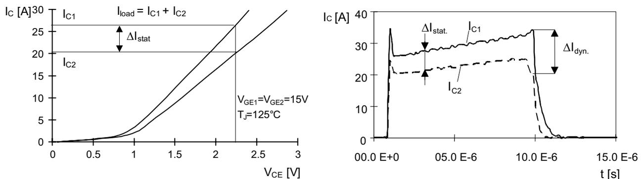
Figure 5.8.1 Stationary current distribution in two parallel IGBT with different output characteristics.
