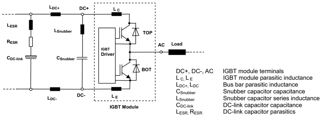
Figure 5.7.13 Simplified equivalent DC link circuit with typical, concentrated parasitic inductances
