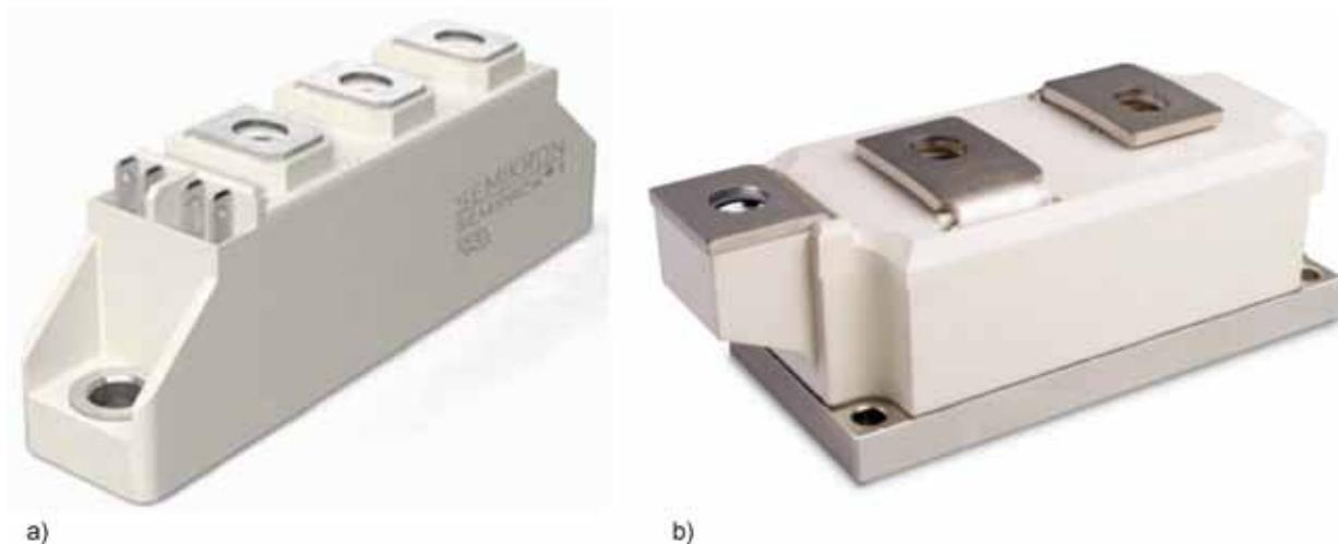
Figure 2.5.36 a) SEMIPACK®1 (soldered chips, soldered / bonded top side, aux. spring contacts)
