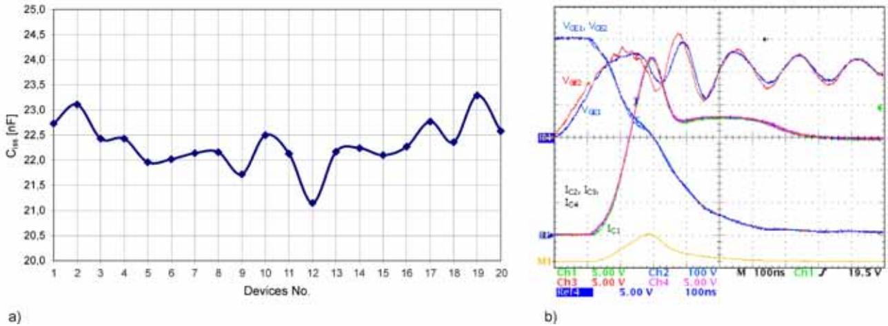
Figure 5.8.5 a) Variation recorded for input capacitance  $C_{ies}$  of a selection of 450 A Trench2 IGBT modules; b) Switching test with 4 parallel modules (turn-on) with an additional 4.7 nF external capacitance between module gate and emitter
