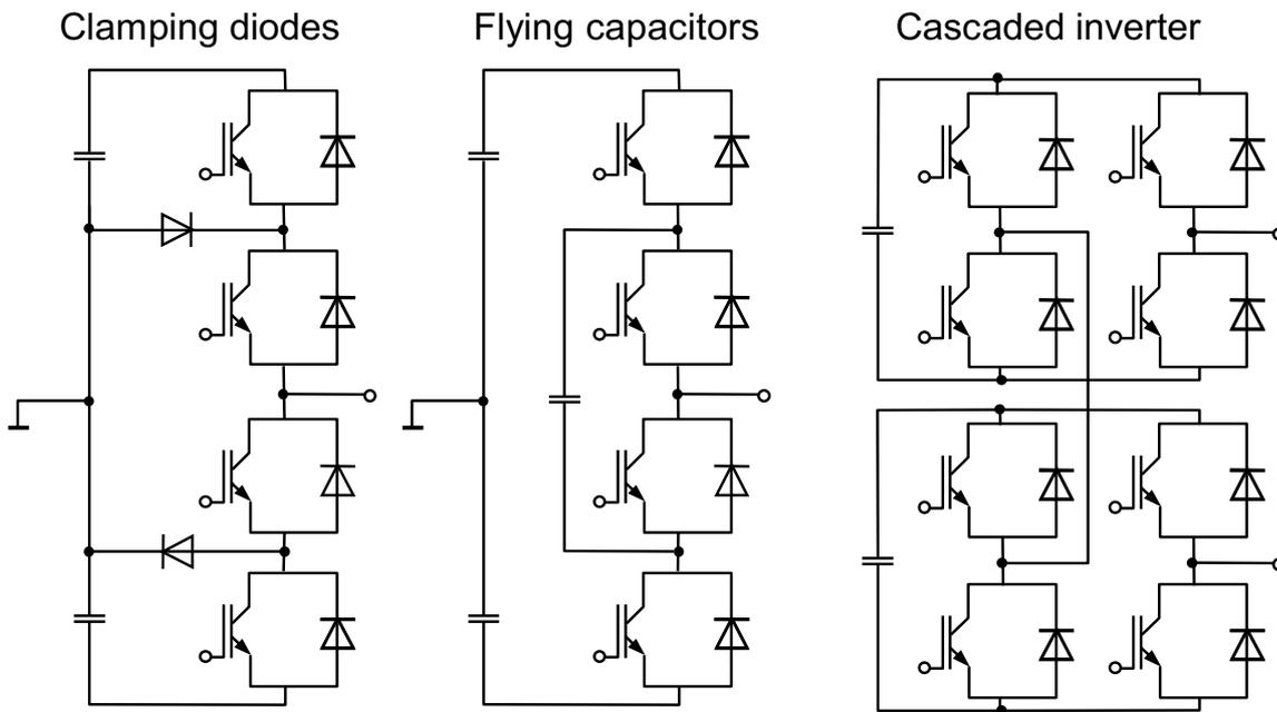
Figure 5.8.17 Examples of IGBT series connection without critical voltage distribution
