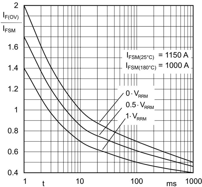
Figure 3.2.7 Overcurrents  $I_{F(OV)}$  permissible in the event of malfunction of a 70 A diode in relation to a surge forward current  $I_{FSM}$  lasting 10 ms under different reverse voltage conditions directly following the last half sine wave; shown over time  $t$ .
