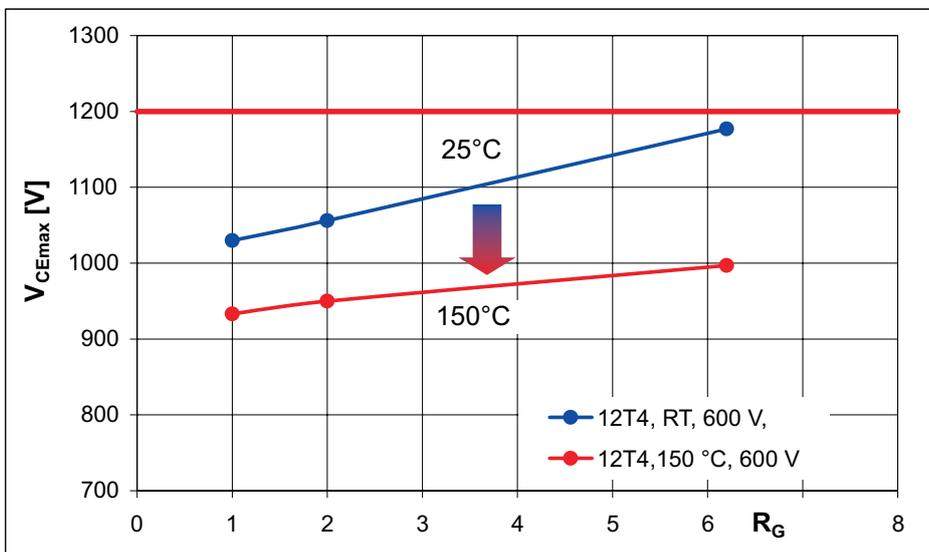
Figure 5.1.2 Voltage load  $V_{CEmax}$  of a 1200 V /400 A IGBT module with T4 chips at chip level at  $V_{CC} = 600 \text{ V}$  and turn-off of  $I_c = 2 \cdot I_{Cnom} = 800 \text{ A}$  and different external gate resistances and temperatures
