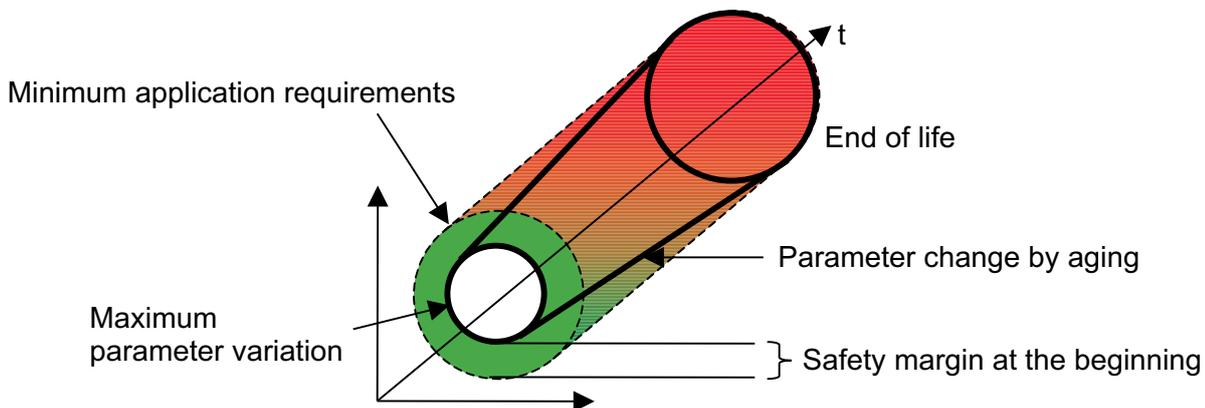
Figure 2.7.1 Design process for reliability. Target: to sufficiently factor in safety and reliability at the beginning of the service life to ensure that product requirements are still met at the end of service life.
