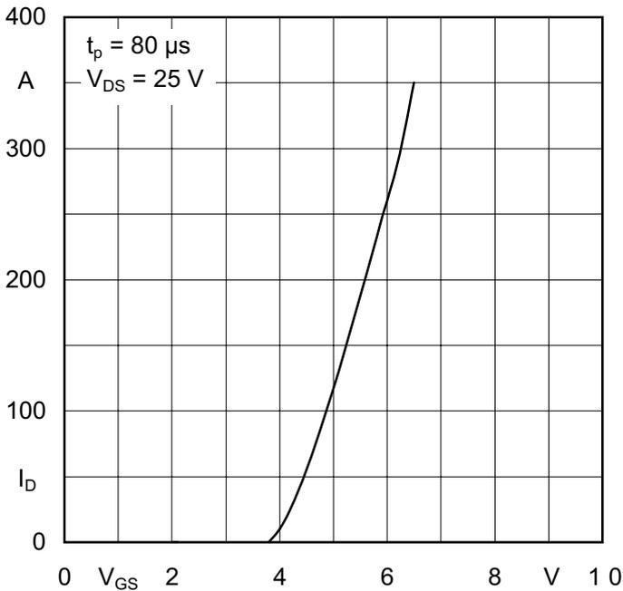
Figure 3.4.7 Typical transfer characteristic  $I_D = f(V_{GS})$ **[Fig. 5] Typical characteristic of ON-resistance versus chip temperature**
