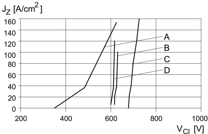
Figure 5.7.17 Static characteristics of selected Zener elements
