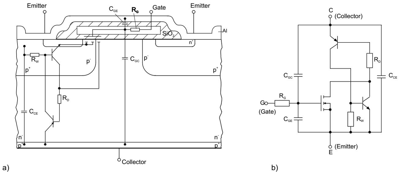
Figure 2.4.4 IGBT cell (NPT structure, planar gate) including the key parasitic elements;
