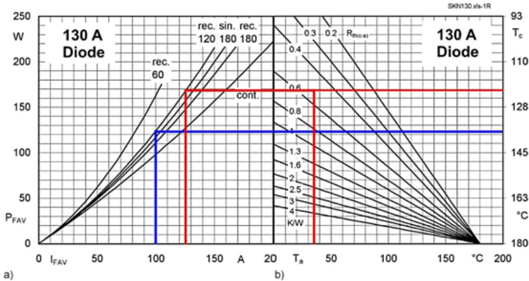
Figure 4.1.2 a) Mean forward power dissipation  $P_{FAV}$  over mean forward current  $I_{FAV}$  for different current waveforms; b) Case temperature  $T_c$  over ambient temperature  $T_a$ ; the parameter is the thermal resistance case-to-air  $R_{th(c-a)}$
