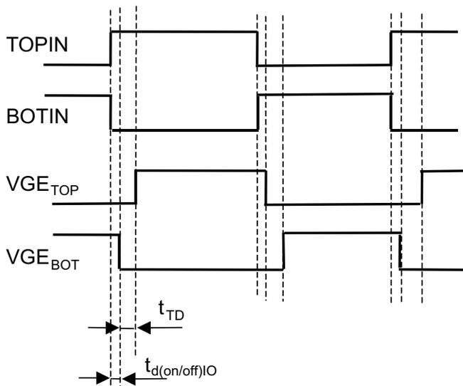
Figure 3.6.12 Delay times of SKiiP control signals
