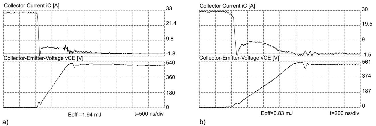
Figure 5.9.11 a) Soft turn-off of a 1200 V / 50 A NPT IGBT at  $C_K = 47$  nF
