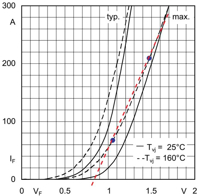
Figure 3.2.9 Forward characteristics (typical and maximum values) of a rectifier diode at two different virtual junction temperatures  $T_{vj}$ ; dotted red line = forward slope resistance used to determine  $V_{(T0)}$  and  $r_f$ ;  $r_f$  results from the line inclination
