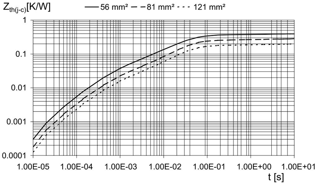
Figure 2.5.22 Time curve of thermal impedances  $Z_{th(j-c)}$  of a module with Al<sub>2</sub>O<sub>3</sub> DBC substrate for different chip areas [37]
