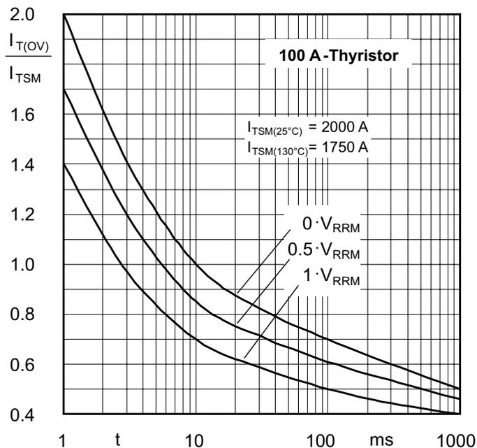
Figure 3.2.14 Permissible overload on-state currents  $I_{T(OV)}$  in relation to surge on-state current  $I_{TSM}$  for a duration of 10 ms for different reverse voltage conditions directly following the last sinusoidal half-wave as a function of time  $t$ .
