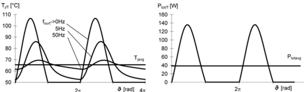
Figure 5.2.13 Simulated junction temperature and power dissipation characteristics of a 1200 V / 50 A-IGBT in inverter mode for different fundamental output frequencies; [37]  $v_d = 540$  V;  $i_{1eff} = 25$  A,  $f_s = 8$  kHz;  $\cos \varphi = 0.8$ ;  $m = 0.8$ ;  $T_h = 50^\circ\text{C}$
