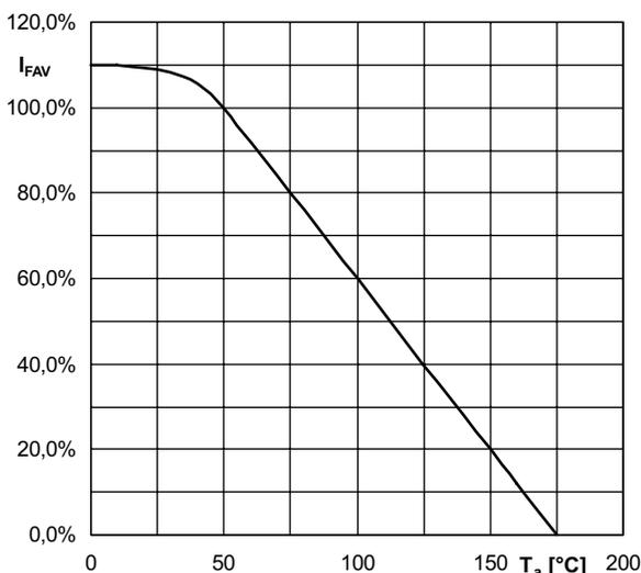
Figure 4.1.1 Permissible mean on-state current  $I_{FAV}$  (as percentage of  $I_{FAV}$  at  $T_a = 50^\circ\text{C}$ ) as a function of the ambient temperature  $T_a$  under the cooling conditions specified in the datasheet.
