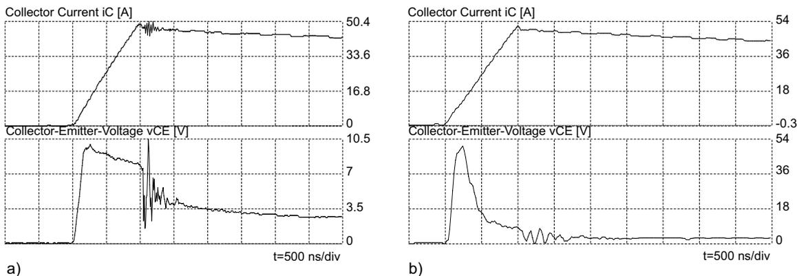
Figure 5.9.9 a)  $di/dt$ -impression in a 1200 V / 50 A-NPT-IGBT ( $di/dt = 50 \text{ A}/\mu\text{s}$ ;  $i_L = 50 \text{ A}$ )
