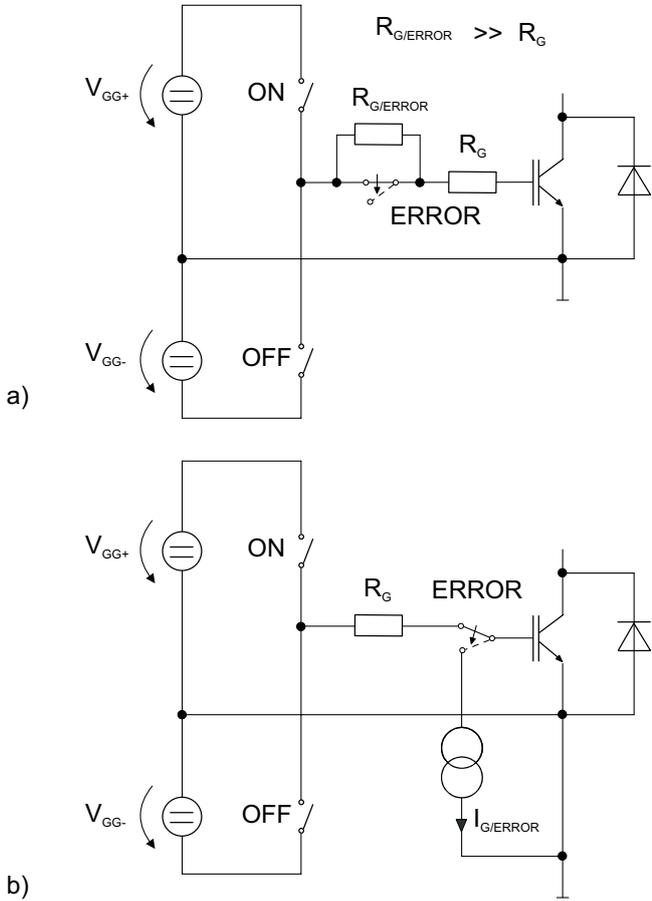
Figure 5.7.18 Possible IGBT soft turn-off processes in the event of malfunction (extremely simplified diagram)
