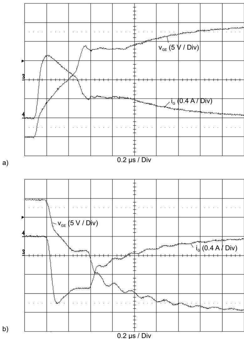
Figure 5.6.2 Gate current and voltage characteristics during turn-on and turn-off
