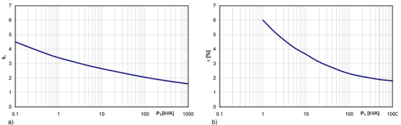
Figure 4.4.8 a) Factor  $k_3$  as a function of the rated power  $P_T$  of the converter transformer; b) Magnetising current  $\varepsilon$  (as a percentage of the rated current) of a converter transformer as a function of its rated power  $P_T$ .
