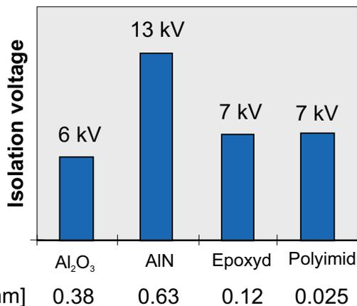
Figure 2.5.12 Insulation voltages for different insulating substrates
