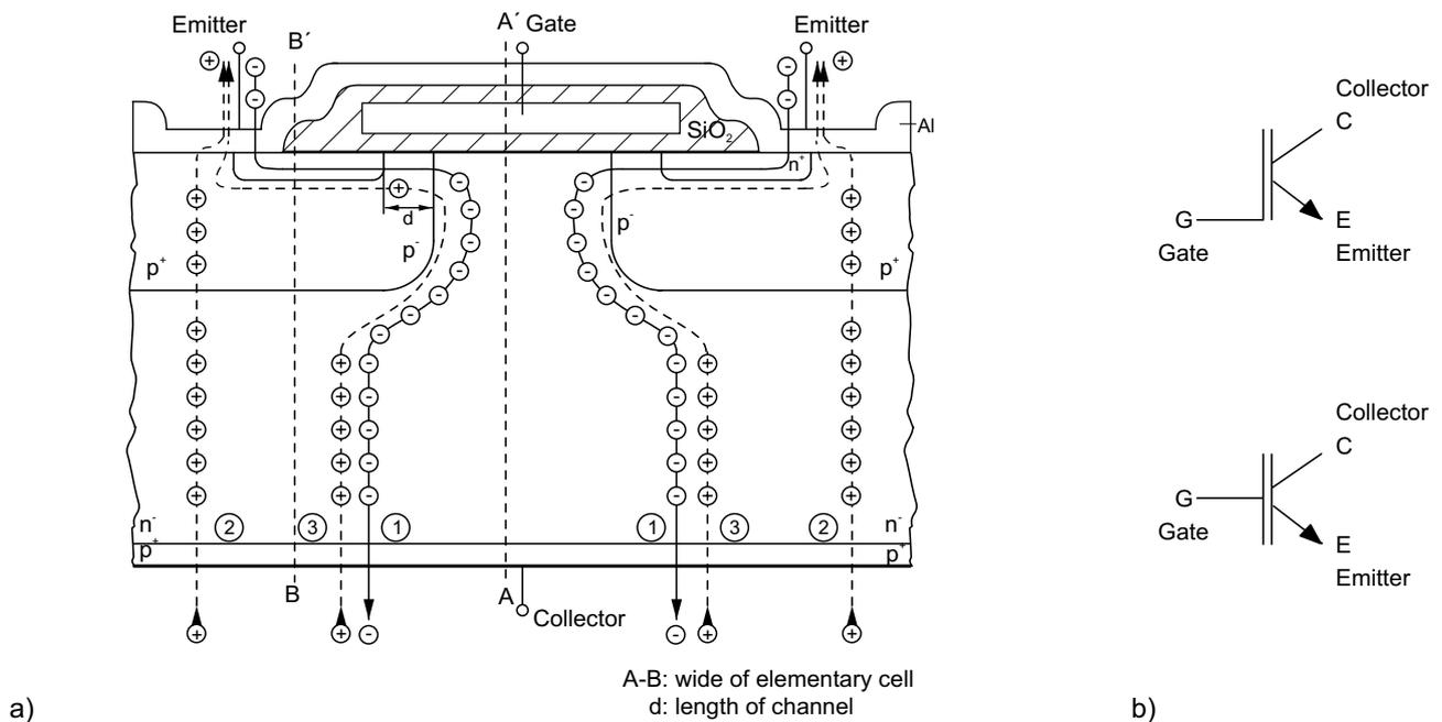
Figure 2.4.3 IGBT with vertical structure and planar gate;
