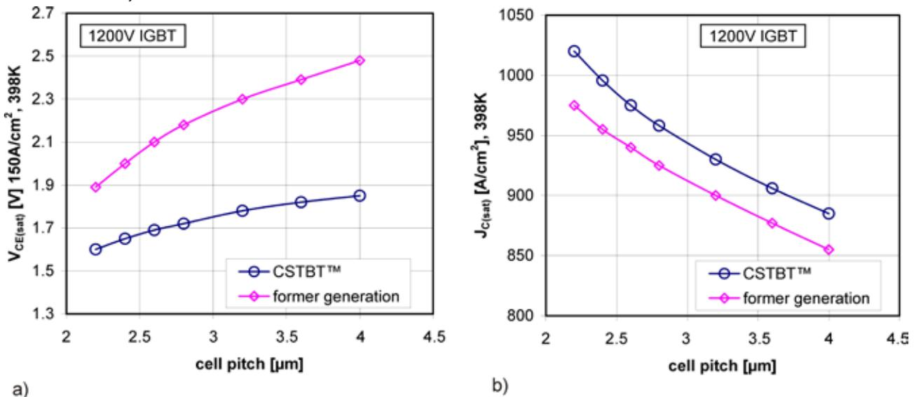
Figure 2.4.8 a) Dependency of the on-state voltage  $V_{CE(sat)}$  of a 1200 V IGBT on the cell pitch for  $T_j = 125^\circ\text{C}$ ; b) Dependency of the collector current density  $J_{C(sat)}$  of a 1200 V IGBT on the cell pitch for  $T_j = 125^\circ\text{C}$  [15]
