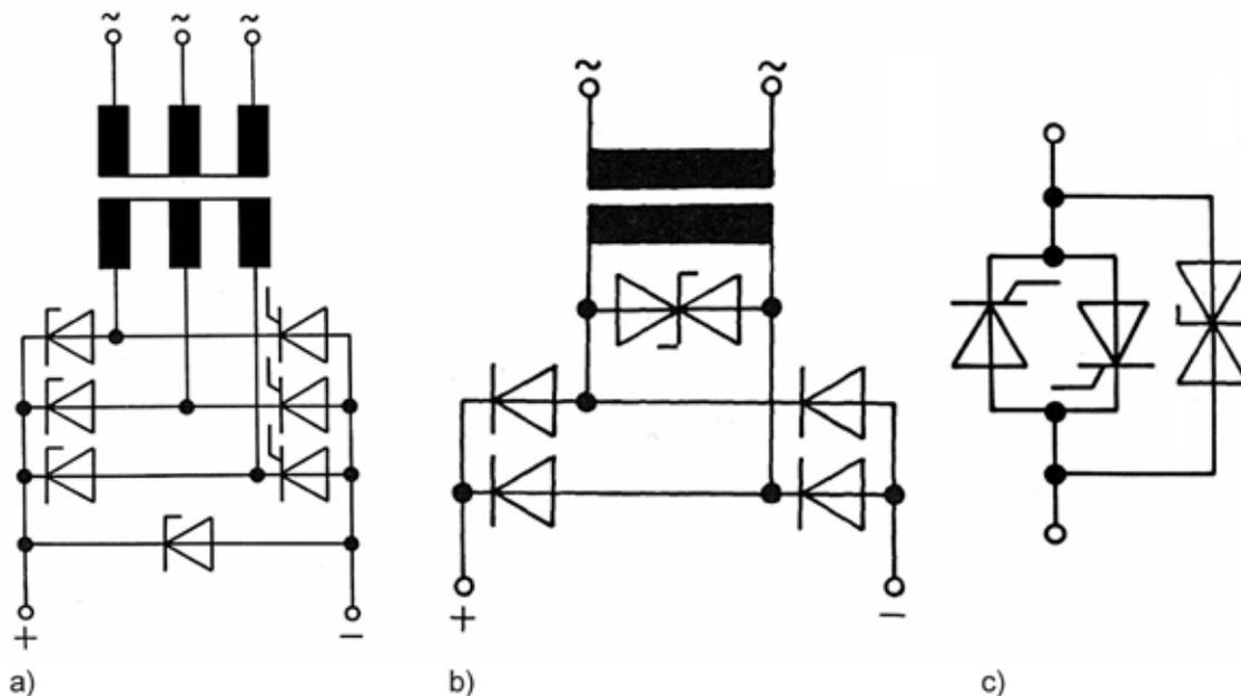
Figure 4.4.13 a) Half-controlled six-pulse bridge circuit with controlled avalanche rectifier diodes that protect the thyristors from overvoltage at the same time; b) AC side protection of a 2-pulse bridge-circuit featuring a bipolar suppressor diode; c) AC voltage controller snubber featuring a bipolar suppressor diode
