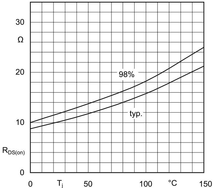
Figure 3.4.8 Typical characteristic of ON-resistance versus chip temperature
