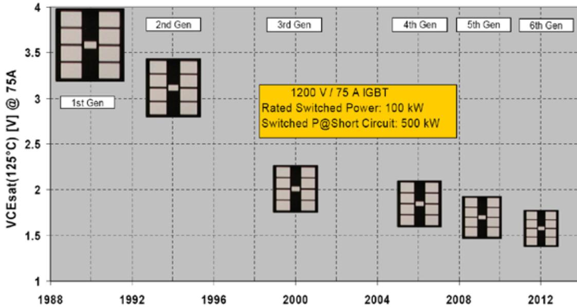
Figure 2.4.9 Development of chip size and on-state voltage of 1200 V / 75 A IGBT chips from Infineon [16]
