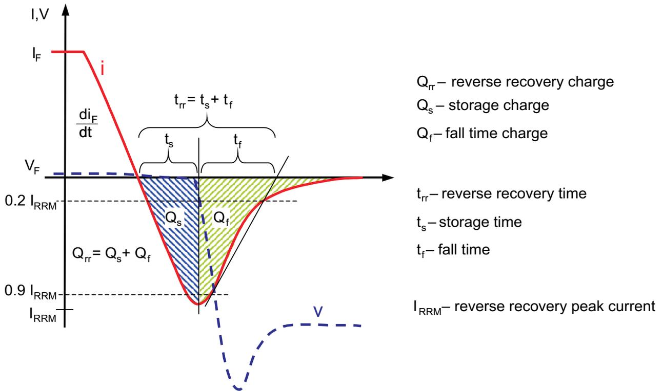
Figure 3.2.11 Current and voltage characteristics of a rectifier diode passing over from conductive to blocking state.
