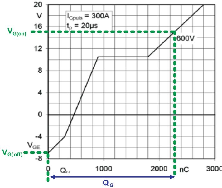
Figure 3.3.6 Gate charge characteristic of an IGBT
