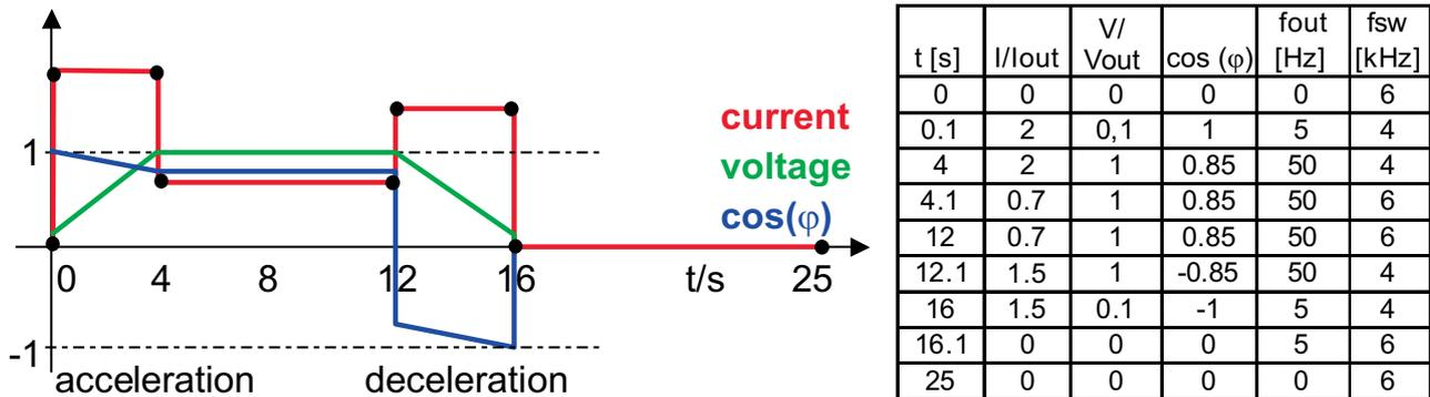
Figure 5.2.18 Definition of a load cycle in SemiSel
