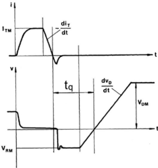
Figure 3.2.23 Main current  $i$  and main voltage  $v$  of a thyristor over time during commutation from on-state to off-state; the circuit commutated turn-off time  $t_q$  is the shorted time interval during which an applied direct off-state voltage will not trigger the thyristor
