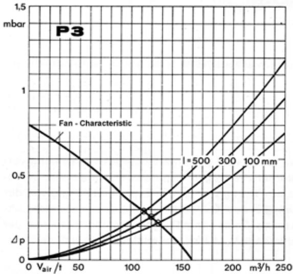
Figure 4.2.10 Diagrams showing pressure drop  $\Delta p$  for different lengths  $l$  of P3 heat sink as a function of air volume  $V_{\text{air}}/t$ , as well as the volume of air moved by the fan as a function of the negative pressure (fan characteristic). The points of intersection constitute the resulting volume of air for the given combination of fan / heat sink profile.
