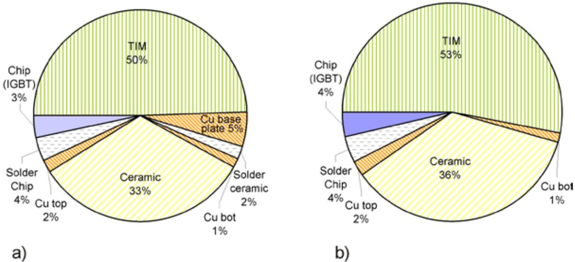
Figure 2.5.16 Influences on the internal thermal resistance of a 1200 V power module, chip surface 9 mm \* 9 mm: a) for DBC substrates ( $Al_2O_3$ ) on Cu base plate, 100  $\mu m$  TIM; b) for DCB substrates ( $Al_2O_3$ ) without Cu base plate, 25  $\mu m$  TIM
