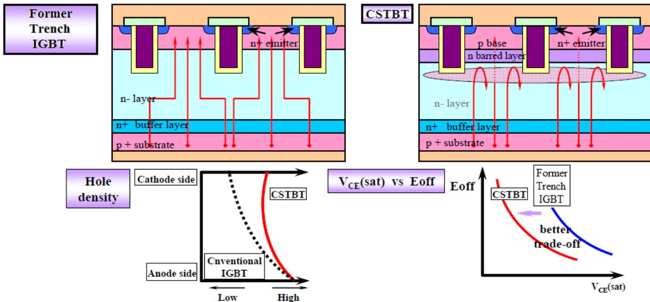
Figure 2.4.13 Basic structure, charge carrier distribution in on-state and trade-off between on-state voltage  $V_{CE(sat)}$  and turn-off losses  $E_{off}$  in conventional Mitsubishi Trench IGBT and CSTBT [21]
