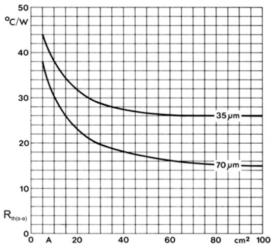
Figure 4.2.3  $R_{th(s-a)}$  of a 1.5 mm thick PCB copper lamination, single-sided lamination, layer thickness 35  $\mu m$  and 70  $\mu m$ , as a function of the area  $A$ . Any mounting position, provided unobstructed airflow across the entire surface is ensured.
