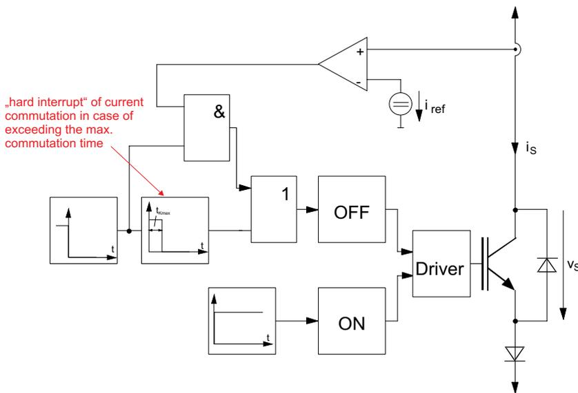
Figure 5.9.8 Modified ZCS: basic principle
