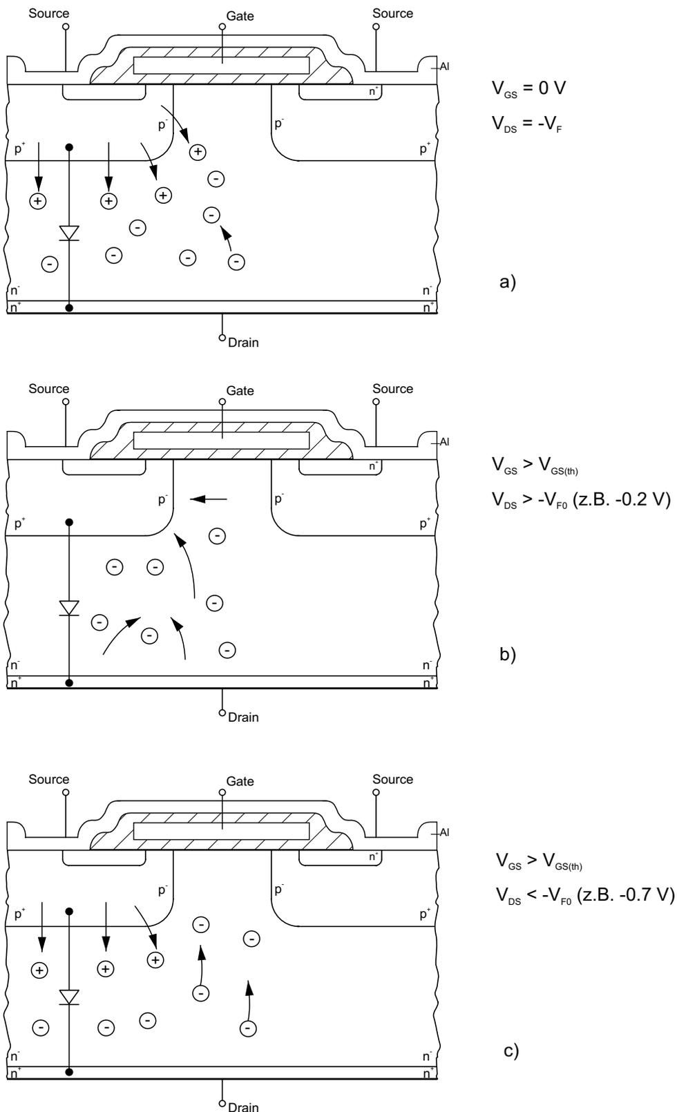
Figure 2.4.18 Inverse operation of a power MOSFET [26] ; a) Closed channel (bipolar current flow); b) Open channel and low negative  $V_{DS}$  (unipolar current flow); c) Open channel and high negative  $V_{DS}$  (combined current flow)
