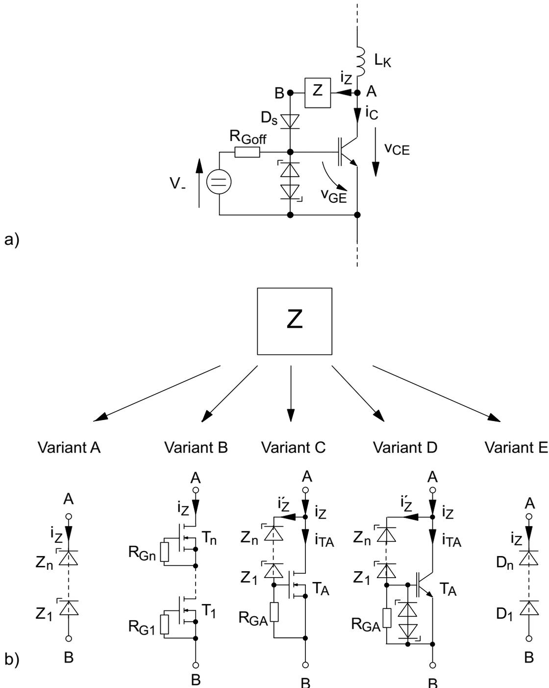
Figure 5.7.15 Basic principle and types of active clamping
