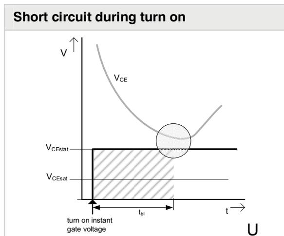
Figure 5.6.11 Possible scenarios for saturation voltage control triggering
