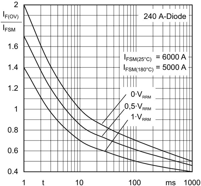
Figure 4.1.4 Permissible error-induced overcurrents  $I_{F(OV)}$  in relation to surge forward current  $I_{FSM}$  for different reverse voltage conditions directly following the last sinusoidal half-wave as a function of time  $t$
