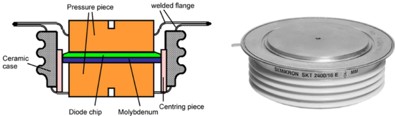
Figure 2.5.32 Sectional view of a disk cell and view of a thyristor disk cell
