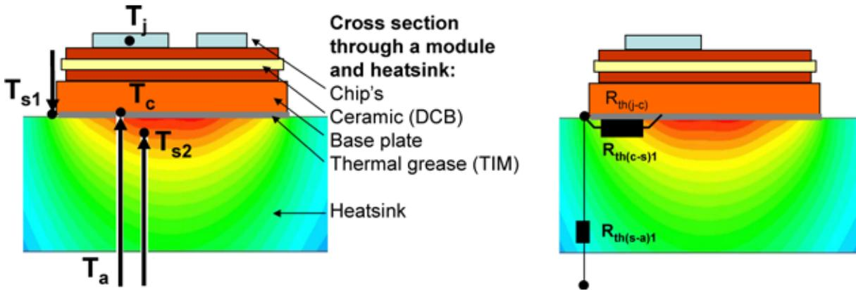
Figure 5.3.5 Measuring points  $T_{s1}$  and  $T_{s2}$  to determine  $R_{th(c-s)}$  and  $R_{th(s-a)}$
