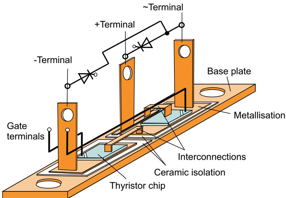
Figure 2.5.35 Schematic layout of a thyristor-halfbridge module
