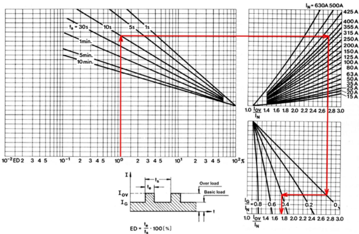
Figure 4.4.18 Alignment chart for the determination of the permissible overcurrent of semiconductor fuses in intermittent operation with and without load
