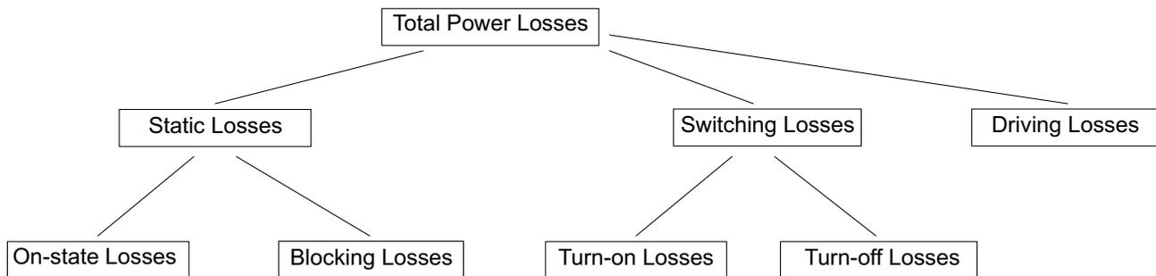
Figure 5.2.1 Individual power losses of power modules used as switches
