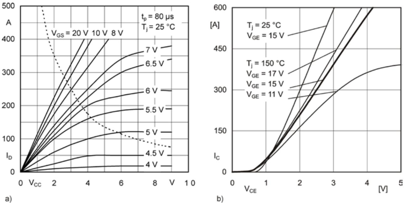
Figure 5.6.4 Forward characteristics versus control voltage  $V_{GG+}$
