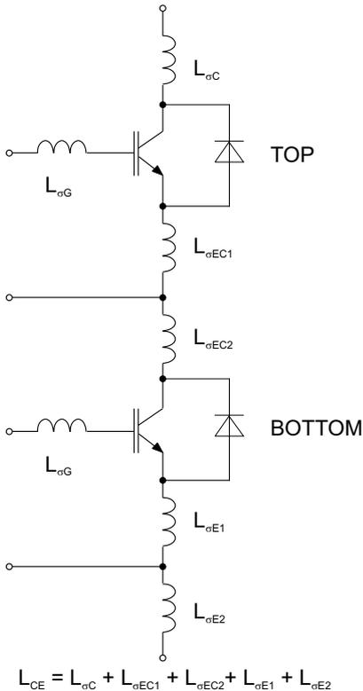
Figure 2.5.24 Parasitic inductances in a dual IGBT module
