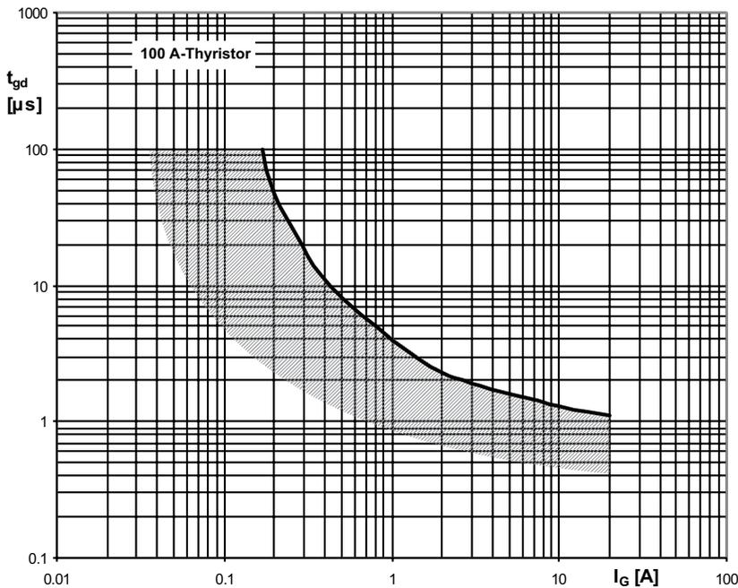
Figure 3.2.19 Typical dependency of a thyristor gate-controlled delay time  $t_{gd}$  on gate current  $I_G$ ; the shaded area represents the variation range.
