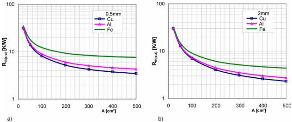
Figure 4.2.1  $R_{th(s-a)}$  for square bare cooling plates made of steel (Fe), aluminium (Al) and copper (Cu) over the area  $A$  for 0.5 mm plate thickness (left) and 2 mm plate thickness (right) for unobstructed airflow across the surface and approx. 40 K temperature difference  $\Delta T_{(s-a)}$
