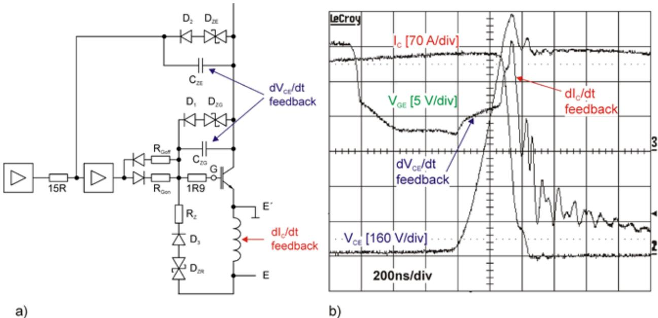
Figure 5.7.20 a) Overvoltage protection by means of combined active clamping and dynamic feedback
