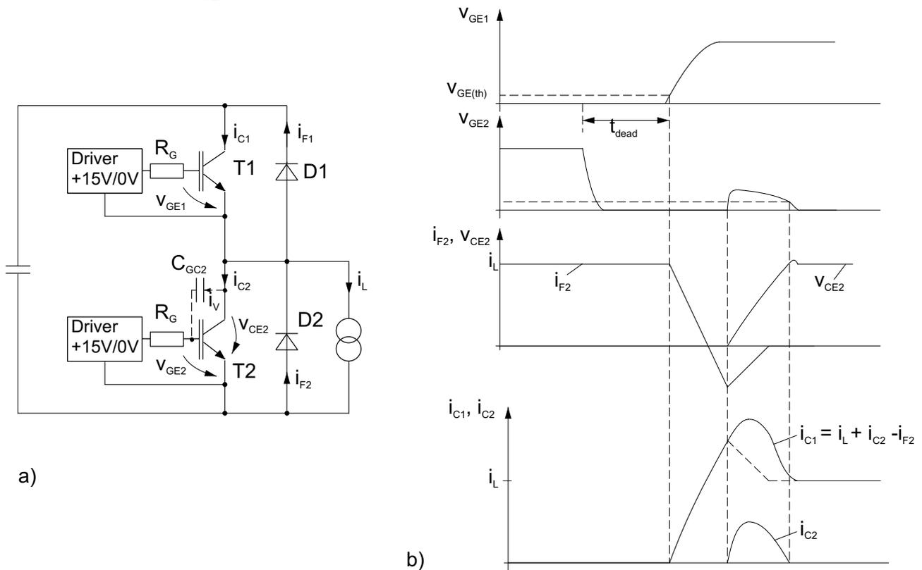
Figure 5.6.3 Cross current in an IGBT bridge arm due to turn-on by  $dv_{CE}/dt$  feedback of T2
