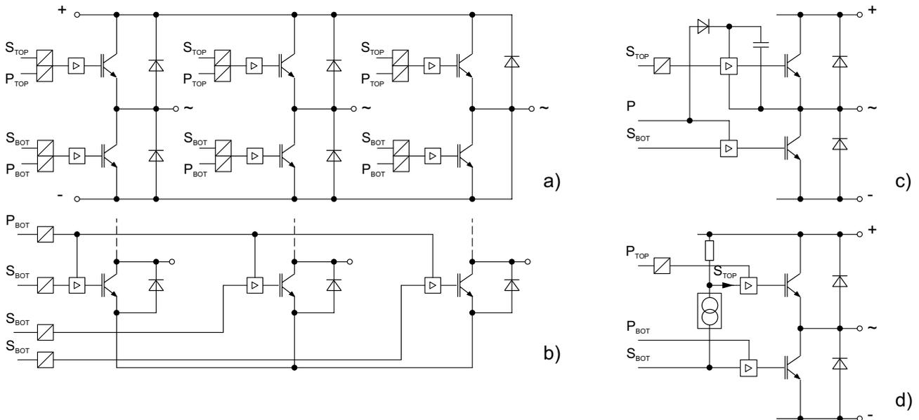
Figure 5.6.12 Selected signal and energy transmission principles
