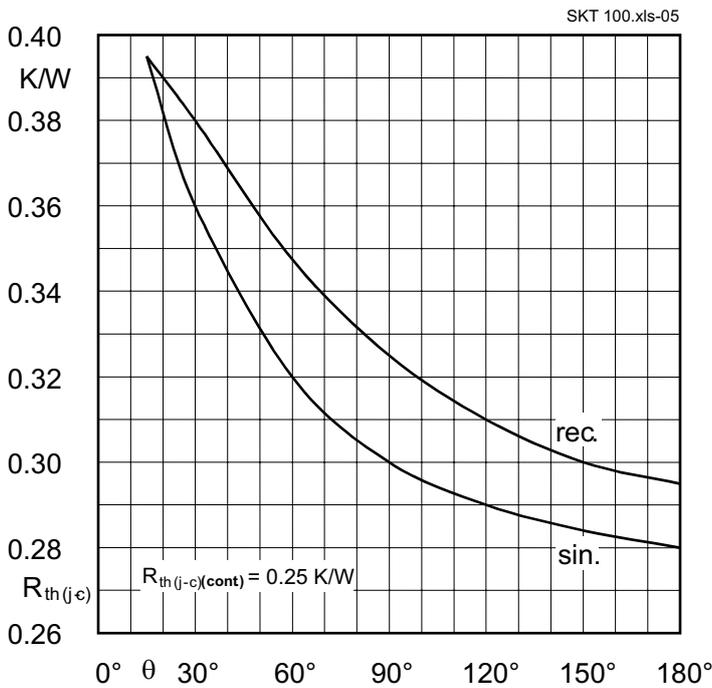
Figure 3.2.3  $R_{th(j-c)}$  of a discrete 100A thyristor multiplied by a corrective factor to calculate the temperature fluctuation as a function of the current conduction angle  $\Theta$  and current waveform
