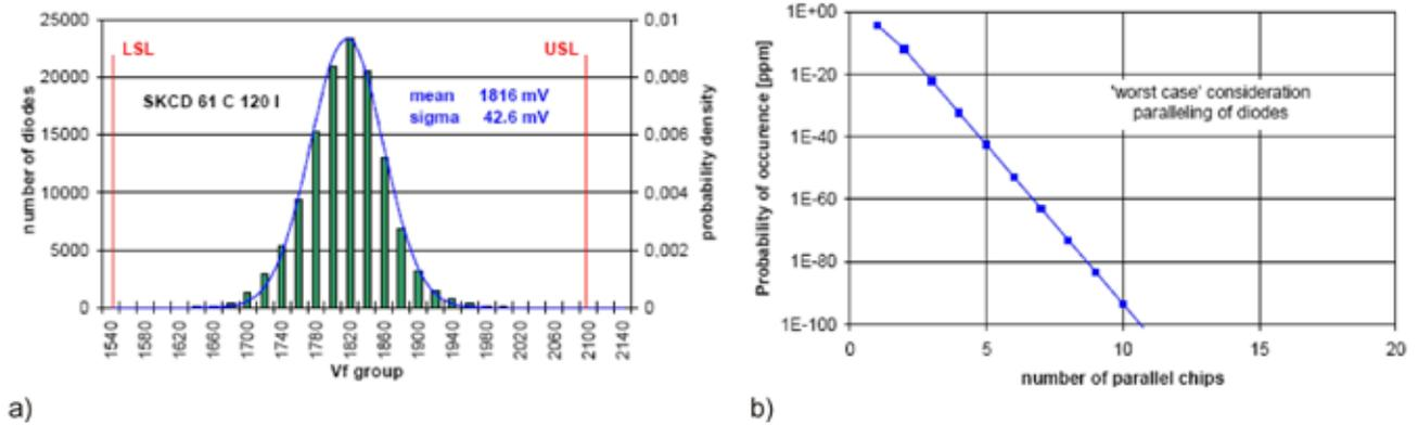
Figure 5.8.3 a) Statistic distribution of diode voltage  $V_f$  @ 50 A for 125,000 diode chips;
