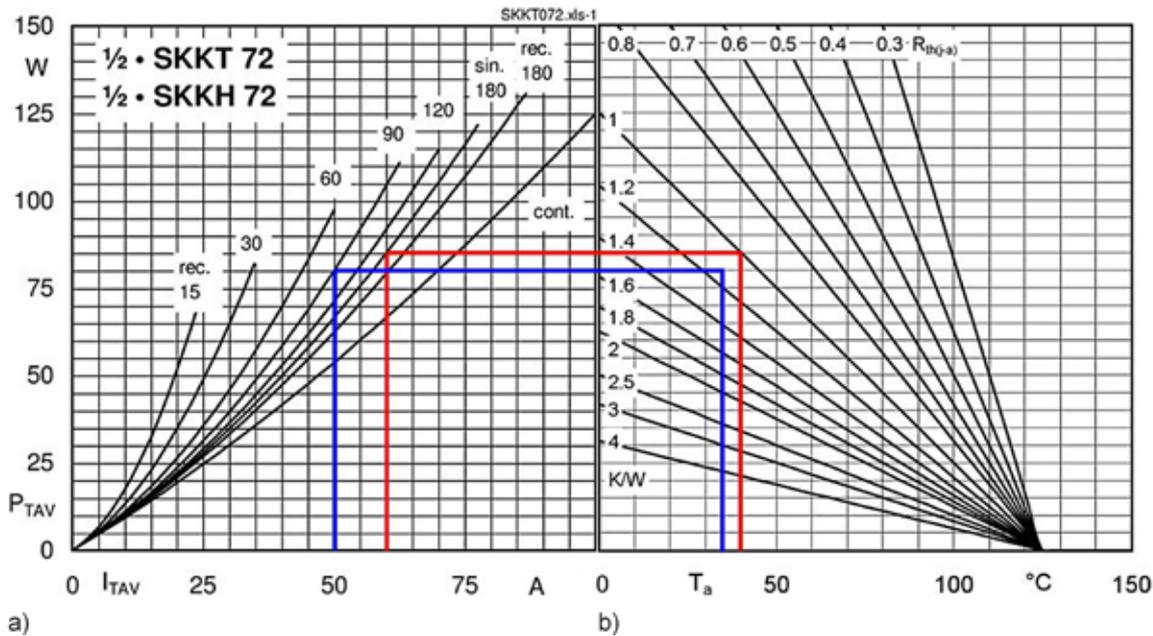
Figure 4.1.10 a)  $P_{TAV}$  as a function of the mean forward current  $I_{TAV}$  for half sine waves (sin. 180), pure DC (cont.) and for rectangular pulses (rec. 15 to 180); b) Permissible power dissipation  $P_{TAV}$  over ambient temperature  $T_a$  for different  $R_{th(j-a)}$ ; all of this data applies to one thyristor alone.
