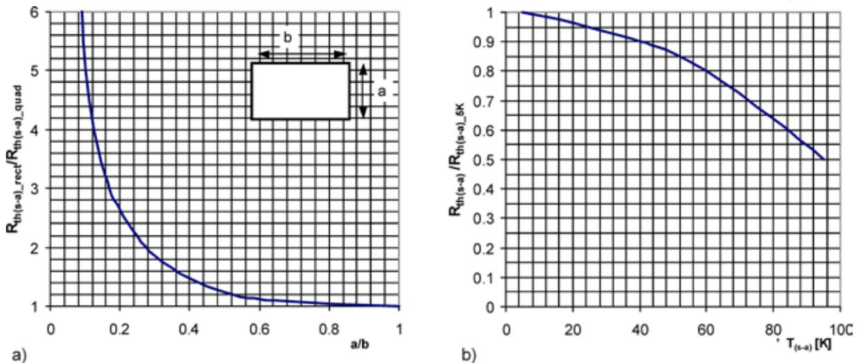
Figure 4.2.2 a) Relative change in  $R_{th(s-a)}$  for non-quadratic cooling plates (r) in dependence of side length ratio  $a/b$ ; b) Relative change in  $R_{th(s-a)}$  of a cooling plate as a function of the temperature difference between cooling plate ( $T_s$ ) and the inflowing air ( $T_a$ ) in relation to a value at  $T_s - T_a = 5$  K
