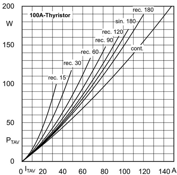
Figure 3.2.16 Mean on-state power dissipation  $P_{TAV}$  as a function of the mean on-state current  $I_{TAV}$  for pure direct current (cont.), 180° half sine waves (sin.180) and rectangular current pulses from 15° to 180° (rec. 15 to 180).
