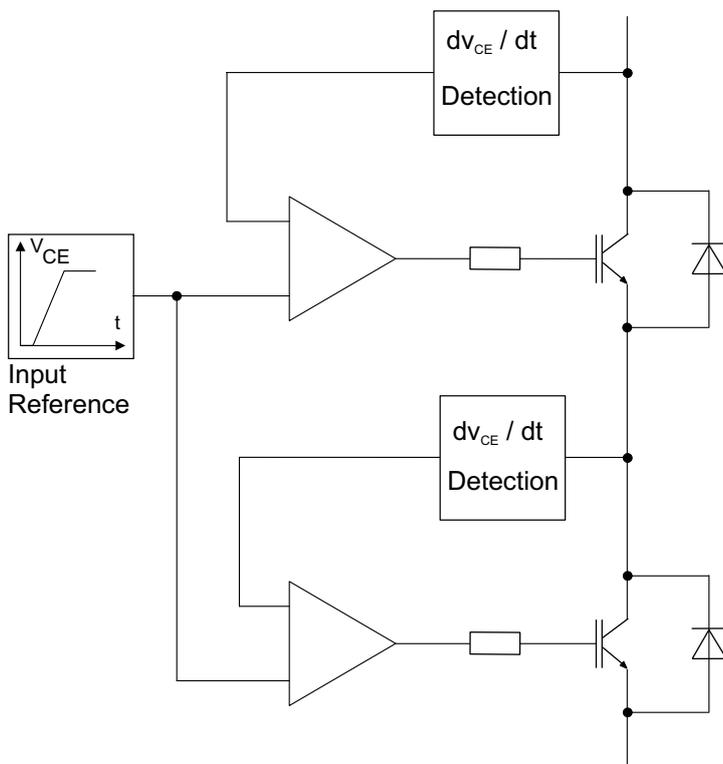
Figure 5.8.21 Dynamic voltage symmetry using  $dv/dt$  control
