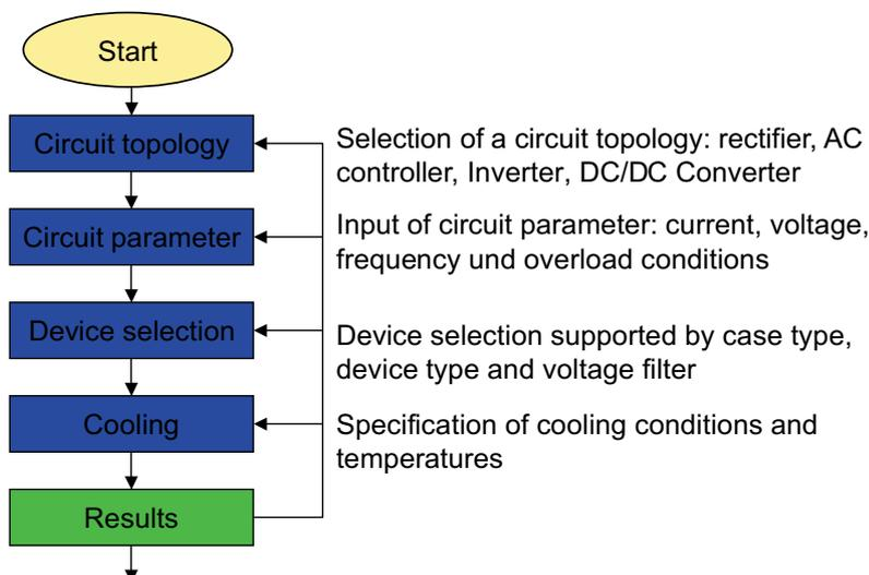
Figure 7.1.1 Program steps in "step by step" dimensioning
