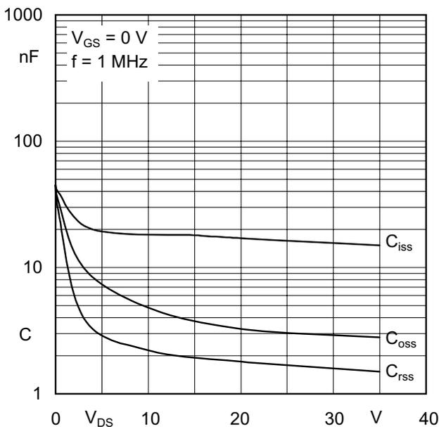
Figure 3.4.12 Typical characteristic of internal capacitances as a function of drain-source voltage
