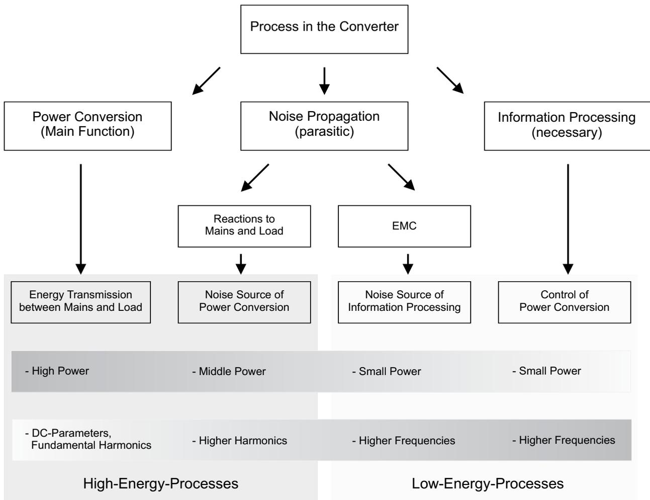
Figure 5.4.2 Energy processes in converters [60]
