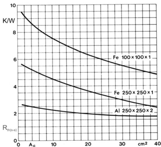
Figure 4.2.4  $R_{th(s-a)}$  of cooling plates with the given dimensions (in mm) made of steel (Fe) and aluminium (Al) as functions of the contact surface area  $A_c$  of the heat generating component for low cooling plate / air temperature difference. The cooling air must be able to flow unobstructed across the entire surface.
