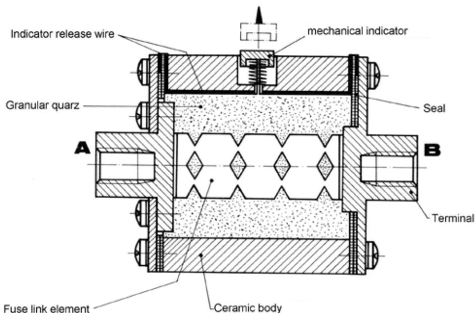
Figure 4.4.16 Cross-section of a semiconductor fuse link
