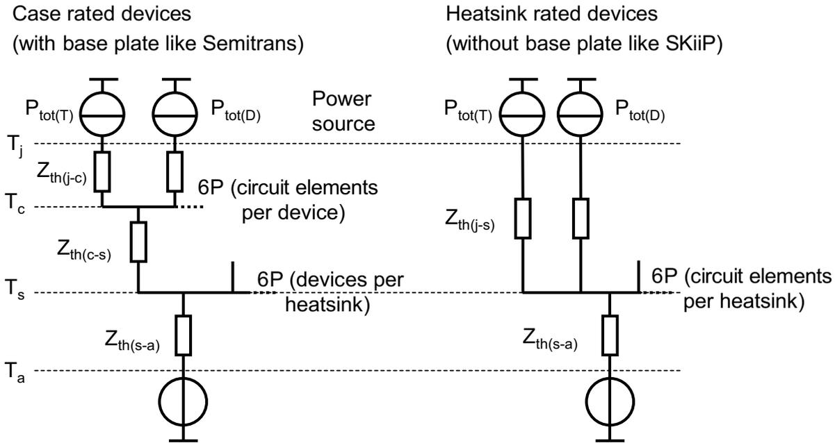
Figure 5.2.5 Simplified thermal equivalent circuit diagram of IGBT and freewheeling diode in a power module: for module with copper base plate (l); for module without base plate (r).
