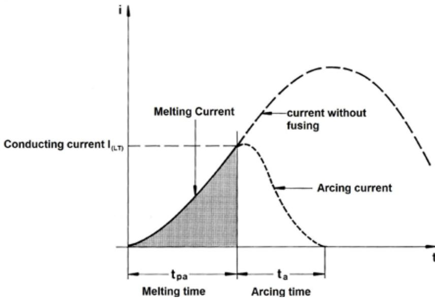
Figure 4.4.17 Current characteristic for short-circuit "turn-off" by a semiconductor fuse with current clamping (let-through current smaller than the peak prospective current); Pre-arc time + arcing time = operating time
