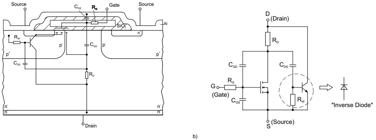
Figure 2.4.16 Power MOSFET cell including the key parasitic elements
