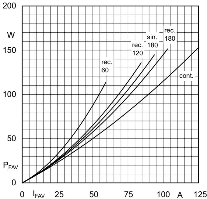
Figure 3.2.10 Mean forward power dissipation  $P_{FAV}$  over mean forward current  $I_{FAV}$  of a 70 A diode for pure direct current (cont.), half sine waves 180° (sin. 180) and rectangular current pulses 60° (rec. 60) to 180° (rec. 180)
