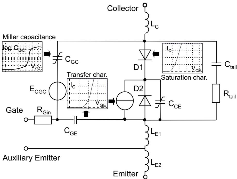
Figure 7.2.4 Example of an IGBT behaviour model with equivalent circuit elements [84]
