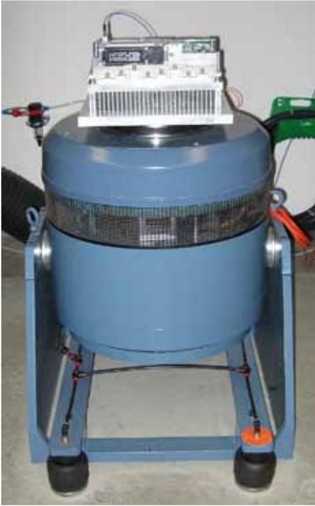
Figure 2.7.4 SKiiP system on a vibrating plate
