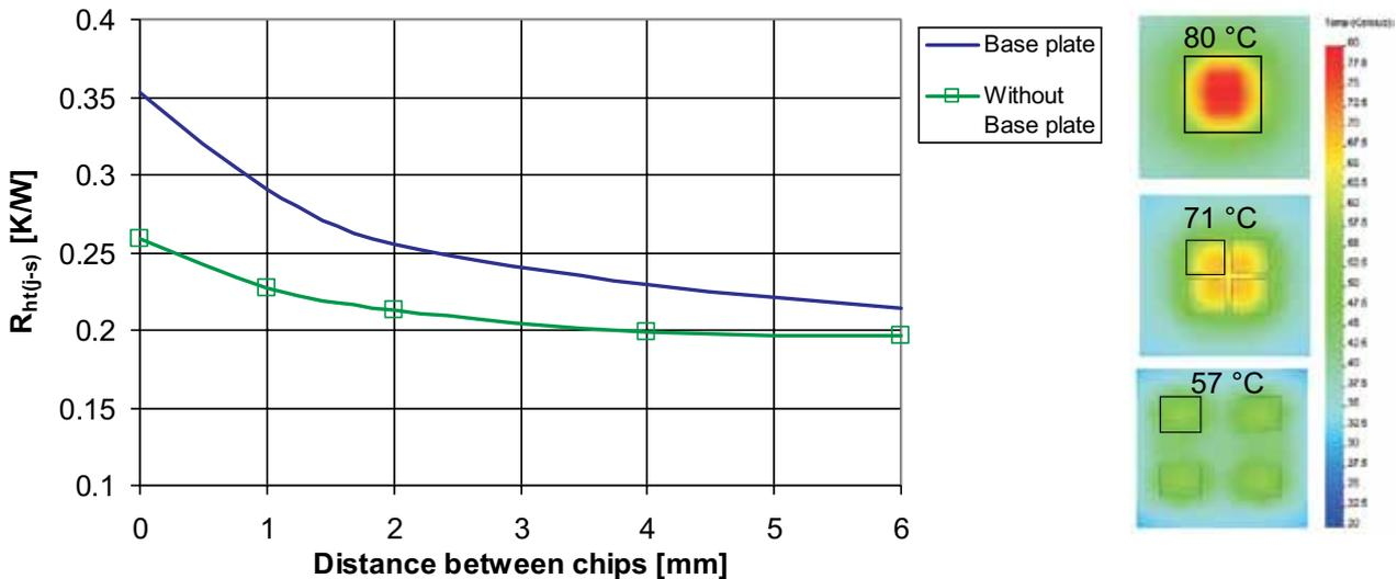
Figure 2.5.21 Thermal resistance  $R_{\text{th}(j-s)}$  of four  $36 \text{ mm}^2$  chips as a function of the chip distance; (thermal paste thickness: with base plate  $100 \mu\text{m}$ , without  $25 \mu\text{m}$ ), right: simulation of chip temperatures assuming same power loss and chip area but increasing distance (0 mm, 1 mm, 6 mm)
