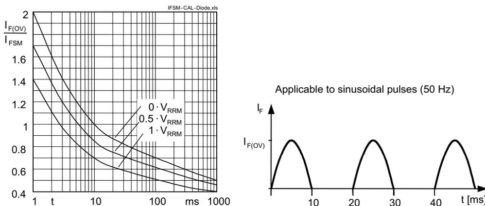
Figure 3.3.3 Surge forward current characteristics: Overload forward currents  $I_{F(OV)}$  permissible in the event of a malfunction as a function of time related to surge forward current  $I_{FSM}$  at 10 ms under different reverse voltage conditions directly after the last half sine wave.
