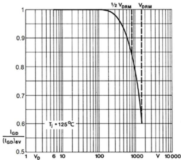
Figure 3.2.22 Gate non-trigger current  $I_{GD}$  at  $V_D = 6\text{ V}$  as a function of off-state voltage  $V_D$ ; typical characteristic for a thyristor with a max. repetitive peak off-state voltage  $V_{DRM} = 1600\text{ V}$
