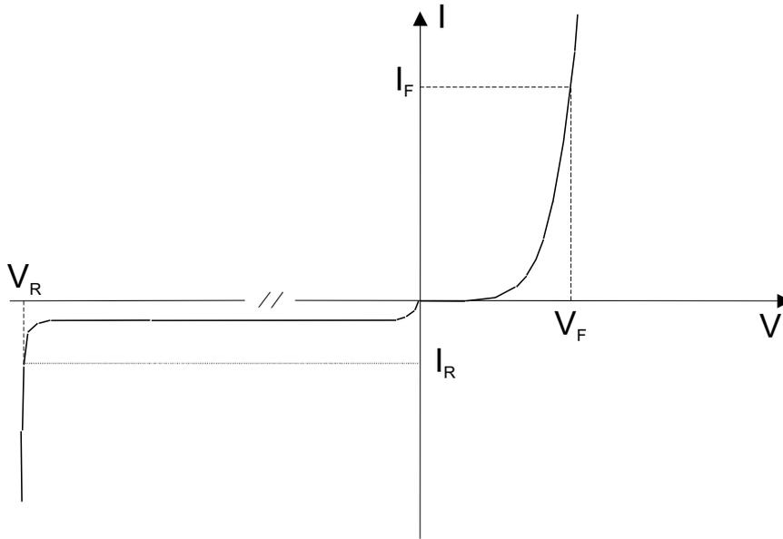
Figure 2.3.5 Definition of reverse and forward diode voltage
