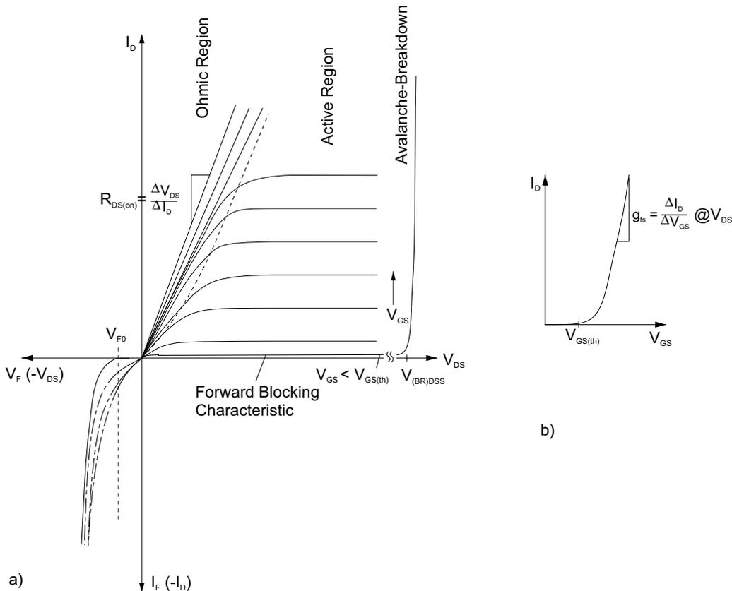
Figure 2.4.17 a) Output characteristics of a power MOSFET (n-channel enhancement type)
