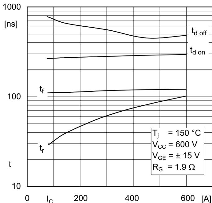
Figure 3.3.21 IGBT switching times versus collector current
