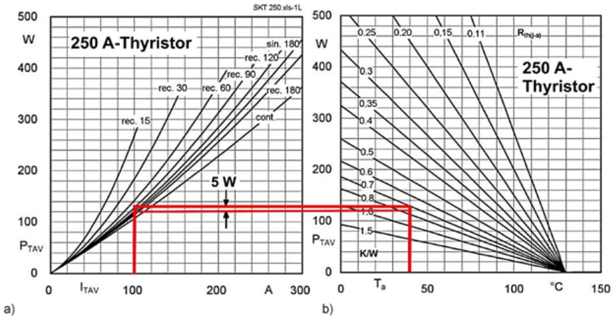
Figure 4.1.5 a) Mean forward dissipation  $P_{TAV}$  over mean forward current  $I_{TAV}$  for different conduction angles; b) Permissible power dissipation  $P_{TAV}$  over ambient temperature  $T_a$  and different  $R_{th(j-a)}$ .
