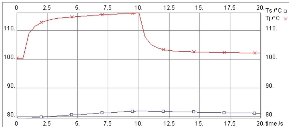
Temperature characteristic overload current
