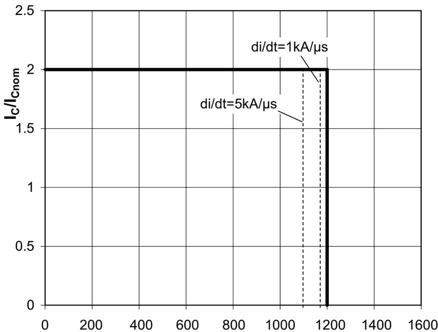
Figure 3.3.28 Turn-off safe operating area (RBSOA) of a 1200 V IGBT;  $T_j < T_{j(max)}$ ;  $V_{GE} = \pm 15$  V;  $R_G = R_{G(nom)}$
