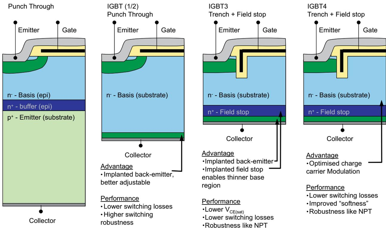
Figure 2.4.10 IGBT concepts, basic properties and off-state field intensity characteristics (acc. to [18])
