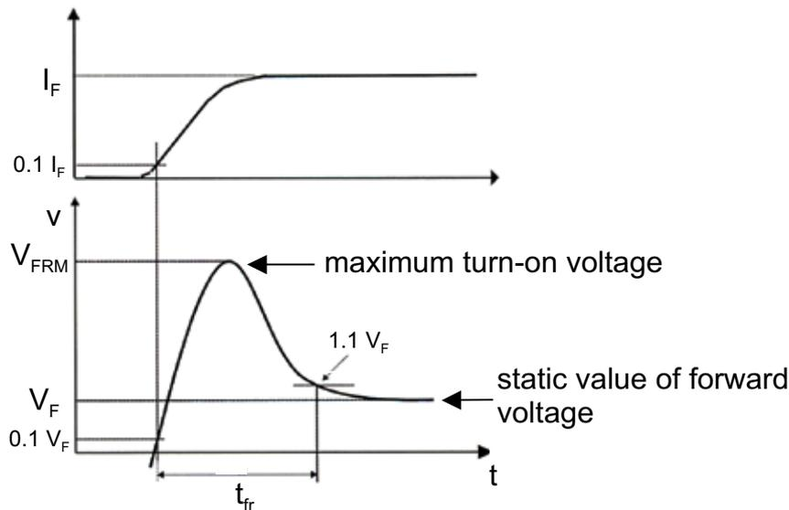
Figure 2.2.4 Diode turn-on behaviour
