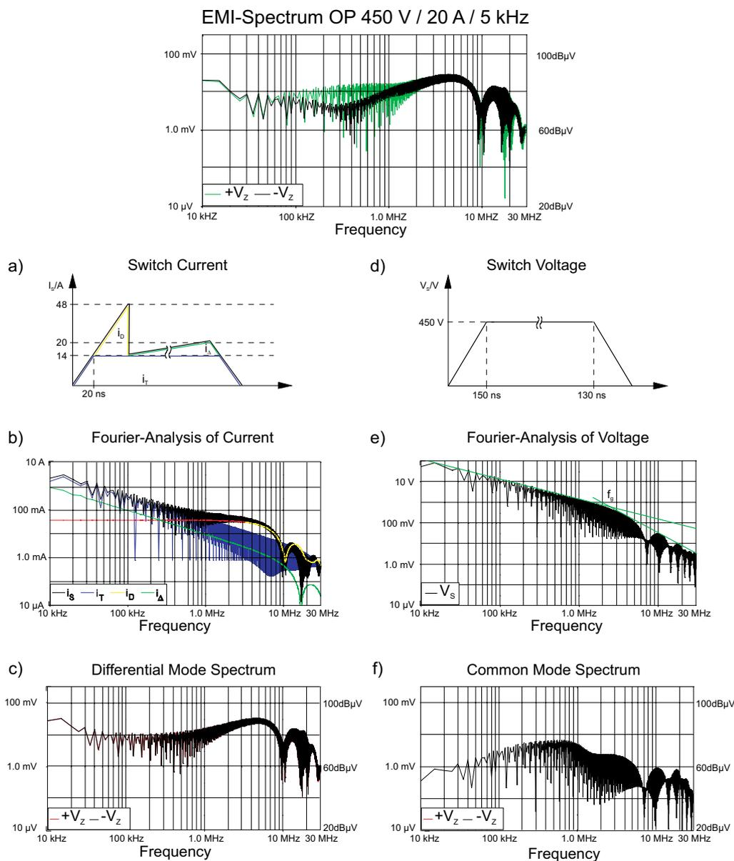
Figure 5.4.6 Simulation results for a 1200 V / 50 A NPT IGBT dual module
