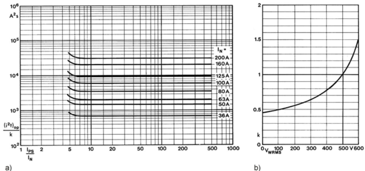
Figure 4.4.19 a) Operating  $i^2t$  values  $(i^2t)_{op}$  divided by the factor  $k$ , as a function of the prospective short-circuit current  $I_{PS}$ , in relation to the fuse rated current  $I_N$  for semiconductor fuses of 35 A - 200 A; b) Factor  $k$  as a function of the recovery voltage  $V_{WRMS}$
