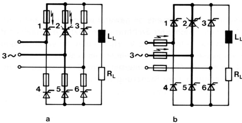
Figure 4.4.22 Switching voltages across the tripped fuses in the case of a short circuit induced by failure of thyristor 2 to block
