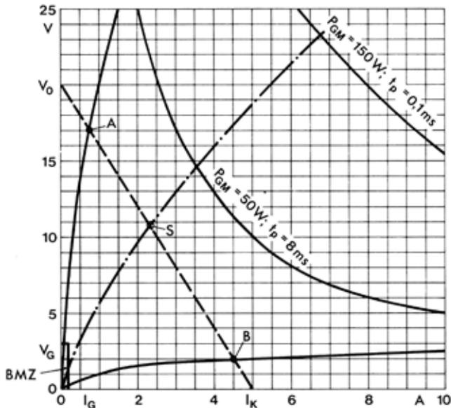
Figure 4.3.2 Gate current ( $I_G$ ) – gate voltage ( $V_G$ ) characteristic of a thyristor in linear scheme; dotted output characteristic,  $V_0$  – no-load voltage and  $I_K$  – short-circuit current of the driver device; dash-dotted output characteristic of the control terminal – cathode of a typical thyristor
