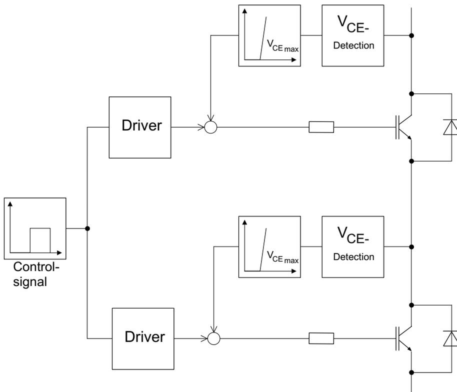
Figure 5.8.22 Active voltage limitation / active clamping
