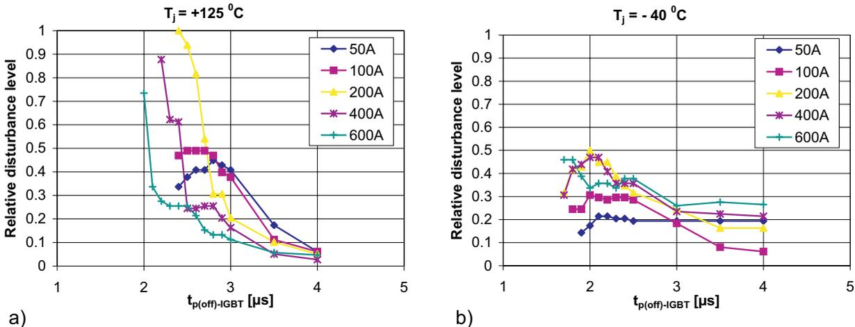
Figure 2.3.14 Relative interference level related to the maximum value at 200 A and 125°C for IGBT turn-off signals of different durations as a function of current and temperature (a)  $T_j=125^\circ\text{C}$ , b)  $T_j=-40^\circ\text{C}$ )
