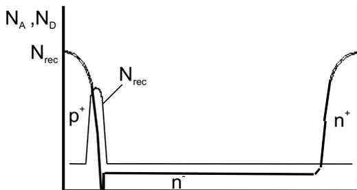
Figure 2.3.2 Narrow region with a high concentration of recombination centres at the pn-junction, generated by light ion irradiation
