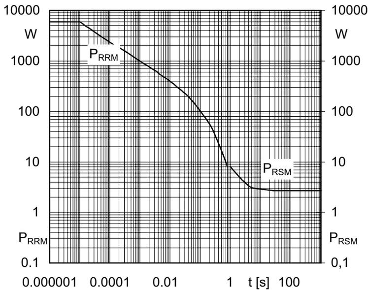
Figure 3.2.8 Non-repetitive peak reverse power dissipation  $P_{RSM}$  ( $t < 1$  s, forward current load  $0.8 \cdot I_{FAV}$ ) and peak repetitive reverse power dissipation  $P_{RRM}$  ( $t > 1$  s, no forward current load) of a 20 A avalanche rectifier diode as a function of time  $t$ .
