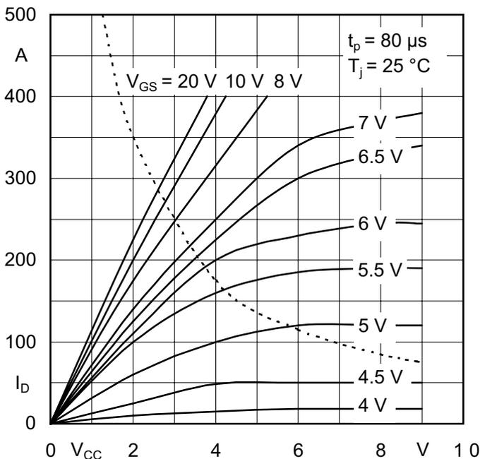
Figure 3.4.6 Typical forward characteristics  $I_D = f(V_{DS})$
