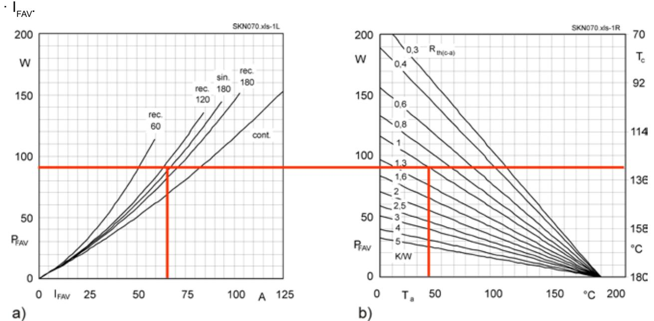
Figure 3.2.12 a) Mean forward power dissipation  $P_{FAV}$  over mean forward current  $I_{FAV}$  for different current waveforms; b) Case temperature  $T_c$  over ambient temperature  $T_a$ ; the parameter is the thermal resistance case-to-air  $R_{th(c-a)}$  of a 70 A diode
