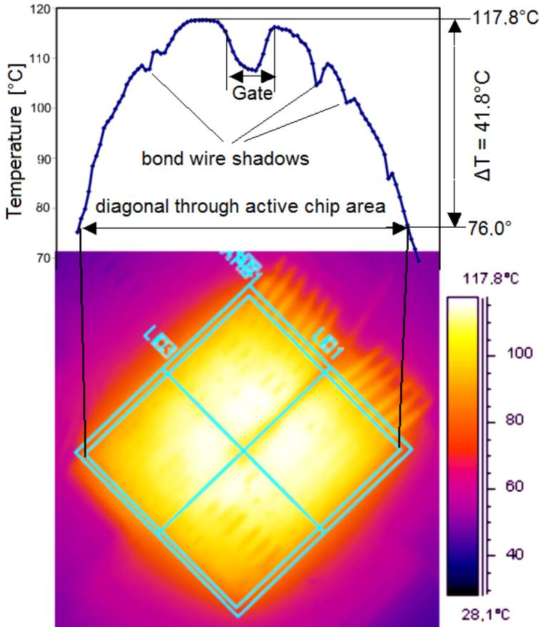
Figure 3.2.1 The bottom part of the illustration shows the infrared image of a live, bonded chip with an active area of  $12 \times 12 \text{ mm}^2$ ; the scale on the right represents the assignment of temperatures to pseudo colours. The upper part of the illustration shows the evaluation of the infrared image in reference to the temperature measured across the chip
