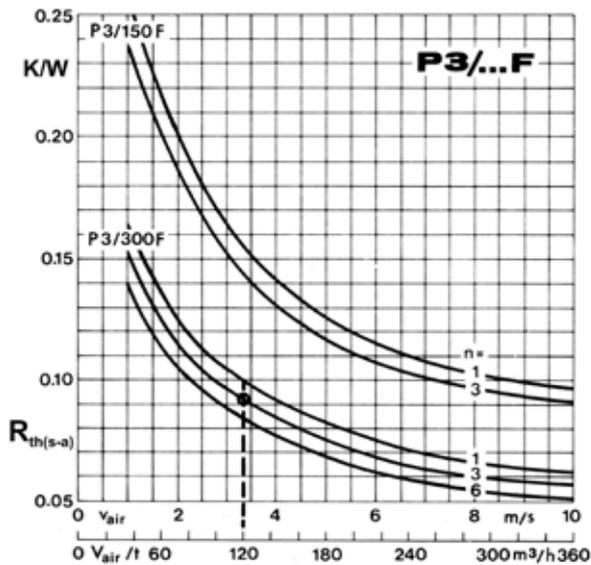
Figure 4.2.11  $R_{\text{th}(s-a)}$  for P3 heat sink profile in different lengths, equipped with  $n = 1 - 6$  components, as a function of the air volume  $V_{\text{air}}/t$  or air velocity  $v_{\text{air}}$
