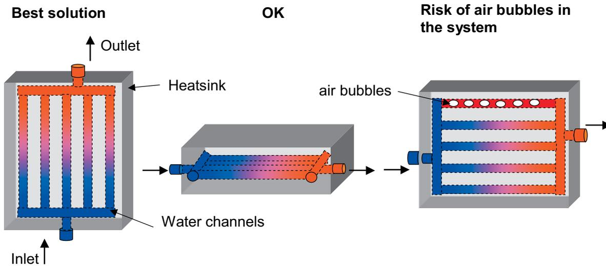
Figure 5.3.18 Tips on how to arrange water coolers
