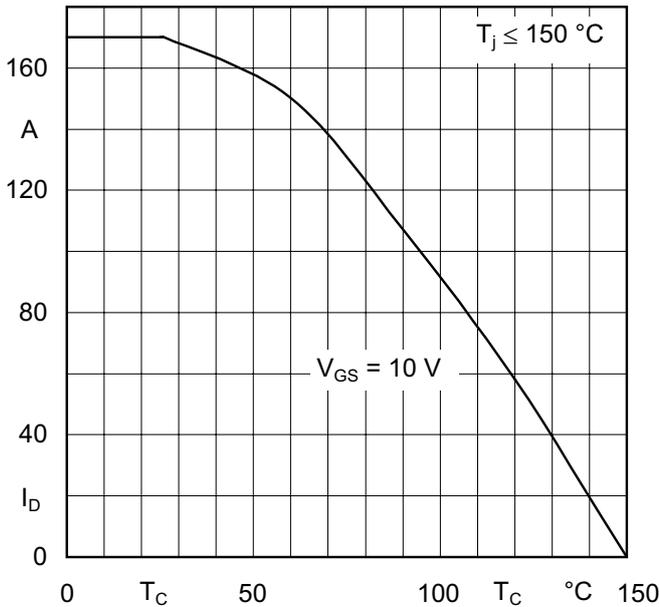
Figure 3.4.9 Drain current derating versus case temperature
