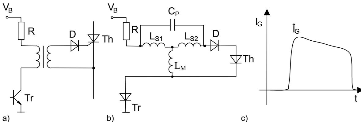
Figure 4.3.1 a) Drive circuit, b) Equivalent circuit; c) Time characteristic of drive signal
