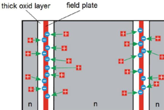
Figure 2.4.23 Principle layout of an OptiMOS [29]
