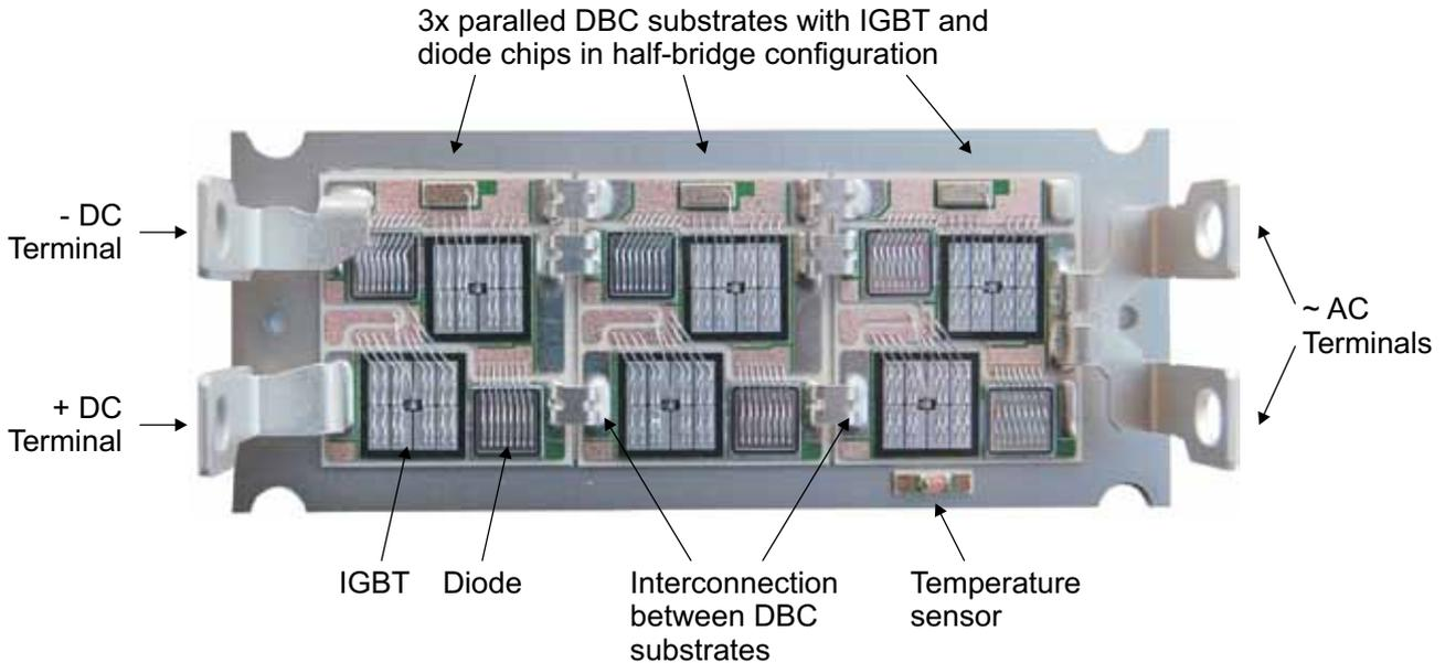
Figure 2.5.45 Internal structure of a SEMiX3 module
