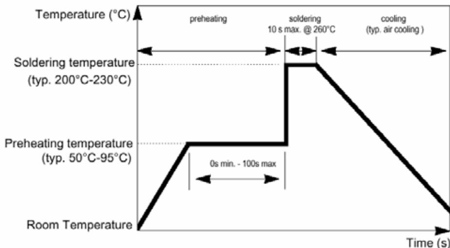
Figure 6.3.9 Wave soldering profile for SEMIKRON power modules
