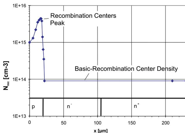
Figure 2.3.3 Recombination centre profile in the CAL diode (diagram)
