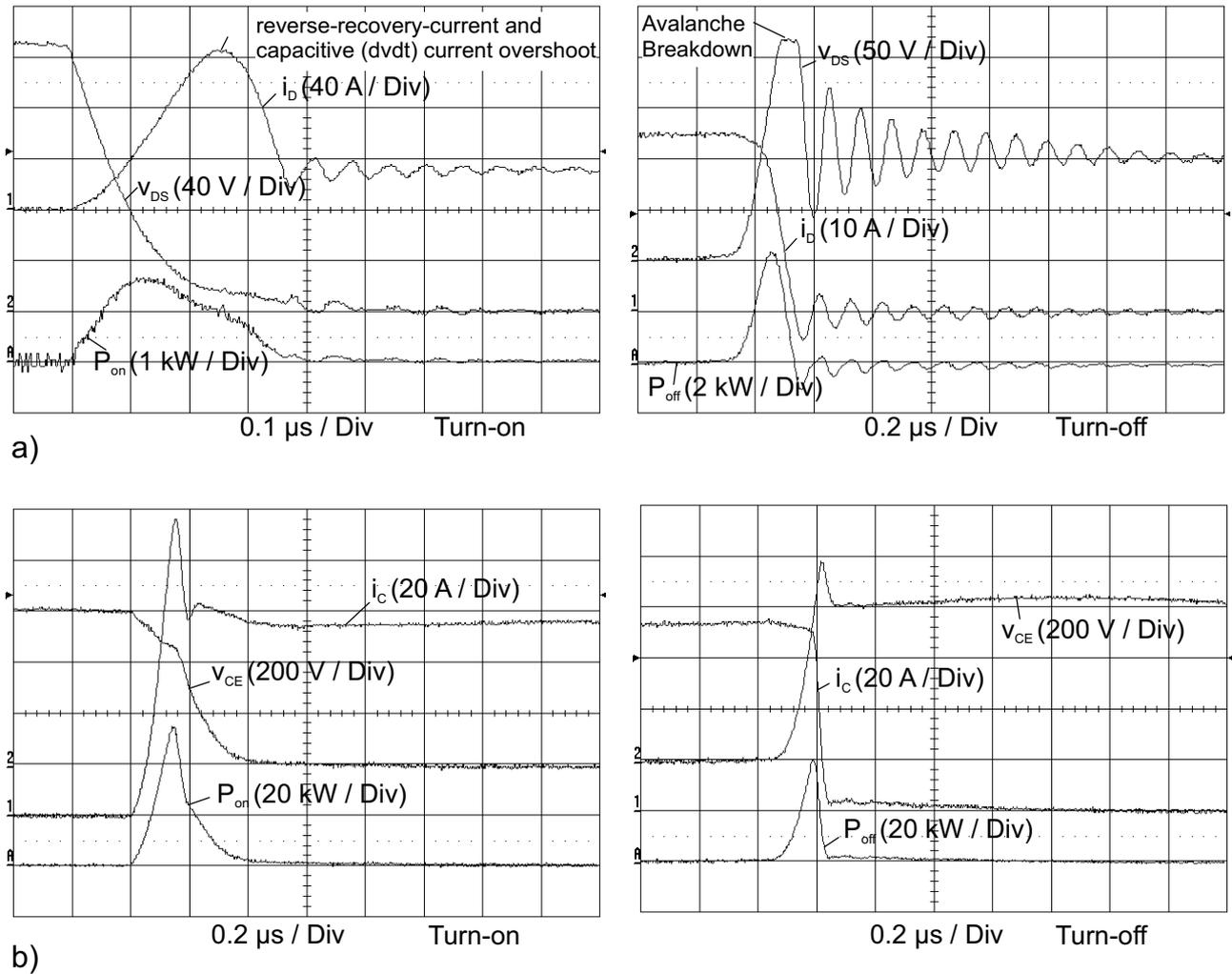
Figure 5.1.8 Measured switching processes (hard turn-on and turn-off under ohmic-inductive load)
