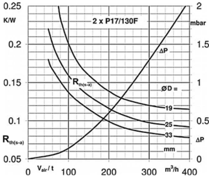
Figure 4.2.9  $R_{th(s-a)}$  of P17 heat sink of 130 mm in length for disc cells with double-sided cooling and pressure drop  $\Delta P$  between air entry and exit as a function of the air volume in the given time  $V_{air}/t$ .  $\varnothing D$  is the diameter of the contact element of the disc cell.
