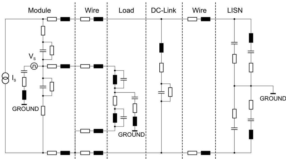
Figure 5.4.4 EMI equivalent circuit of a step-down converter [38]
