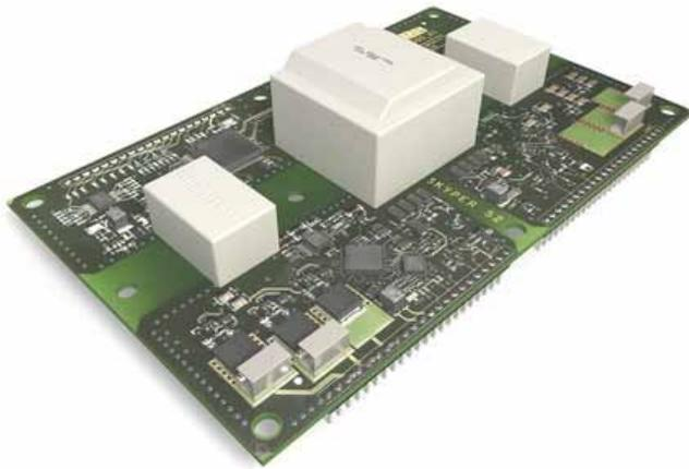
Figure 5.6.16 SKYPER 52 R driver stage PCB
