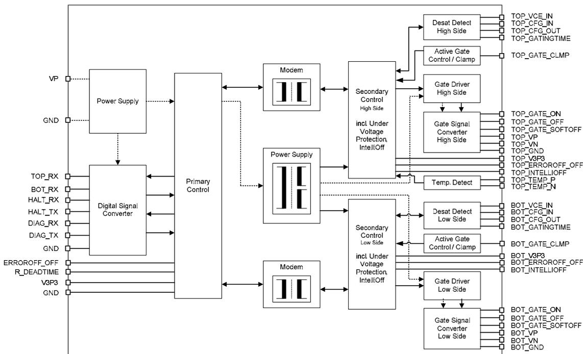
Figure 5.6.17 SKYPER 52 R driver stage block diagram
