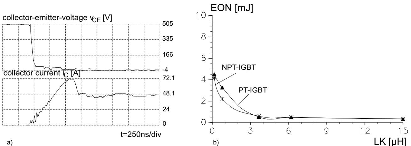
Figure 5.9.14 a) Low-loss turn-on of an NPT IGBT ( $L_K = 3.6 \mu\text{H}$ )
