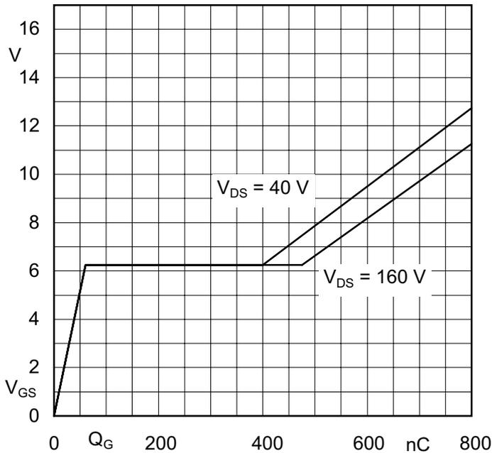
Figure 3.4.13 Typical gate charge characteristic  $V_{GS} = f(Q_G)$
