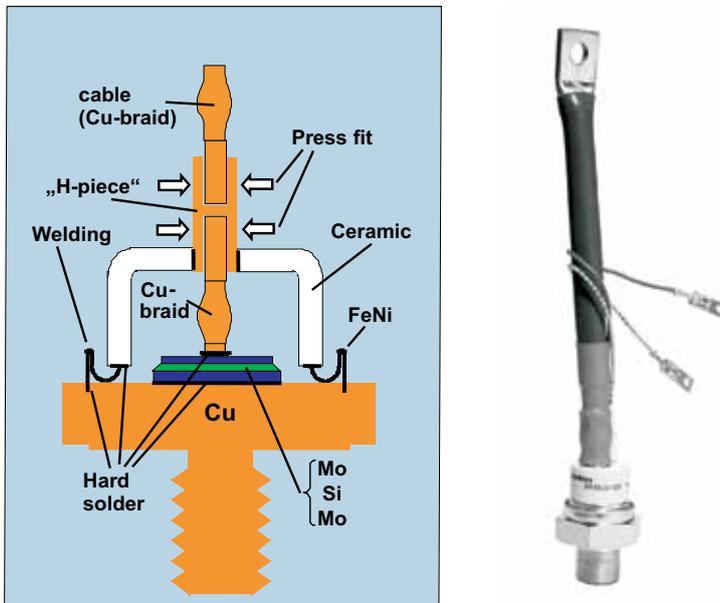
Figure 2.5.31 Sectional view of a stud-mounted diode and example of a stud thyristor
