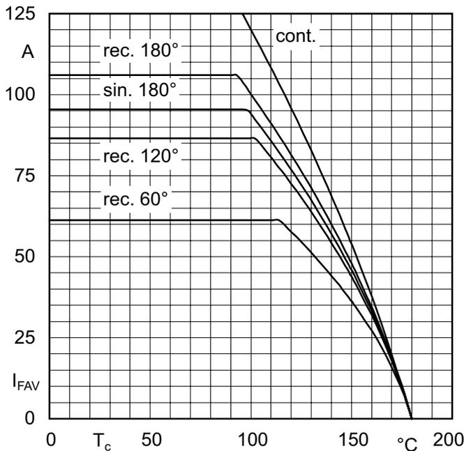
Figure 3.2.6 Mean forward current  $I_{FAV}$  of a 70 A rectifier diode as a function of the case temperature  $T_c$ . 180, rectangular pulses 180°, 120°, 60°: rec. 180, rec. 120, rec. 60)
