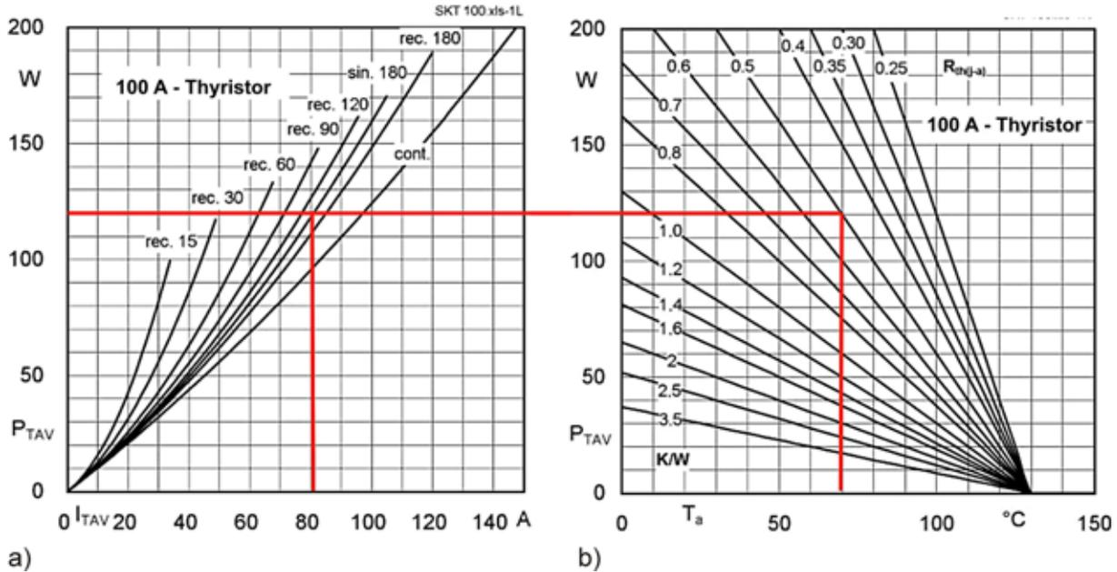
Figure 3.2.27 a) Mean on-state power dissipation  $P_{TAV}$  over mean on-state current  $I_{TAV}$  for different current waveforms; b) Permissible ambient temperature  $T_a$  over thermal resistance junction-to-ambient  $R_{th(j-a)}$  including the contact thermal resistance case-to-heatsink
