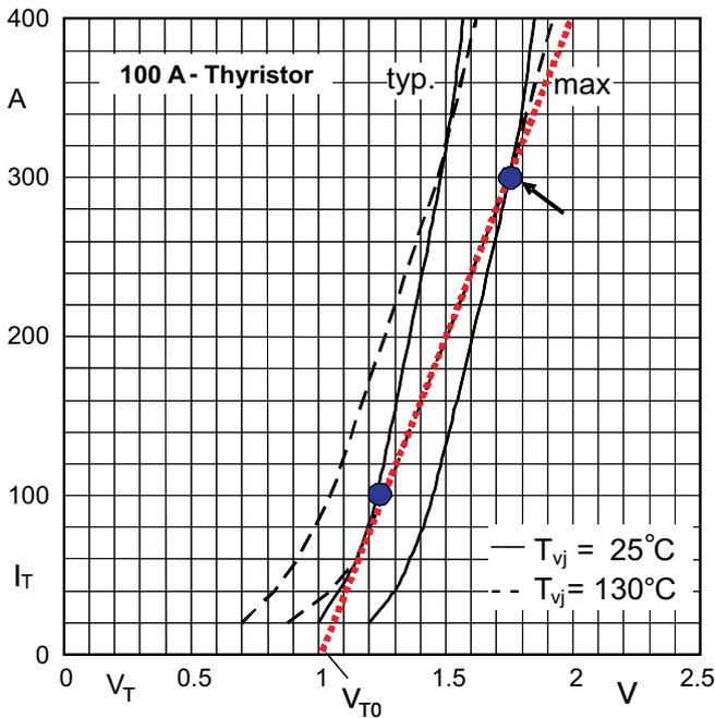
Figure 3.2.15 Thyristor on-state characteristics (typical and maximum) at two different virtual junction temperatures  $T_{vj}$ ; the arrow shows the test limit; dotted red line = on-state slope resistance used to determine  $V_{T(0)}$  and  $r_T$ ;  $r_f$  results from the straight line inclination
