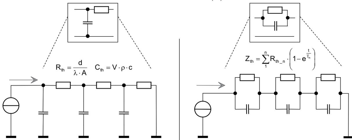
Figure 5.2.7 Mapping of the  $Z_{th}$  four-pole blocks by means of thermal equivalent circuit diagrams; left: conductor-type "physical" equivalent circuit diagram (Cauer network); right: chain-type "mathematical" equivalent circuit diagram (Foster network)
