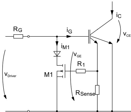
Figure 5.7.11 Short-circuit current limitation by reducing gate-emitter voltage [37]
