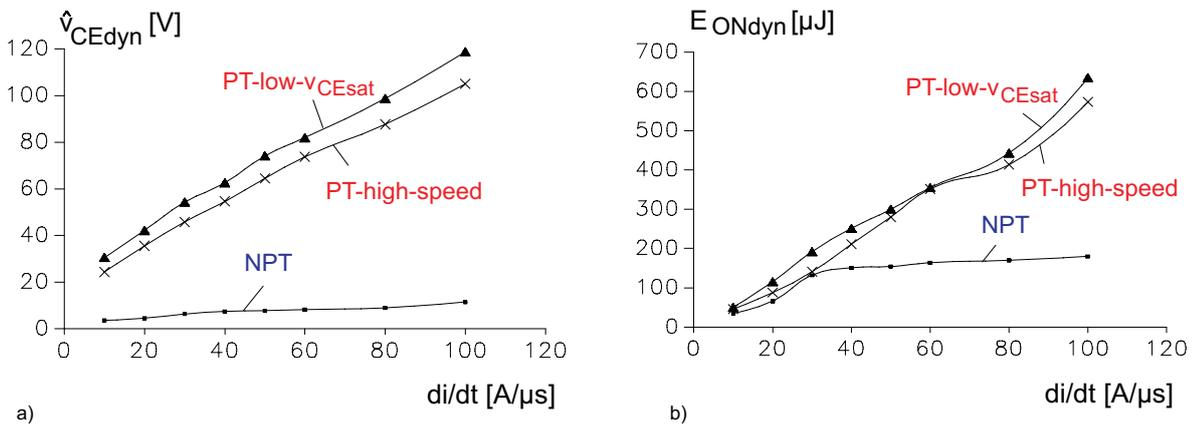
Figure 5.9.10 a) Dynamic on-state voltage amplitude of 1200 V / 50 A NPT and PT IGBT as a function of impressed  $di/dt$  ( $i_L = 30$  A)
