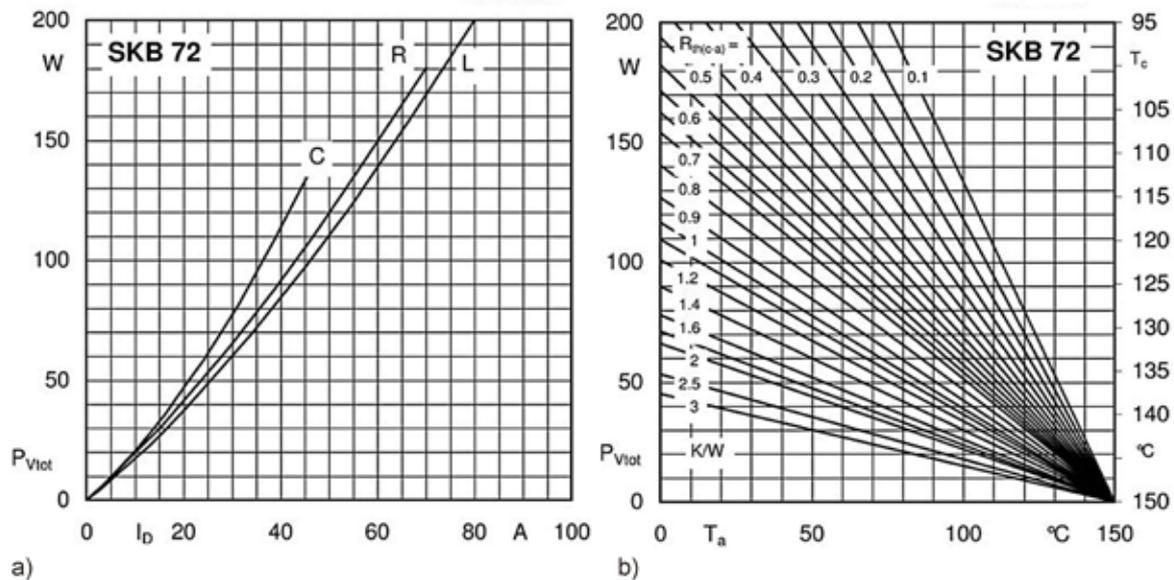
Figure 4.1.11 a) Power dissipation  $P_V$  of a silicon compact rectifier as a function of the rated DC current  $I_D$  for C, R and L load; b) Case temperature  $T_c$  over ambient temperature  $T_a$  for different  $R_{th(c-a)}$
