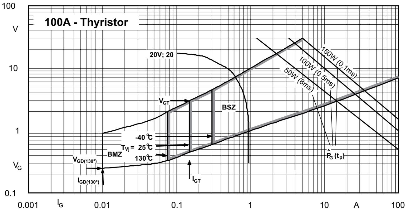
Figure 3.2.21 Trigger current ( $I_G$ ) over trigger voltage ( $V_G$ ) of a 100 A thyristor (spread) with areas of possible and safe triggering.  $\hat{P}_G(t_p)$  is the maximum permissible peak gate power dissipation at a gate current pulse duration  $t_p$ ; the curve labelled "20 V; 20  $\Omega$ " is the characteristic of a trigger device for 20 V no-load voltage and 20  $\Omega$  internal resistance.
