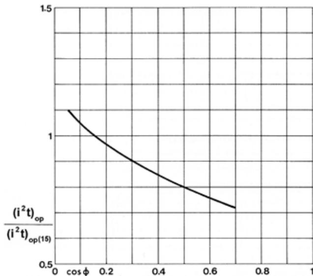
Figure 4.4.20 Operating  $(i^2t)$  value of a semiconductor fuse, in relation to the value for  $\cos \varphi = 0.15$ , shown as a function of the power factor  $\cos \varphi$
