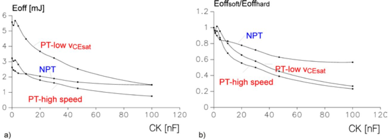
Figure 5.9.12 a) Turn-off losses of 1200 V / 50 A IGBT as a function of the commutation capacitance  $C_K$  ( $v_K = 500$  V;  $i_L = 50$  A)
