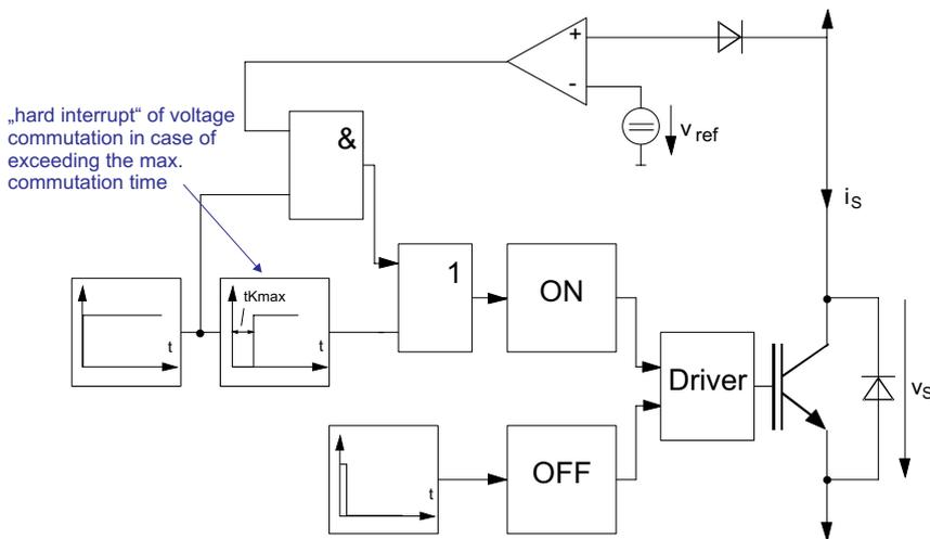
Figure 5.9.7 Modified ZVS: basic principle
