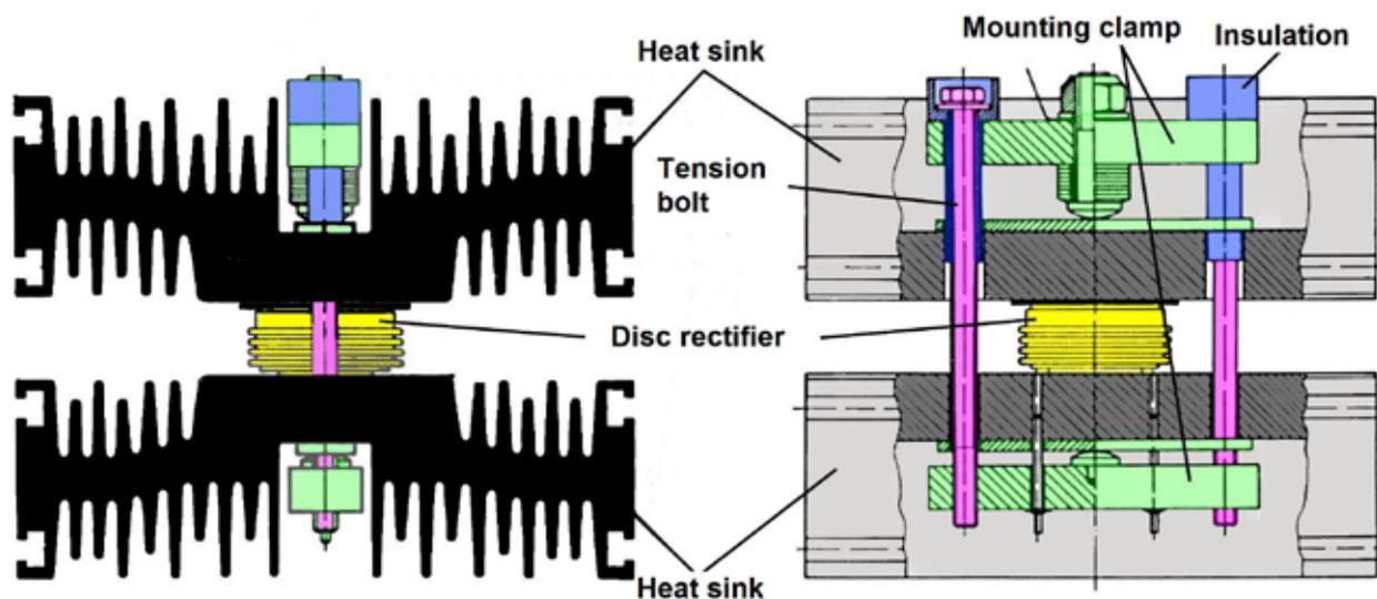
Figure 4.2.8 Double-sided cooling of disc cell using two heat sink profiles
