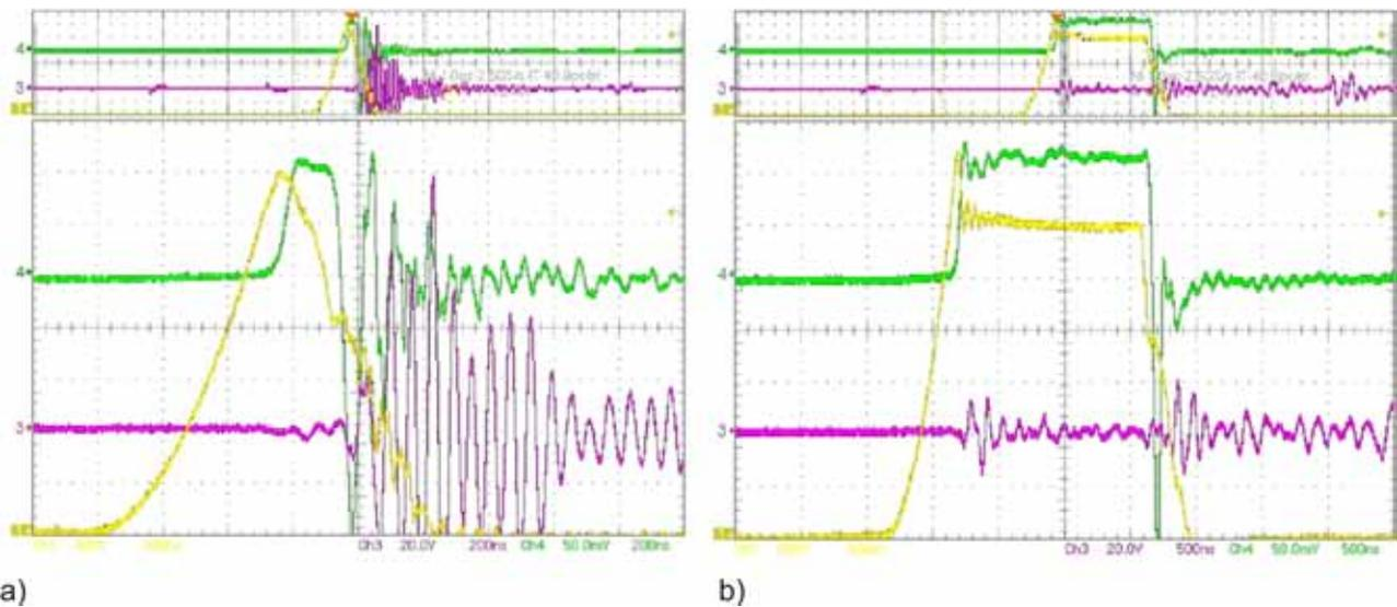
Figure 2.3.13 a) Turn-off at high interference level (pink) at  $V_{CC}=1200$  V ( $V_{AK}$  -yellow) and  $I_F=400$  A (green) at  $t_p=0.8$   $\mu$ s (200 ns/Div); b) Turn-off at "normal" interference level (pink) at  $t_p=2$   $\mu$ s (500 ns/Div)
