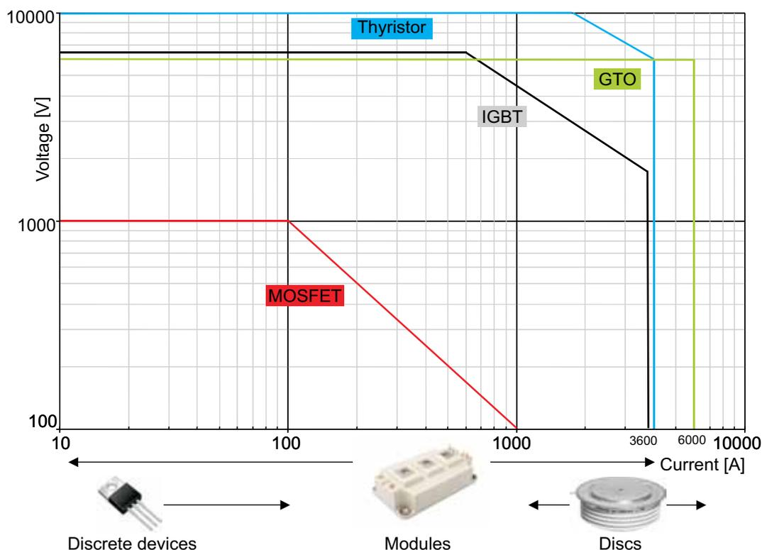
Figure 2.1.1 Present current and voltage limits for controllable power semiconductors
