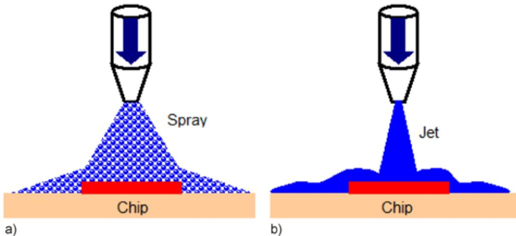
Figure 5.3.22 Principle behind spray cooling (a) and jet cooling (b)
