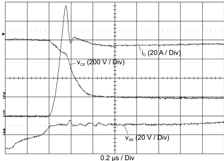
Figure 3.3.8 Turn-on of an IGBT (commutation to the conducting freewheeling diode)
