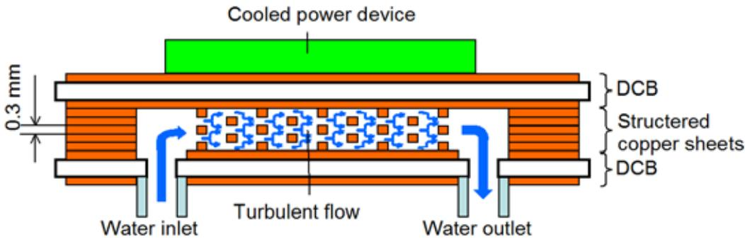
Figure 5.3.20 Diagram showing cross-section of a microchannel cooler
