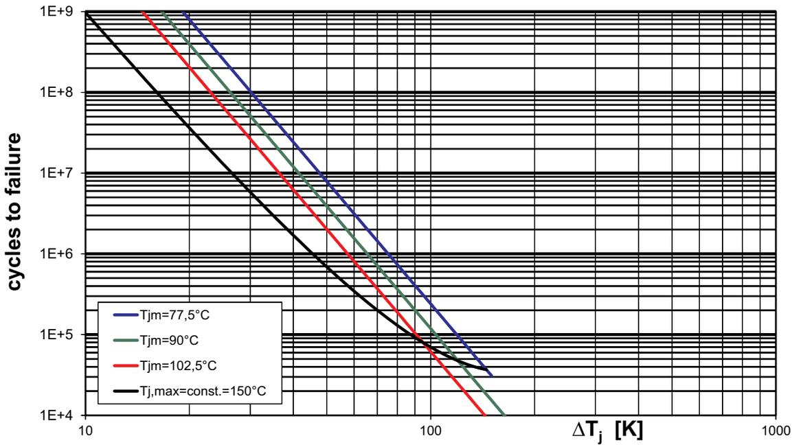
Figure 2.7.17 Dependency of the power cycling value  $N_f$  as a function of the temperature cycling amplitude  $\Delta T_j$  and the mean temperature  $T_{jm}$  for advanced IGBT modules with improved bond wire parameters and/or improved die attach (sintering)
