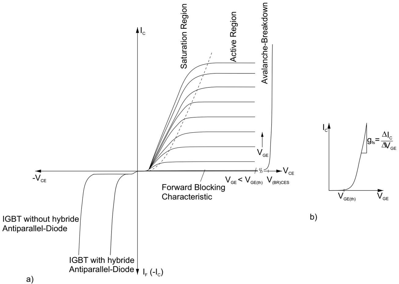
Figure 2.4.5 a) Output characteristics of an IGBT (n-channel enhancement type);
