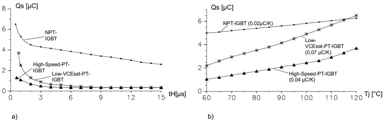
Figure 5.9.16 a) Residual storage charge of PT and NPT IGBT ZCS as a function of hold-off time ( $v_K = 400 \text{ V}$ ,  $i_L = 30 \text{ A}$ ,  $L_K = 10 \mu\text{H}$ )
