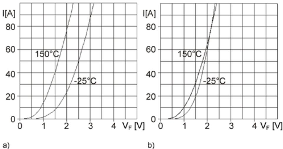
Figure 5.8.2 Temperature dependency of the on-state voltage for different types of diodes
