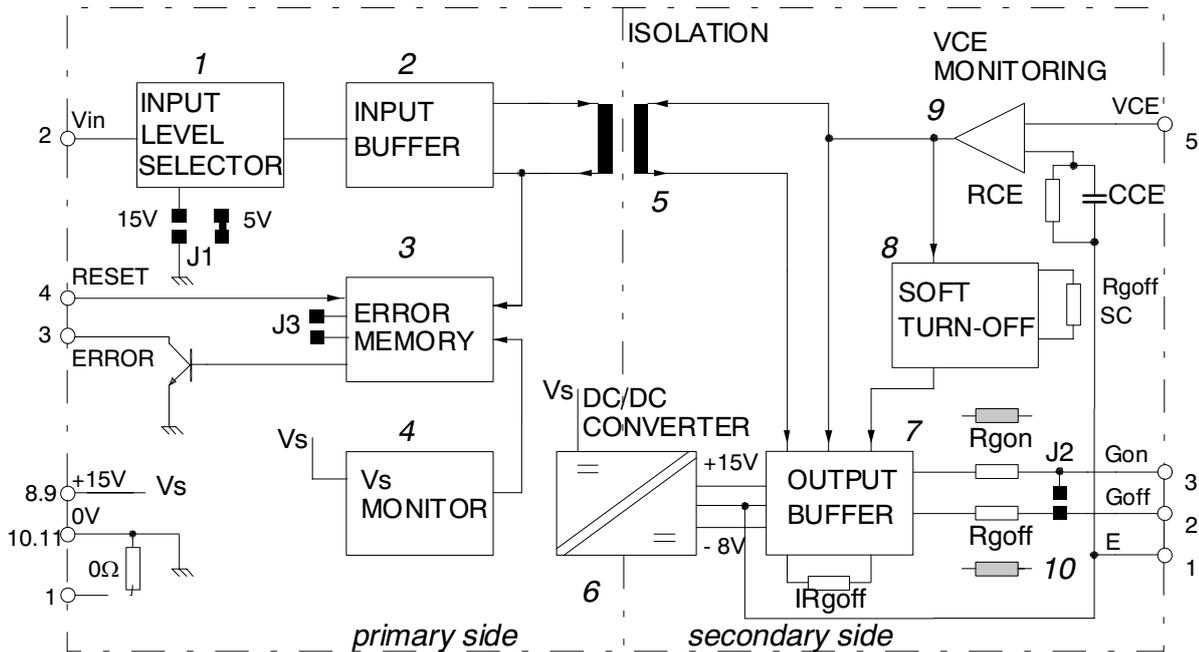
Figure 5.6.15 Block diagram of a SKHI10 driver stage
