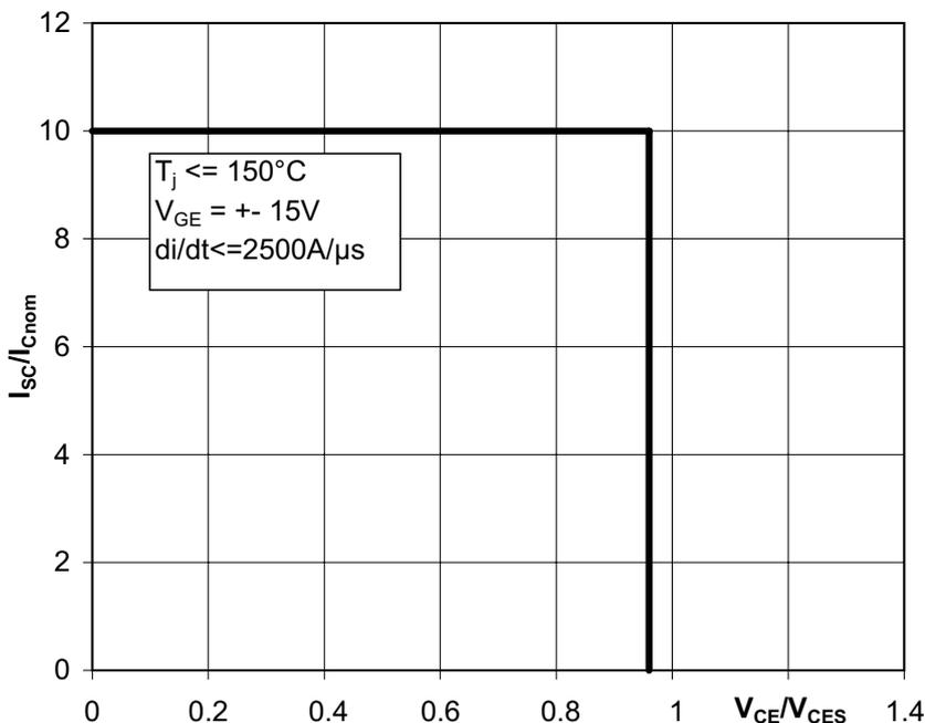
Figure 3.3.29 Safe operating area during short circuit (SCSOA)
