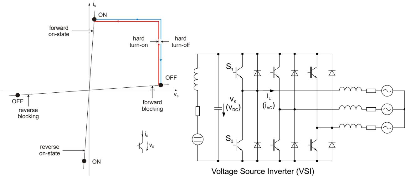
Figure 5.9.2 Operating point characteristic of switch current and voltage for hard switching (IGBT, MOSFET) and typical circuit diagram for voltage source inverter
