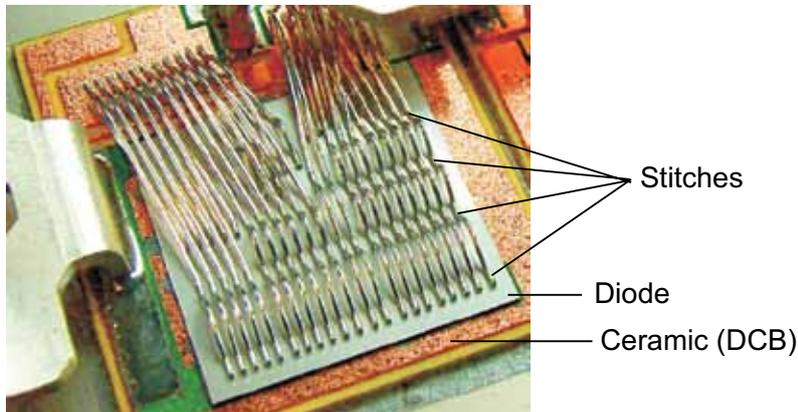
Figure 2.5.3 Many parallel, "multi-stitched" bond wires on a diode chip, 502 mm<sup>2</sup> face.
