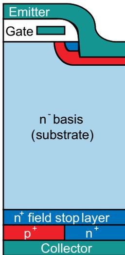
Figure 2.4.14 Structure of an RC-IGBT from ABB [23]
