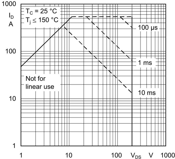
Figure 3.4.5 Safe operating area during single-pulse operation (SCSOA)
