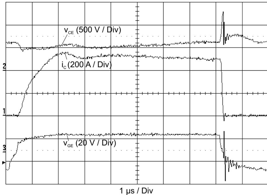
Figure 5.7.4 SC I characteristics of an IGBT
