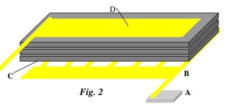
scheme as shown in schematic figure 2 is recommended. The order of printing is the same as above, except that two layers of the bottom termination B is recommended for etching of fine lines. The minimum recommended line width is 2 mils. Three layers of the thermistor paste are printed and fired, followed by top termination D.
