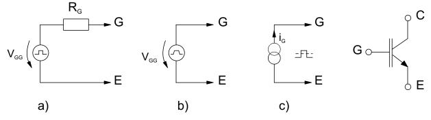
Figure 5.6.1 Gate driving process for MOSFET and IGBT [37] a) Control by resistance, b) Control by voltage, c) Control by current
