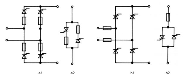
Figure 4.4.15 Possible arrangements for semiconductor fuses in a converter bridge (a1 and b1) and for an AC controllers (a2 und b2); a) Arm fuse or b) Phase fuse
