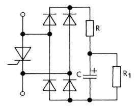
Figure 4.4.3 Single-thyristor snubber networks using an auxiliary bridge
