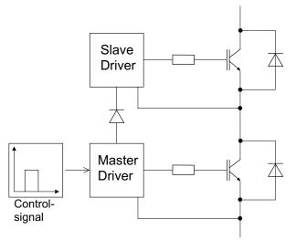
Figure 5.8.23 Basic principle behind the master / slave concept
