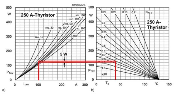
Figure 4.1.5 a) Mean forward dissipation  $P_{TAV}$  over mean forward current  $I_{TAV}$  for different conduction angles; b) Permissible power dissipation  $P_{TAV}$  over ambient temperature  $T_a$  and different  $R_{th(i-a)}$ .
