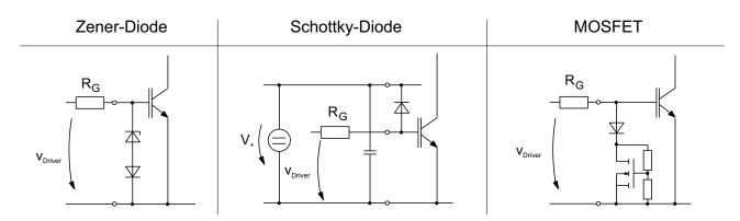
Figure 5.7.21 Simple passive gate voltage limitation circuits (passive gate clamping)
