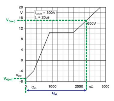
Figure 3.3.6 Gate charge characteristic of an IGBT
