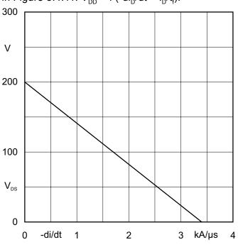
Figure 3.4.11 Drain-source voltage derating versus drain current rate of fall
