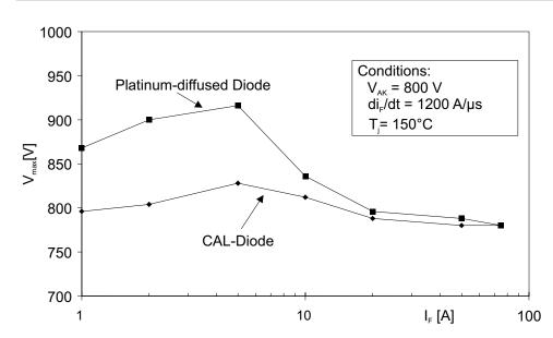
Figure 2.3.10 Peak voltage during commutation in dependence of the forward current as a parameter for diode switching behaviour
