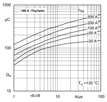
Figure 3.2.28 Reverse recovery charge  $Q_{rr}$  over rate of current fall during switch-off commutation -di/dt for different on-state currents  $I_{TM}$ .
