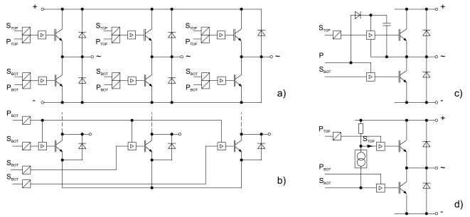
Figure 5.6.12 Selected signal and energy transmission principles STOP, SBOT: control signal for TOP / BOTTOM switch PTOP. PBOT: driving energy for TOP / BOTTOM switch
