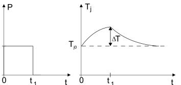
Figure 5.2.10 Time curve of power dissipation and junction temperature in the event of a single power dissipation pulse
