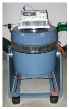
Figure 2.7.4 SKiiP system on a vibrating plate
