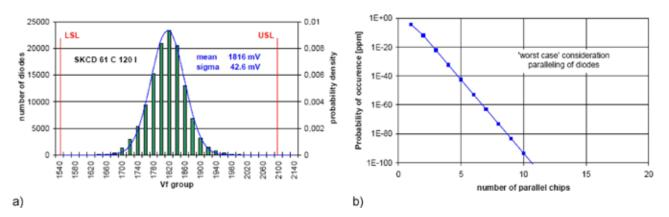
Figure 5.8.3 a) Statistic distribution of diode voltage Vf @ 50 A for 125,000 diode chips; b) Probability of combination 1 x LSL and (n-1) x USL chips for n parallel chips
