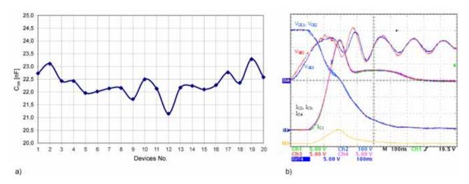
Figure 5.8.5 a) Variation recorded for input capacitance C<sub>ies</sub> of a selection of 450 A Trench2 IGBT modules; b) Switching test with 4 parallel modules (turn-on) with an additional 4.7 nF external capacitance between module gate and emitter
