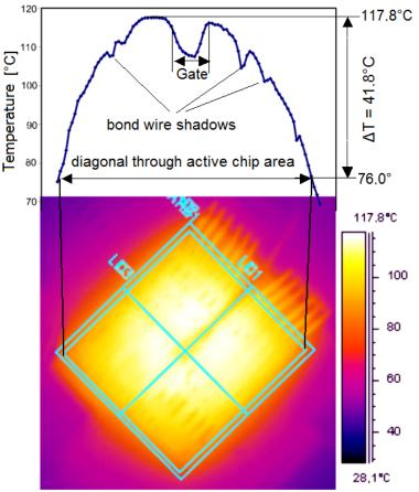
Figure 3.2.1 The bottom part of the illustration shows the infrared image of a live, bonded chip with an active area of 12x12 mm<sup>2</sup>; the scale on the right represents the assignment of temperatures to pseudo colours. The upper part of the illustration shows the evaluation of the infrared image in reference to the temperature measured across the chip
