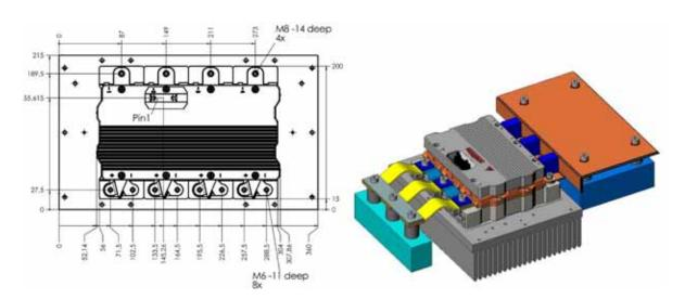
Figure 3.6.4 Power terminals of a SKiiP3
