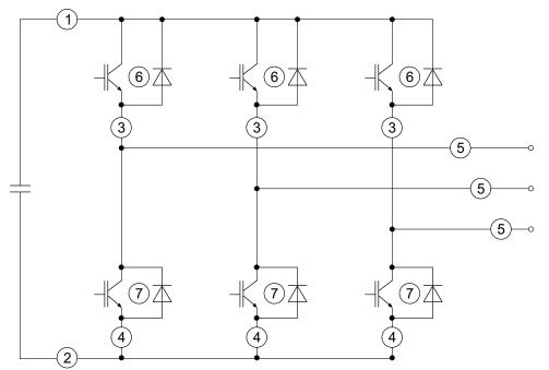
Figure 5.7.9 Voltage source inverter (VSI) with detection points for fault currents
