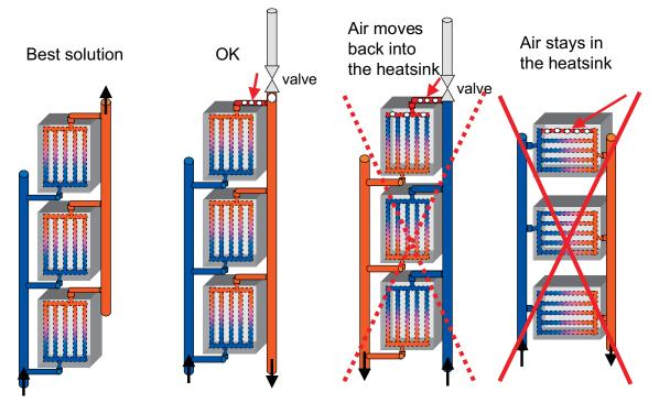
Figure 5.3.19 Setting up the water circuit
