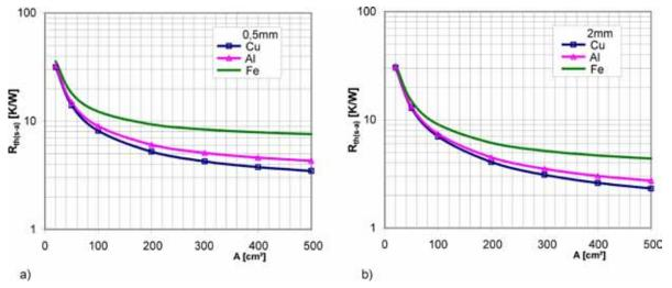
R<sub>th(s-a)</sub> for square bare cooling plates made of steel (Fe), aluminium (AI) and copper (Cu) Figure 4.2.1 over the area A for 0.5 mm plate thickness (left) and 2 mm plate thickness (right) for unobstructed airflow across the surface and approx. 40 K temperature difference  $\Delta T_{(s-a)}$
