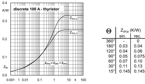
Figure 3.2.4  $Z_{th}$  to case  $(Z_{th(j-c)})$  and to heatsink  $Z_{th(j-s)}$  of a discrete 100 A thyristor, and mathematical auxiliary parameter  $Z_{th(z)}$  to calculate the temperature fluctuation at line frequency for different current conduction angles and waveforms
