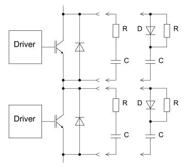
Figure 5.8.19 Passive networks for dynamic voltage symmetry
