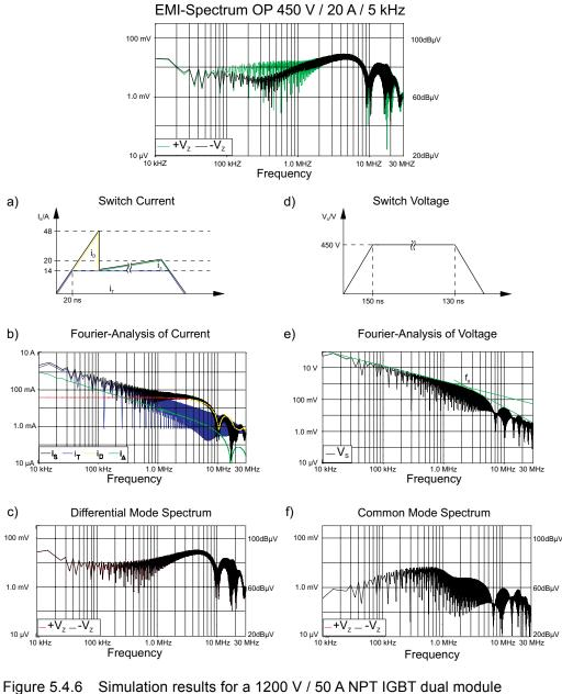
Figure 5.4.6 Simulation results for a 1200 V / 50 A NPT IGBT dual module Operation parameters: DC link voltage V<sub>z</sub> = 450 V; Load current = 20 A Pulse frequency = 5 kHz
