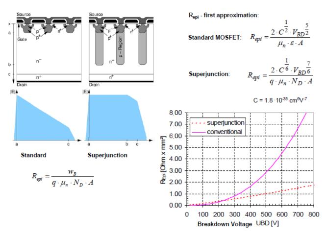
Figure 2.4.22 Comparison of standard and superjunction MOSFET [28]
