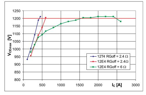
Figure 5.1.1 Voltage load of 450 A IGBT modules at chip level containing T4 or E4 chips, with  $V_{cc}$  = 800 V and T<sub>c</sub> = 25°C upon short circuit turn-off
