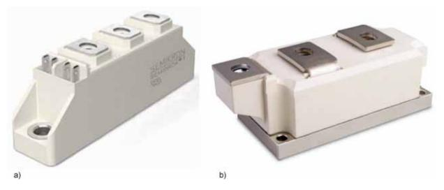
Figure 2.5.36 a) SEMIPACK®1 (soldered chips, soldered / bonded top side, aux. spring contacts) b) SEMIPACK®5 (pressure-contact chips)
