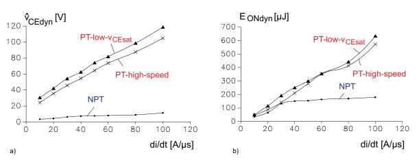
Figure 5.9.10 a) Dynamic on-state voltage amplitude of 1200 V / 50 A NPT and PT IGBT as a function of impressed di/dt ( $i_{L}$  = 30 A)
