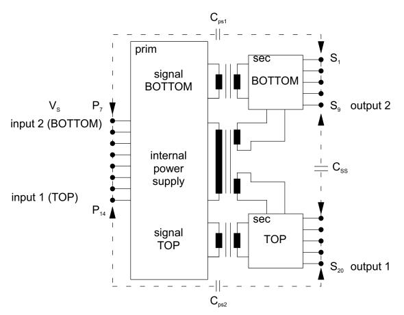
Figure 5.6.13 Diagram of equivalent coupling capacitances in a half-bridge driver with potential isolation C<sub>ps1</sub>: C<sub>ps2</sub>: Capacitance between primary and BOTTOM secondary side
