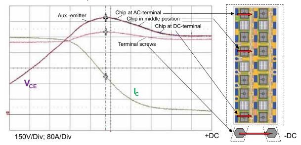
Figure 2.5.26 Overvoltage reading in the SKiM93 during turn-off at different chip positions and the outer terminals at 6.7 kA/µs, time scale = 20 ns/Div
