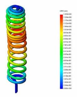
Figure 2.5.6 Natural frequency analysis of a non-loaded spring with a 1.1 kHz resonance frequency in Z-direction
