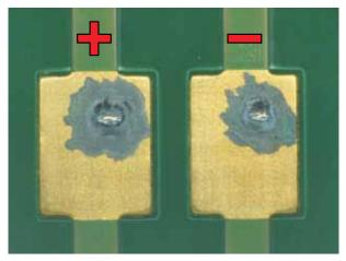
Figure 2.7.6 Pollution gas test of MiniSKiiP springs on a PCB (3 ppm H<sub>2</sub>S, 40°C, 80% RH, 2,000 h, 15 V)
