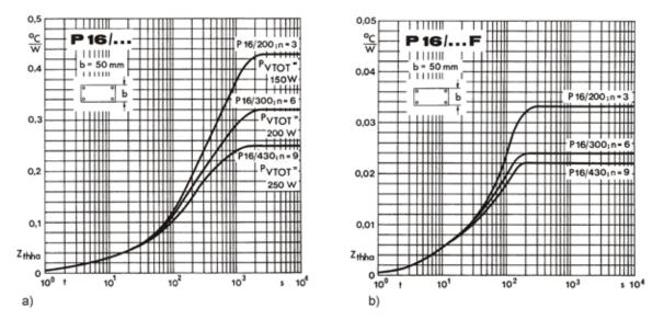
Z<sub>th(s-a)</sub>(t) characteristics for different P16 heatsink lengths/length in [mm], number of heat Figure 5.3.6 sources n; a) in case of free convection with different power dissipation values; b) for forced air cooling
