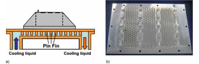
Figure 5.3.12 Pin-fin-liquid cooler to enlarge the heat transfer area; a) Schematic drawing; b) Photograph of the cooling side
