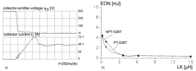
Figure 5.9.14 a) Low-loss turn-on of an NPT IGBT ( $L_{\kappa}$  = 3.6 µH)
