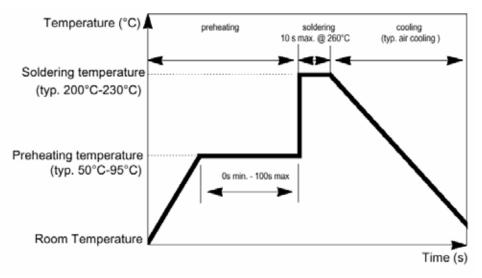
Figure 6.3.9 Wave soldering profile for SEMIKRON power modules
