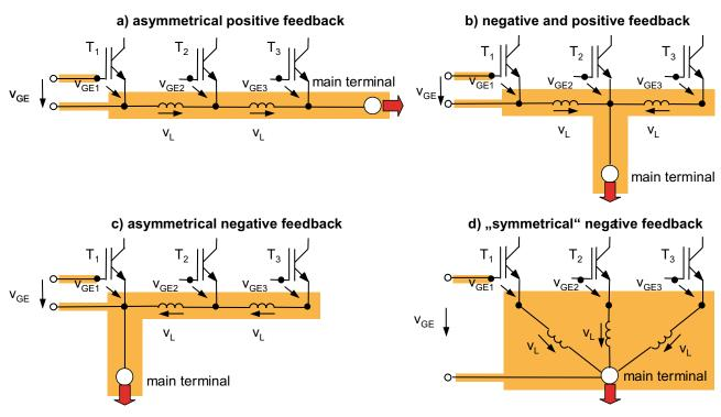
Figure 5.8.10 Examples of positive and negative main current feedback in the driver circuit Example a) shows different degrees of positive feedback, causing transistor T<sub>2</sub> to turn on **more quickly** than  $T_1 \cdot v_{GE3} = v_{GE} + 2 \cdot v_L > v_{GE1} = v_{GE}$ . In example b)  $T_2$  has positive feedback and  $T_3$  negative feedback
