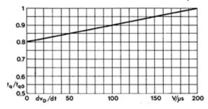
Figure 3.2.25 Typical characteristic of circuit commutated turn-off time  $t_q$  (where  $dv_D/dt = 200 \text{ V/}\mu\text{s}$ ) over rate of rise of the repetitive on-state voltage  $dv_D/dt$ .
