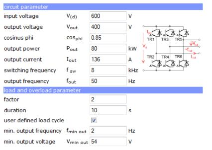
Figure 5.2.17 Entering the electrical ratings and overload conditions
