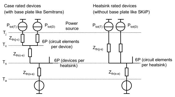
Figure 5.2.5 Simplified thermal equivalent circuit diagram of IGBT and freewheeling diode in a power module: for module with copper base plate (I); for module without base plate (r).
