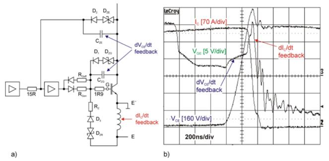
Here, the information on di/dt or dv/dt is obtained by inductance at the emitter or by capacitance at the collector.
