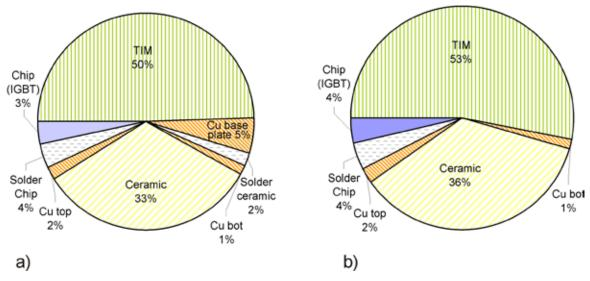
Figure 2.5.16 Influences on the internal thermal resistance of a 1200 V power module, chip surface 9 mm \* 9 mm: a) for DBC substrates (Al<sub>2</sub>O<sub>3</sub>) on Cu base plate, 100 μm TIM;
