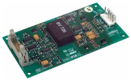
Figure 5.6.14 PCB of a SKHI10 driver stage
