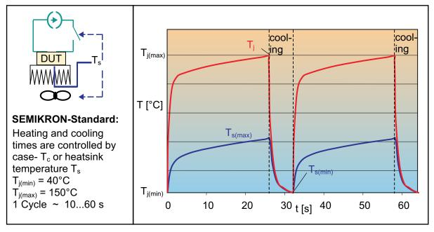
Figure 2.7.3 Power cycling test: test set-up and measurement method
