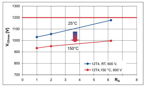
Figure 5.1.2 Voltage load V<sub>CEmax</sub> of a 1200 V /400 A IGBT module with T4 chips at chip level at V<sub>CC</sub> = 600 V and turn-off of I<sub>C</sub> =  $2 \cdot I_{Cnom}$  = 800 A and different external gate resistances and temperatures
