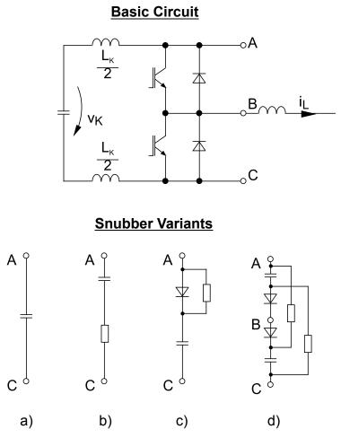
Figure 5.7.12 Passive overvoltage limitation networks (snubbers)
