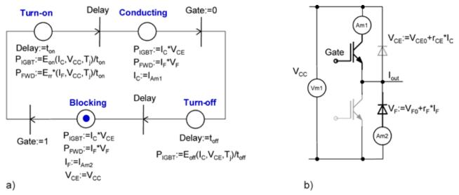
Figure 7.2.1 Semiconductor modelling using state models; a) State description; b) Electric equivalent circuit
