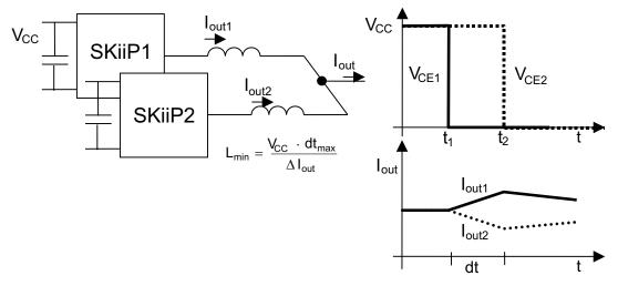
Figure 5.8.15 Dynamic decoupling of parallel individual modules using inductances in the load terminal paths
