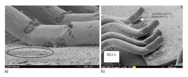
Figure 2.7.12 Bond wire damage; a) Breakage and lift-off at the marked area; b) Failure due to bond wire lift-off [48]
