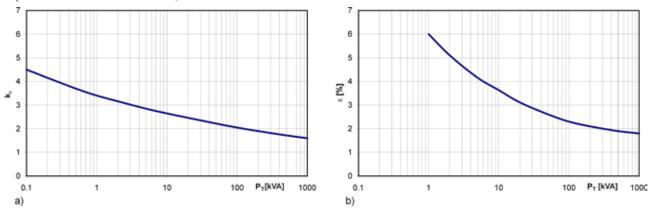
Figure 4.4.8 a) Factor  $k_3$  as a function of the rated power  $P_T$  of the converter transformer; b) Magnetising current  $\epsilon$  (as a percentage of the rated current) of a converter transformer as a function of its rated power  $P_T$ .
