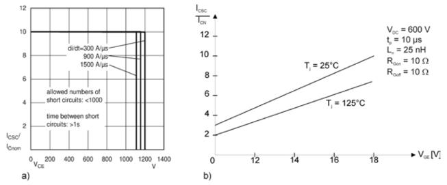
Figure 5.7.7 Short circuit specifications of an IGBT
