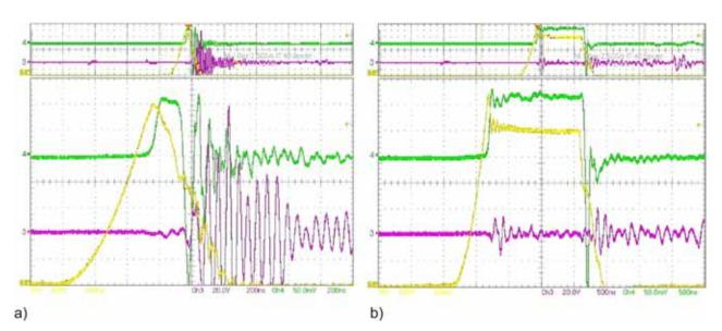
Figure 2.3.13 a) Turn-off at high interference level (pink) at  $V_{cc}$ =1200 V ( $V_{AK}$ -yellow) and  $I_F$ =400 A (green) at  $t_p$ =0.8 µs (200 ns/Div); b) Turn-off at "normal" interference level (pink) at  $t_p$ =2 µs (500 ns/Div)
