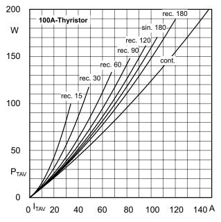
Figure 3.2.16 Mean on-state power dissipation P<sub>TAV</sub> as a function of the mean on-state current I<sub>TAV</sub> for pure direct current (cont.), 180° half sine waves (sin.180) and rectangular current pulses from 15° to 180° (rec. 15 to 180).
