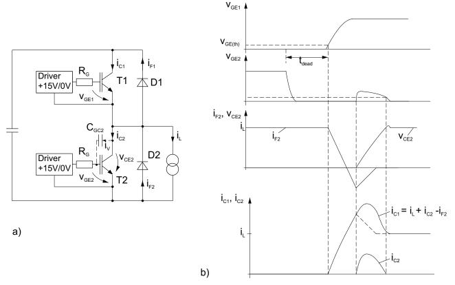
Figure 5.6.3 Cross current in an IGBT bridge arm due to turn-on by dv<sub>CE</sub>/dt feedback of T2 a) Circuit diagram, b) Current and voltage characteristics
