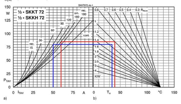
Figure 4.1.10 a)  $P_{TAV}$  as a function of the mean forward current  $I_{TAV}$  for half sine waves (sin. 180), pure DC (cont.) and for rectangular pulses (rec. 15 to 180); b) Permissible power dissipation  $P_{TAV}$  over ambient temperature  $T_a$  for different  $R_{th(j-a)}$ ; all of this data applies to one thyristor alone.
