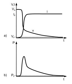
Figure 2.2.10 Current and voltage curves (a) and losses (b) during thyristor turn-on.
