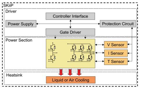
Figure 3.6.1 Principle layout of a SKiiP IPM (left: "GB" topology, right: "GD" topology)
