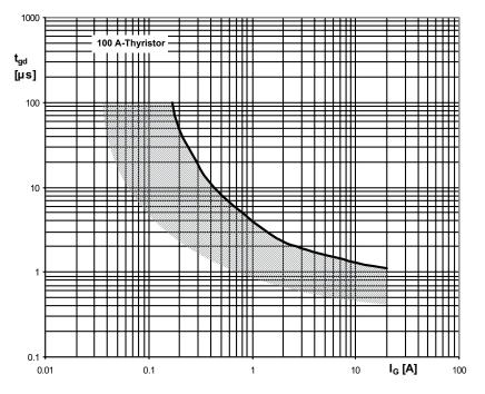
Figure 3.2.19 Typical dependency of a thyristor gate-controlled delay time t<sub>gd</sub> on gate current I<sub>g</sub>; the shaded area represents the variation range.
