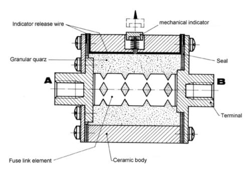
Figure 4.4.16 Cross-section of a semiconductor fuse link
