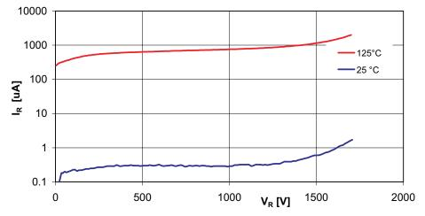
Figure 2.3.6 Example of the reverse current of a 1700 V CAL diode, parameter T<sub>i</sub>
