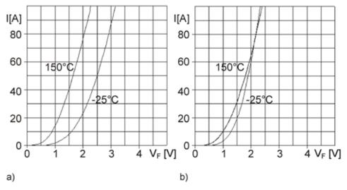
Figure 5.8.2 Temperature dependency of the on-state voltage for different types of diodes a) highly negative temperature coefficient; b) positive temperature coefficient from rated current on (75 A)
