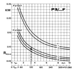
Figure 4.2.11  $R_{th(s-a)}$  for P3 heat sink profile in different lengths, equipped with n = 1 - 6 components, as a function of the air volume  $V_{air}/t$  or air velocity  $v_{air}$
