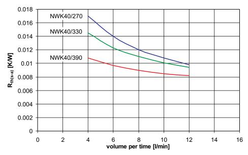
Figure 5.3.15 Thermal resistance as a function of the volumetric flow rate of the NWK40 with SKiiP3 for various lengths and a 50:50 water / glycol mixture
