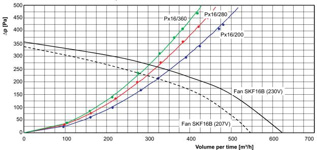
Pressure drop characteristic for Px16/200 ; Px16/280 ; Px16/360
