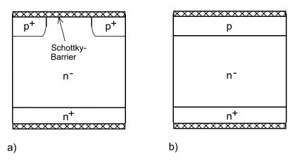
Figure 2.3.4 p-emitter to improve soft recovery behaviour: a) Emitter structures, e.g. merged PIN/Schottky diode b) Fully reduced p-doping
