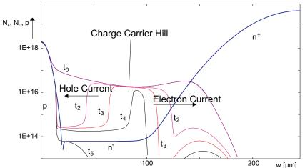
Figure 2.3.11 Diffusion profile and simulation of the decline in charge carriers (hole density) in a snappy diode
