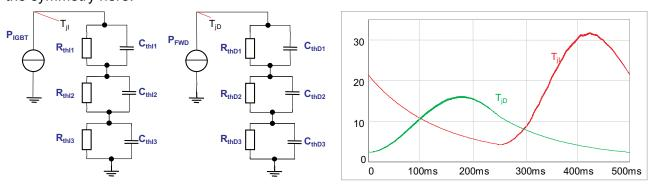
Figure 7.2.3 Thermal equivalent circuit and example of calculated temperature characteristic of a PWM inverter with 2 Hz output frequency
