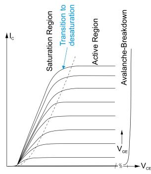
Figure 5.7.8 IGBT desaturation limit
