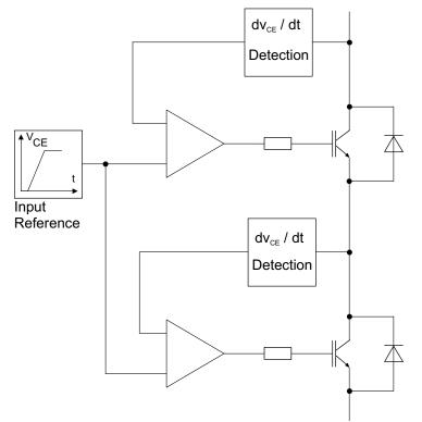
Figure 5.8.21 Dynamic voltage symmetry using dv/dt control
