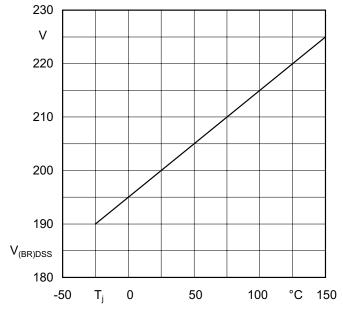
Figure 3.4.10 Typical drain-source breakdown voltage versus temperature
