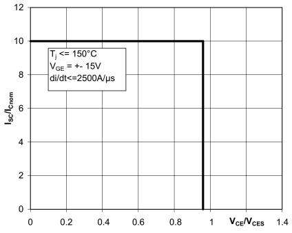
Figure 3.3.29 Safe operating area during short circuit (SCSOA)
