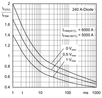
Figure 4.1.4 Permissible error-induced overcurrents I<sub>F(OV)</sub> in relation to surge forward current I<sub>FSM</sub> for different reverse voltage conditions directly following the last sinusoidal half-wave as a function of time t
