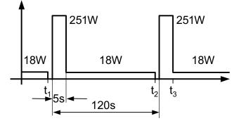
Figure 4.1.3 Power dissipation  $P_{FAV}$  over time for the example given. At the times  $t_1$  and  $t_2$ , the diode is switched off and back on again immediately.
