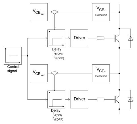
Figure 5.8.20 Principle behind switching time correction
