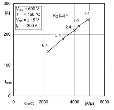
Figure 3.3.25 Peak reverse recovery current of the freewheeling diode (CAL diode) of an IGBT module
