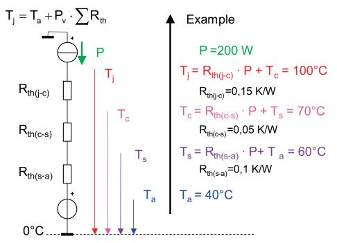
Figure 5.2.8 Temperature calculation under stationary conditions
