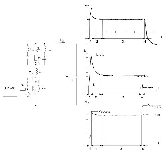
Figure 5.7.5 Equivalent circuit and principle characteristics of SC II, [37]
