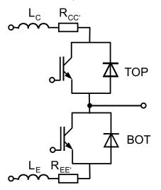
Figure 3.3.13 Parasitic inductances and resistances of an IGBT module  $L_c + L_E = L_{cE}$ , and  $R_{cC'} + R_{EE'} = R_{CC'+EE'}$
