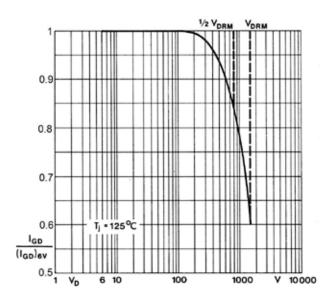
Figure 3.2.22 Gate non-trigger current  $I_{GD}$  at  $V_{D}$  = 6 V as a function of off-state voltage  $V_{D}$ ; typical characteristic for a thyristor with a max. repetitive peak off-state voltage  $V_{DRM}$  = 1600 V
