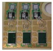
Figure 2.6.1 Current shunts (made by Isabellenhütte) in the emitter path of a MiniSKiiP IGBT module
