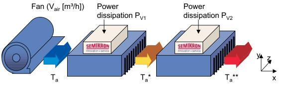
Figure 5.3.26 Thermally stacked, air-cooled layout, split into sectors with different air pre-heating The general formula is:
