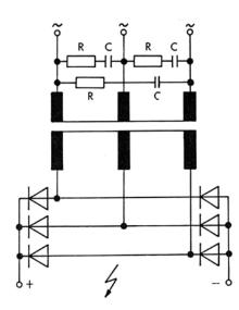
Figure 4.4.7 Primary-side snubber of a high-voltage transformer
