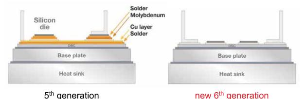
Figure 2.5.14 Development of Semipack rectifier bridges: thermal resistance reduced by the omission of layers
