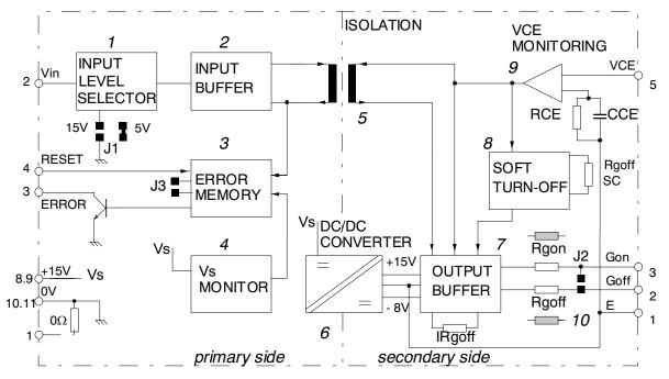
Figure 5.6.15 Block diagram of a SKHI10 driver stage
