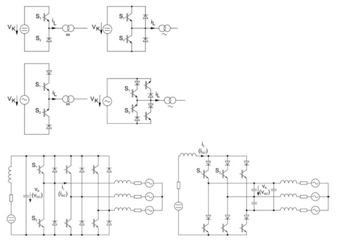
Figure 1.2.3 HS commutation circuits and examples of typical circuits
