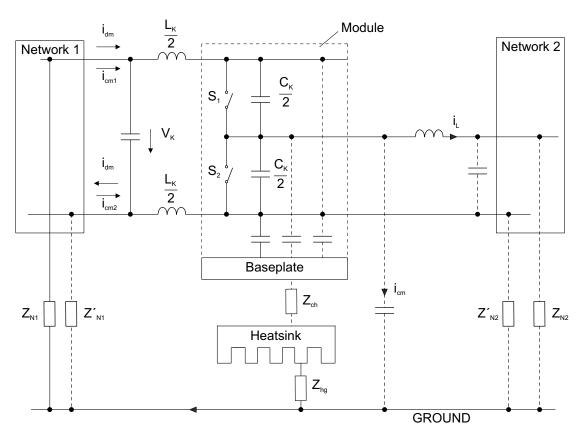
Figure 5.4.3 Equivalent commutation circuit with noise propagation paths [60]
