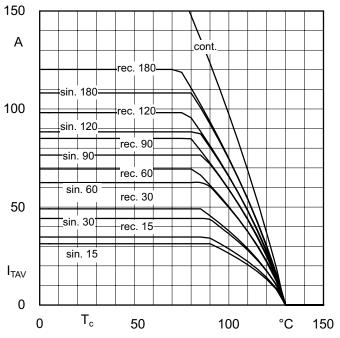
Figure 3.2.13 Mean on-state currents  $I_{TAV}$  of a 100 A thyristor over case temperature  $T_c$  for direct current (cont.), rectangular pulses (rec.) and (controlled) half sine waves (sin.) with different current conduction angles  $\Theta$
