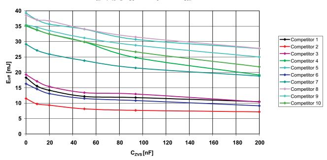
E<sub>off</sub>=f(C<sub>κ</sub>) @ V<sub>DC</sub>=600V; I<sub>C</sub>=300A; R<sub>Goff</sub>=3Ohm
