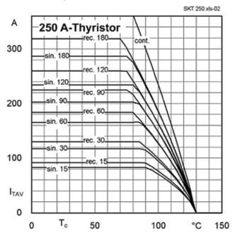
Figure 4.1.7 Mean forward current  $I_{TAV}$  as a function of the case temperature  $T_c$  for pure DC (cont.), controlled half sine waves (sin.) and rectangular pulses (rec.). Parameter: Conduction angle  $\Theta$
