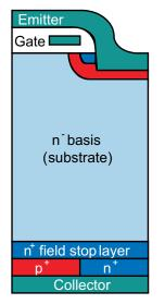
Figure 2.4.14 Structure of an RC-IGBT from ABB [23]
