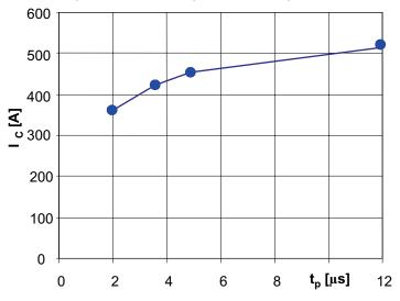
Figure 5.1.4 Necessary current derating to meet V<sub>CE(max)</sub> for very short turn-on times t<sub>p</sub> of a 1200 V-IGBT4 with V<sub>CC</sub> = 800 V and T<sub>c</sub> = 25°C
