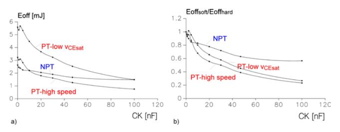
Figure 5.9.12 a) Turn-off losses of 1200 V / 50 A IGBT as a function of the commutation capacitance C<sub> $\kappa$ </sub> (v<sub> $\kappa$ </sub> = 500 V; i<sub>L</sub> = 50 A)
