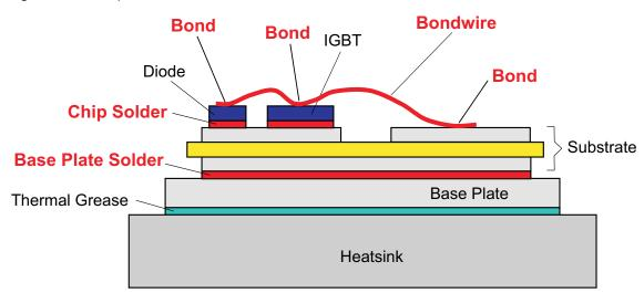
Figure 2.7.8 explains the structural details relevant to the IGBT module life.
