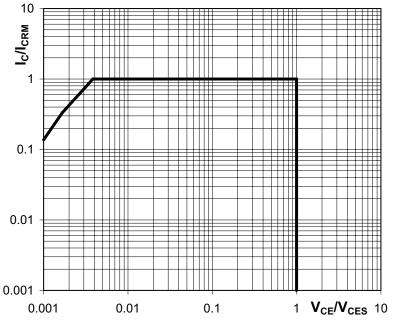
Figure 5.7.3 SOA diagram for an IGBT
