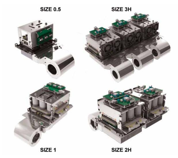
Figure 5.5.3 SEMIKUBE assemblies with optional radial fans
