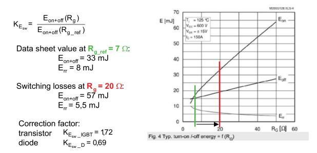
Figure 5.2.20 Establishing the correction factor for switching losses for modified driver parameters
