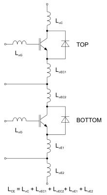
Figure 2.5.24 Parasitic inductances in a dual IGBT module
