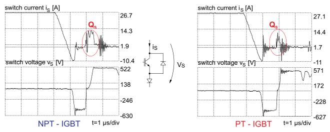
Figure 5.9.15 Turn-off characteristics of 1200 V / 50 A NPT and PT IGBT at the same operating point ( $t_{H}$  = 1.3 µs, L<sub>K</sub> = 10 µH)
