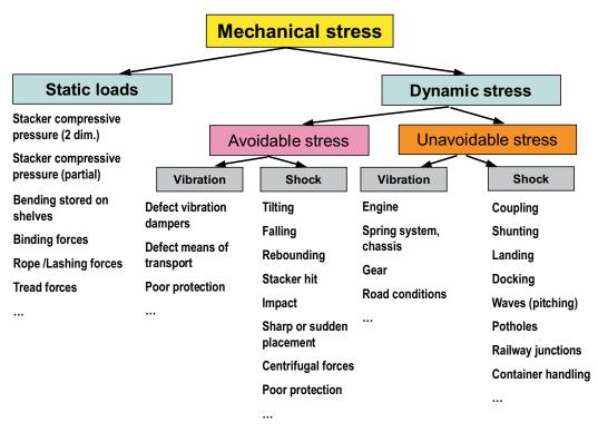
Figure 6.2.2 Types of mechanical stress according to the environmental conditions listed in EN 60721-3-3
