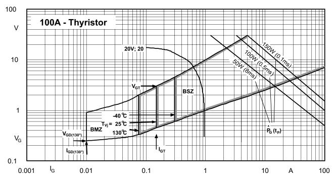
Figure 3.2.21 Trigger current ( $I_G$ ) over trigger voltage ( $V_G$ ) of a 100 A thyristor (spread) with areas of possible and safe triggering.  $\hat{P}_G(t_p)$  is the maximum permissible peak gate power dissipation at a gate current pulse duration  $t_p$ ; the curve labelled "20 V; 20  $\Omega$ " is the characteristic of a trigger device for 20 V no-load voltage and 20  $\Omega$  internal resistance.
