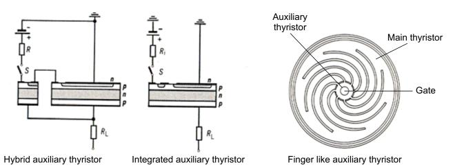
Figure 2.2.11 Trigger energy amplification using an auxiliary thyristor (amplifying gate).
