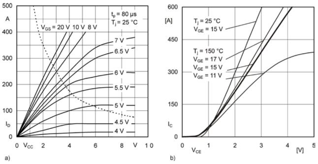
Figure 5.6.4 Forward characteristics versus control voltage  $V_{GG^+}$  a) Power MOSFET module b) IGBT module
