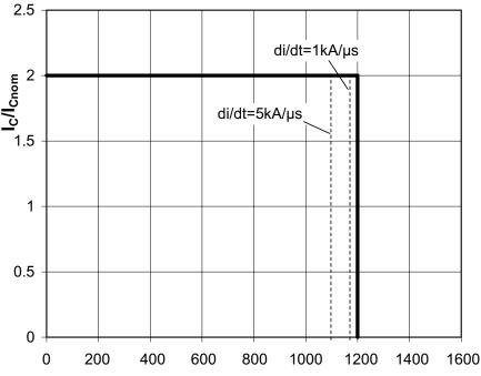
Figure 3.3.28 Turn-off safe operating area (RBSOA) of a 1200 V IGBT; T<sub>i</sub> < T<sub>i(max</sub>); V<sub>GE</sub>=+-15 V; R<sub>G</sub>=R<sub>G(nom)</sub>
