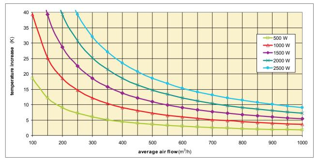
Figure 5.3.28 Temperature difference between incoming and outgoing air as a function of power dissipation  $P_{v_1}$  (W) and the volumetric flow rate,  $T_a = 40^{\circ}C$
