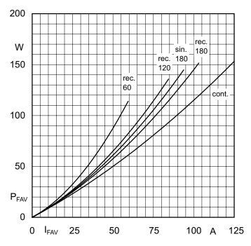
Figure 3.2.10 Mean forward power dissipation P<sub>FAV</sub> over mean forward current I<sub>FAV</sub> of a 70 A diode for pure direct current (cont.), half sine waves 180° (sin. 180) and rectangular current pulses 60° (rec. 60) to 180° (rec. 180)
