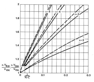
Figure 4.4.6 Time characteristic of the voltages  $V_{DM}$  or  $V_{RM}$  across the thyristor fired last (\_\_\_) and turning off first ( - - - ) for n series connected thyristors ( $V_{VM}$ : Crest value for total terminal voltage, L: Inductance in the commutation circuit, C: Thyristor snubber capacitance).
