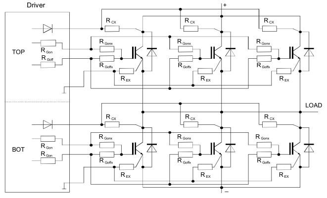
Figure 5.8.12 Parallel connection of IGBT modules
