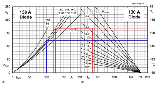
Figure 4.1.2 a) Mean forward power dissipation  $P_{FAV}$  over mean forward current  $I_{FAV}$  for different current waveforms; b) Case temperature  $T_c$  over ambient temperature  $T_a$ ; the parameter is the thermal resistance case-to-air  $R_{th(c-a)}$
