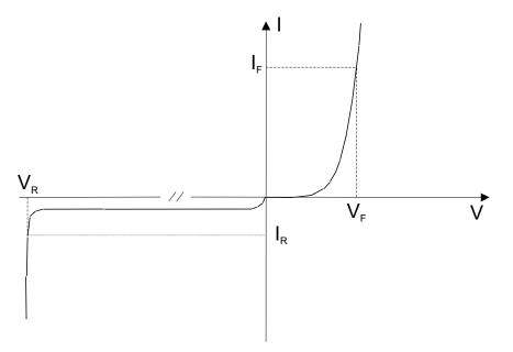
Figure 2.3.5 Definition of reverse and forward diode voltage
