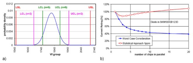
Figure 5.8.4 a) Occurrence of diode combinations of one diode from the LCL with n-1 components from the UCL with a probability of 1 ppm; b) comparison between possible current utilisation under "worst case scenario" conditions with the USL / LSL and current from a statistical point of view
