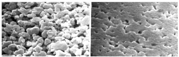
Figure 2.5.1 Silver powder before and after diffusion sintering
