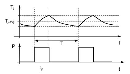
Figure 5.2.12 Temperature curve for periodic pulse load
