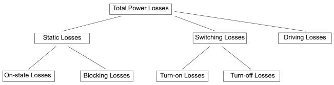
Figure 5.2.1 Individual power losses of power modules used as switches
