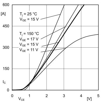
Figure 3.3.15 Typical output characteristics of an IGBT
