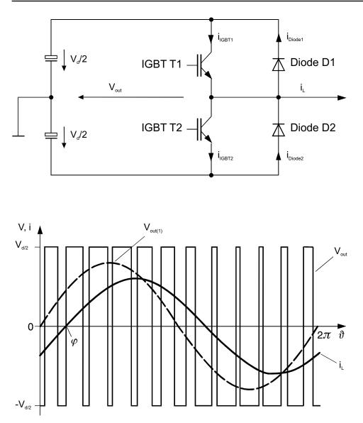
Figure 5.1.6 Basic circuit of a converter phase with IGBT and freewheeling diodes The following can be seen:
