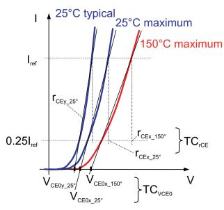
Figure 3.3.5 forward characteristics of an IGBT and definition of the elements of an equivalent straight line
