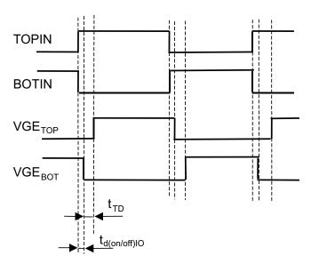
Figure 3.6.12 Delay times of SKiiP control signals
