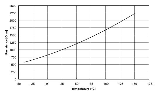
Figure 2.6.4 Characteristic curve of the PTC temperature sensor, type SKCS2Typ100
