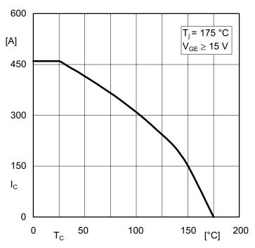
Figure 3.3.16 Derating of collector current versus case temperature
