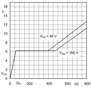
Figure 3.4.13 Typical gate charge characteristic  $V_{GS} = f(Q_G)$
