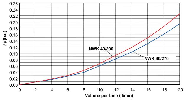
Figure 5.3.14 Pressure drop across a SEMIKRON water cooler (SKiiP3 – NWK40) for 2 different lengths (incl. 90 mm end pieces) dependent on the volumetric flow rate (water-glycol mixture 50%:50%, diagonally opposite inlet / outlet, T<sub>a</sub>= 55°C)
