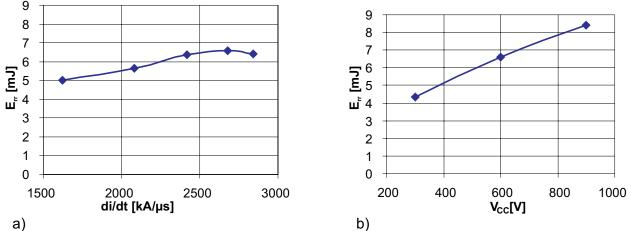
Figure 2.3.18 Dependencies of 100 A/1200 V CAL diode switching losses; a) on di/dt (@100 A, 600 V, 150 °C);
