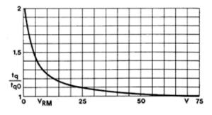
Figure 3.2.26 Typical characteristic of circuit commutated turn-off time t<sub>q</sub> (where t<sub>q0</sub> at V<sub>RM</sub>  $\ge$  75 V) over peak reverse voltage V<sub>RM</sub>.
