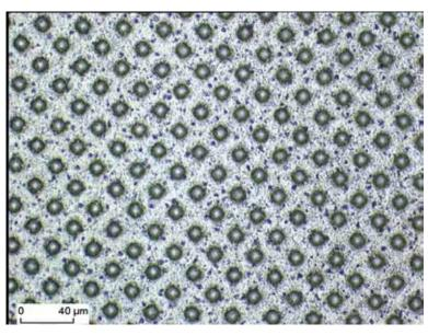
Figure 2.4.1 Cell structure (emitter metallisation) of a Trench IGBT3
