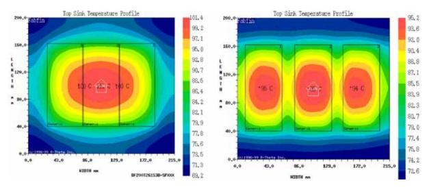
Figure 5.3.3 Effect of better distribution of heat sources across the heatsink surface, temperature simulation on the heatsink surface
