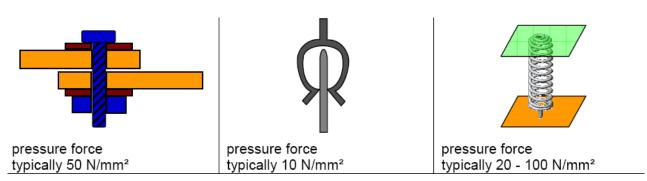
Figure 2.5.7 Comparison of contact pressures of detachable electrical connections (from left to right: screw, plug-in, spring contact)
