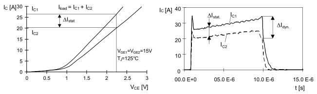
Figure 5.8.1 Stationary current distribution in two parallel IGBT with different output characteristics.
