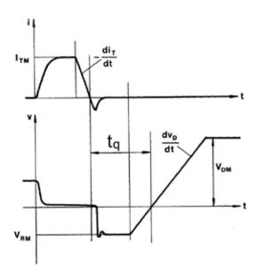
Figure 3.2.23 Main current i and main voltage v of a thyristor over time during commutation from on-state to off-state; the circuit commutated turn-off time t<sub>q</sub> is the shorted time interval during which an applied direct off-state voltage will not trigger the thyristor
