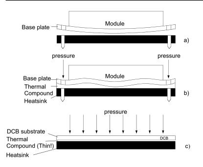
Figure 2.5.18 Problems arising through contact of power module to heat sink
