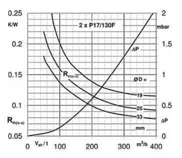
Figure 4.2.9 R<sub>th(s-a)</sub> of P17 heat sink of 130 mm in length for disc cells with double-sided cooling and pressure drop  $\Delta P$  between air entry and exit as a function of the air volume in the given time  $V_{air}/t$ . ØD is the diameter of the contact element of the disc cell.
