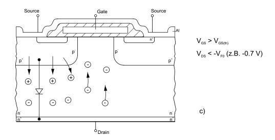
Figure 2.4.18 Inverse operation of a power MOSFET [26] ; a) Closed channel (bipolar current flow); b) Open channel and low negative V<sub>DS</sub> (unipolar current flow); c) Open channel and high negative V<sub>DS</sub> (combined current flow) Generally speaking, the bipolar inverse diode can be utilised within the current limits specified for the MOSFET. Practice, however, often shows that
