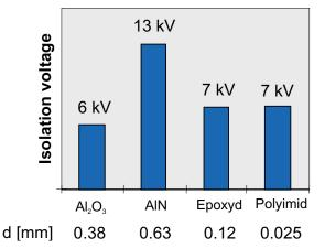
Figure 2.5.12 Insulation voltages for different insulating substrates
