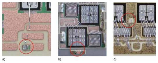
Figure 2.6.6 Temperature sensors in power semiconductor modules, a) Insulated PTC chip in a MiniSKiiP (0.7 mm clearance); b) Insulated NTC component in a SEMiX (1.6 mm clearance); c) non-insulated chip sensor on collector potential in SKiiP4 module
