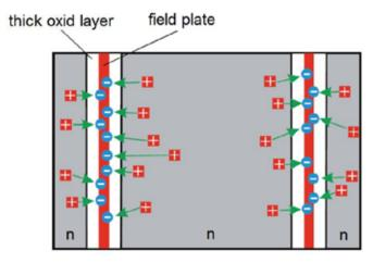
Figure 2.4.23 Principle layout of an OptiMOS [29]
