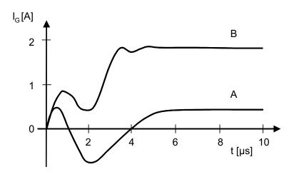
Figure 3.2.20 Gate current I<sub>G</sub> over time, triggered by an insufficiently (curve A) and a sufficiently designed (curve B) driver unit.
