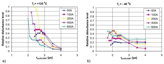
Figure 2.3.14 Relative interference level related to the maximum value at 200 A and 125°C for IGBT turnoff signals of different durations as a function of current and temperature (a)  $T_j$ =125°C, b)  $T_i$ =-40°C)
