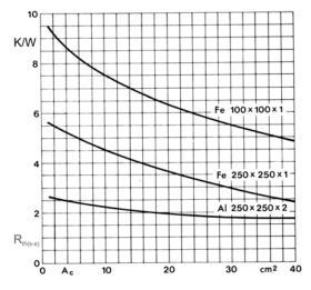
Figure 4.2.4 R<sub>th(s-a)</sub> of cooling plates with the given dimensions (in mm) made of steel (Fe) and aluminium (Al) as functions of the contact surface area  $A_c$  of the heat generating component for low cooling plate / air temperature difference. The cooling air must be able to flow unobstructed across the entire surface.
