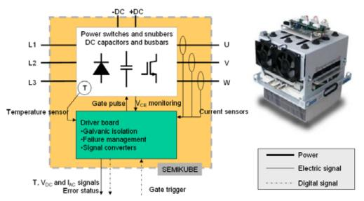
Figure 5.5.1 Functions and principle layout of a SEMIKUBE
