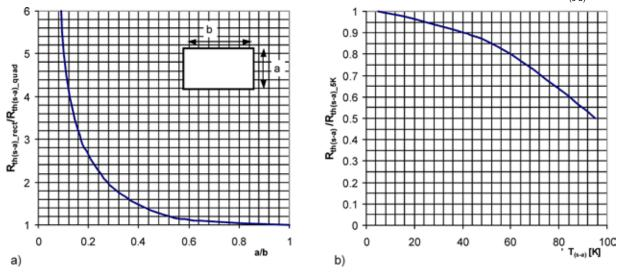
Figure 4.2.2 a) Relative change in  $R_{th(s-a)}$  for non-quadratic cooling plates (r) in dependence of side length ratio a/b; b) Relative change in  $R_{th(s-a)}$  of a cooling plate as a function of the temperature difference between cooling plate ( $T_s$ ) and the inflowing air ( $T_a$ ) in relation to a value at  $T_s$ – T<sub>2</sub> = 5 K
