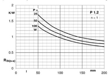
Figure 4.2.7 R<sub>th(s-a)</sub> for various lengths of P 1.2 heat sink with one centrally mounted component and various power dissipation levels P for natural cooling
