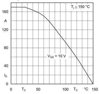
Figure 3.4.9 Drain current derating versus case temperature
