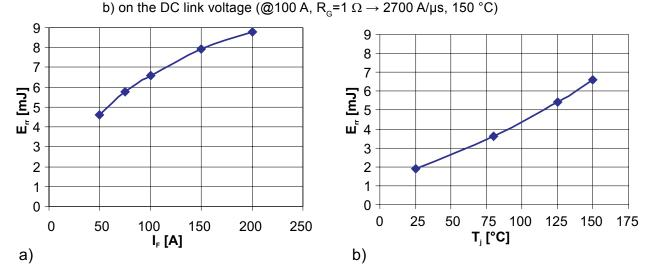
Figure 2.3.19 Dependencies of switching losses of a 100 A/1200 V CAL diode; a) on I<sub>F</sub> (R<sub>G</sub>=1  $\Omega$ , 600 V, 150 °C); b) on junction temperature (100 A, 600 V, R<sub>G</sub>=1  $\Omega$ )
