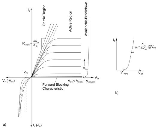
Figure 2.4.17 a) Output characteristics of a power MOSFET (n-channel enhancement type) b) Transfer characteristic  $I_p = f(V_{GS})$
