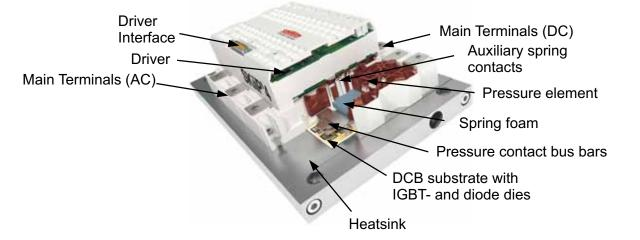
Figure 2.5.40 Basic structure of a 4th-generation SKiiP
