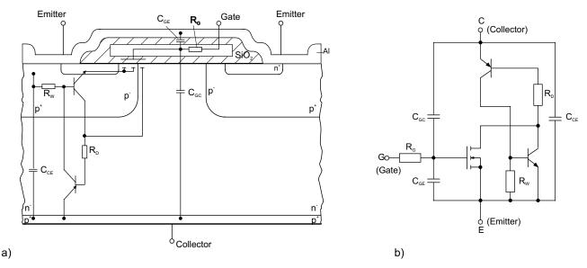
Figure 2.4.4 IGBT cell (NPT structure, planar gate) including the key parasitic elements;
