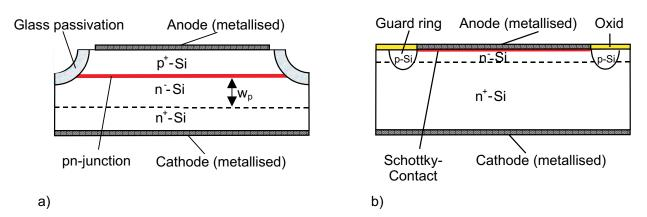
Figure 2.2.3 Schematic layout of a pn-diode (a) and a Schottky diode (b); The glassivation and the guard ring with oxide cover provide protection from environmental impacts and stabilize reverse currents.
