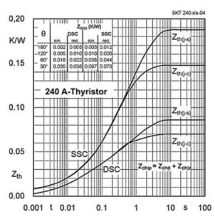
Figure 4.1.8  $Z_{th}$  of a thyristor for SSC and DSC
