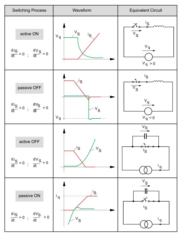
Figure 1.1.1 Basic switching processes
