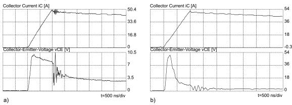
Figure 5.9.9 a) di/dt-impression in a 1200 V / 50 A-NPT-IGBT (di/dt = 50 A/ $\mu$ s; i<sub>L</sub> = 50 A) b) di/dt-impression in a 1200 V / 50 A-PT-IGBT (di/dt = 50 A/ $\mu$ s; i<sub>L</sub> = 50 A)
