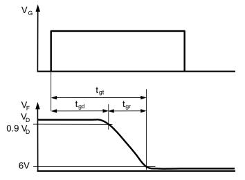
Figure 3.2.18 Gate voltage  $v_{\rm g}$  and forward voltage (instantaneous values)  $v_{\rm F}$  at the moment of thyristor triggering.
