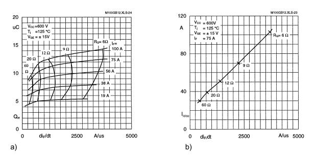
Figure 5.6.6 Recovered charge Q<sub>rr</sub> (a) and peak reverse recovery current I<sub>RRM</sub> (b) of the free-wheeling diodes in an IGBT module (e.g. SKM100GB123D) versus commutation speed -di<sub>F</sub>/dt of the diode current
