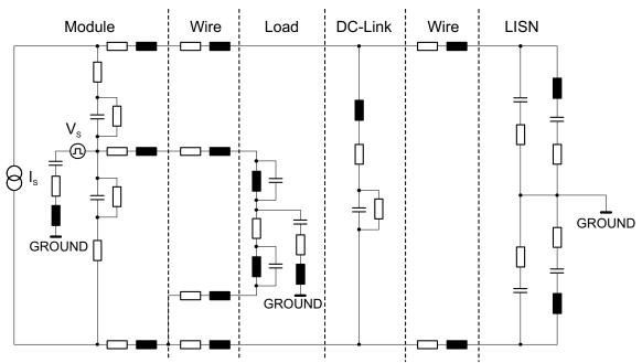
Figure 5.4.4 EMI equivalent circuit of a step-down converter [38]
