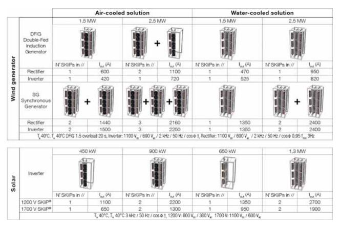
Figure 5.5.5 Current and power output ratings achievable with SEMISTACK RE platforms based on SKiiP3
