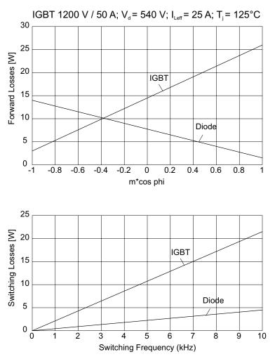
Figure 5.1.7 Switching and forward on-state losses of IGBT and freewheeling diode in a frequency converter
