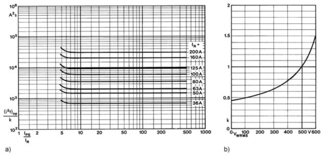
Figure 4.4.19 a) Operating i<sup>2</sup>t values (i<sup>2</sup>t)<sub>op</sub> divided by the factor k, as a function of the prospective shortcircuit current I<sub>PS</sub>, in relation to the fuse rated current I<sub>N</sub> for semiconductor fuses of 35 A -200 A; b) Factor k as a function of the recovery voltage V<sub>wRMS</sub>
