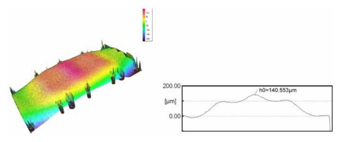
Figure 2.5.17 Measurement of PrimPack FF650R17IE4 base plate by Infineon
