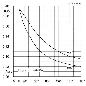
Figure 3.2.3 R<sub>th(j-c)</sub> of a discrete 100A thyristor multiplied by a corrective factor to calculate the temperature fluctuation as a function of the current conduction angle  $\Theta$  and current waveform
