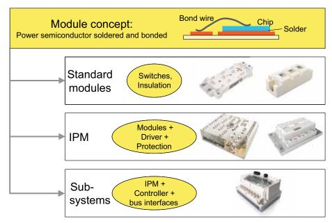
Figure 2.1.3 Power module integration levels
