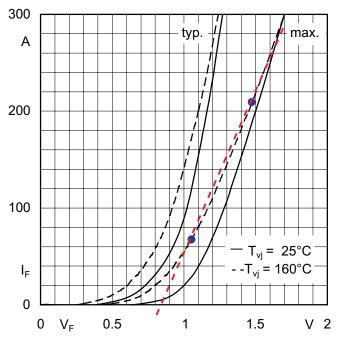
Figure 3.2.9 Forward characteristics (typical and maximum values) of a rectifier diode at two different virtual junction temperatures  $T_j$ ; dotted red line = forward slope resistance used to determine  $V_{(T0)}$  and  $r_f$ ;  $r_f$  results from the line inclination
