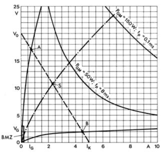
Figure 4.3.2 Gate current  $(I_G)$  – gate voltage  $(V_G)$  characteristic of a thyristor in linear scheme; dotted output characteristic,  $V_0$  – no-load voltage and  $I_K$  – short-circuit current of the driver device; dash-dotted output characteristic of the control terminal – cathode of a typical thyristor
