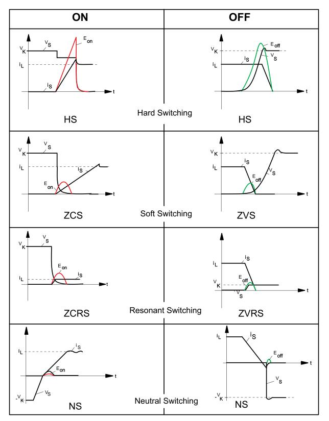
Figure 1.1.2 Types of switching processes ( $v_{\kappa}$  = driving commutation voltage,  $i_{L}$  = load current to be commutated)
