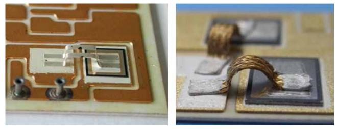
Figure 2.5.2 Sintered silver bands [31] or copper litz wires [32] as substitutes for conventional bond wire connections
