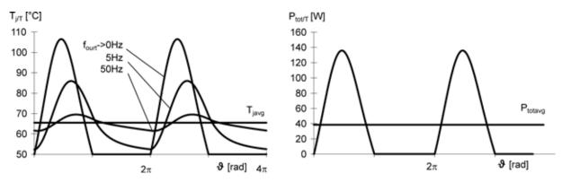
Figure 5.2.13 Simulated junction temperature and power dissipation characteristics of a 1200 V / 50 A-IG-BT in inverter mode for different fundamental output frequencies; [37]  $v_d = 540$  V;  $i_{1eff} = 25$  A,  $f_s = 8$  kHz; cos  $\phi = 0.8$ ; m = 0.8;  $T_h = 50^{\circ}$ C
