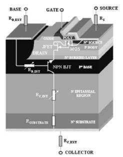
Figure 2.4.15 ESBT structure and equivalent circuit [24]
