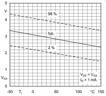
Figure 3.4.14 Gate-source threshold voltage versus temperature
