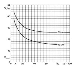
Figure 4.2.3 R<sub>th(s-a)</sub> of a 1.5 mm thick PCB copper lamination, single-sided lamination, layer thickness 35  $\mu$ m and 70  $\mu$ m, as a function of the area A. Any mounting position, provided unobstructed airflow across the entire surface is ensured.
