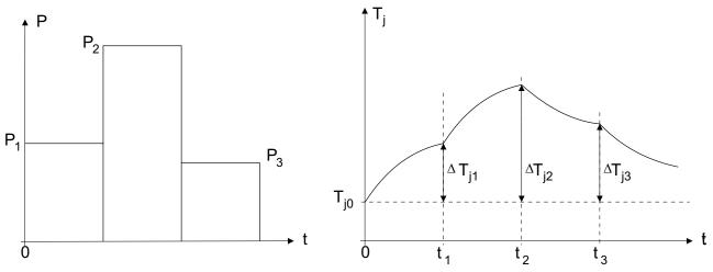
Figure 5.2.11 Time curve of power dissipation and junction temperature in the event of a one-off sequence of m power dissipation pulses
