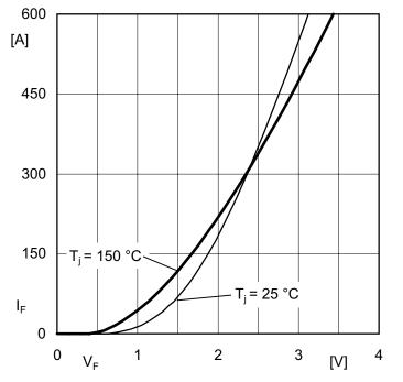
Figure 3.3.24 Forward characteristics of an inverse diode (CAL diode)
