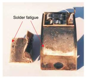
Figure 2.7.10 34 mm module with torn off DBC (light-coloured areas show solder fatigue)
