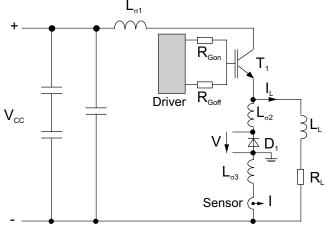
Figure 2.3.15 Reverse recovery test circuit
