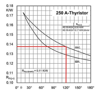
Figure 4.1.6 R<sub>th(j-c)</sub> as a function of the conduction angle  $\Theta$  for controlled half sine waves (sin.) and rectangular pulses (rec.)
