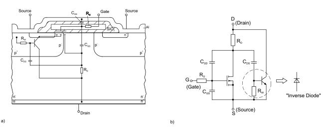
Figure 2.4.16 Power MOSFET cell including the key parasitic elements a) Parasitic elements in the cellular structure; b) Equivalent circuit diagram with parasitic elements
