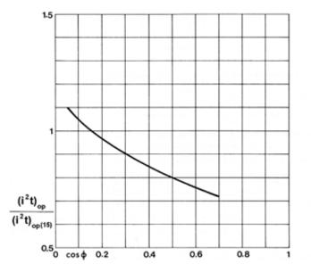
Figure 4.4.20 Operating (i<sup>2</sup>t) value of a semiconductor fuse, in relation to the value for  $\cos \varphi = 0.15$ , shown as a function of the power factor  $\cos \varphi$
