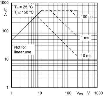
[Fig. 2] Maximum permissible safe operating area during single-pulse operation (SOA)
