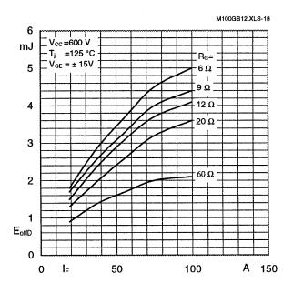
Figure 5.6.7 Free-wheeling diode turn-off losses E<sub>offD</sub> versus R<sub>G</sub> of the transistor during turn-on
