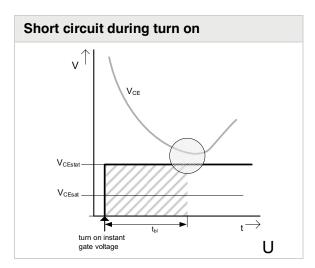
Figure 5.6.11 Possible scenarios for saturation voltage control triggering
