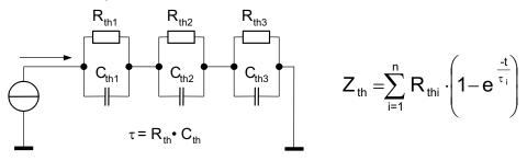
Figure 3.3.14 Dynamic thermal model, where  $\tau_i = R_{thi} \cdot C_{thi}$
