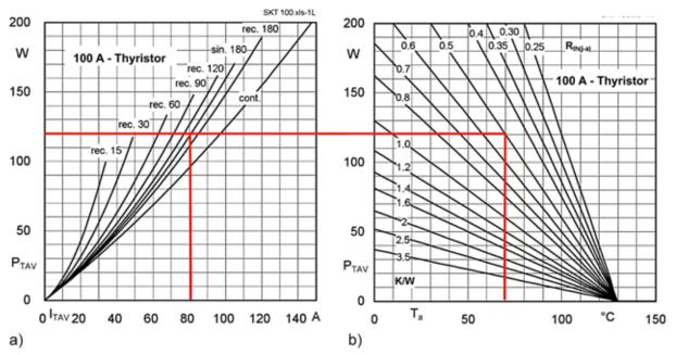
Figure 3.2.27 a) Mean on-state power dissipation  $P_{TAV}$  over mean on-state current  $I_{TAV}$  for different current waveforms; b) Permissible ambient temperature  $T_a$  over thermal resistance junction-to-ambient  $R_{th(i-a)}$  including the contact thermal resistance case-to-heatsink
