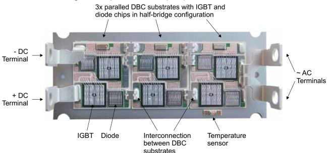
Figure 2.5.45 Internal structure of a SEMiX3 module
