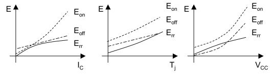
Figure 7.2.2 Example of dependency of switching losses on  $I_c, T_i$  and  $V_{cc}$
