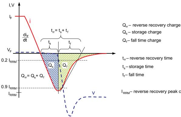
Q<sub>s</sub> – storage charge Q<sub>f</sub>-fall time charge
