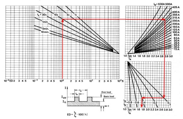
Figure 4.4.18 Alignment chart for the determination of the permissible overcurrent of semiconductors fuses in intermittent operation with and without load
