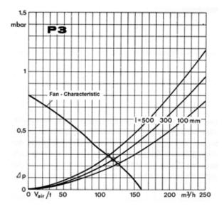
Figure 4.2.10 Diagrams showing pressure drop ∆p for different lengths I of P3 heat sink as a function of air volume V<sub>air</sub>/t, as well as the volume of air moved by the fan as a function of the negative pressure (fan characteristic). The points of intersection constitute the resulting volume of air for the given combination of fan / heat sink profile.
