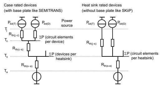
Figure 3.3.10 (Static) thermal models for modules with and without base plate
