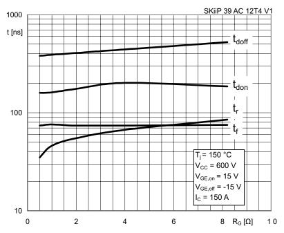
Figure 5.1.9 IGBT4 switching times dependent on the external gate resistance R<sub>g</sub>
