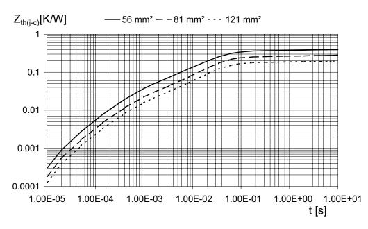
Figure 2.5.22 Time curve of thermal impedances  $Z_{th(j-c)}$  of a module with  $Al_2O_3$  DBC substrate for different chip areas [37]
