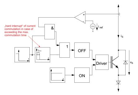
Figure 5.9.8 Modified ZCS: basic principle
