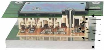
Preasure top with screw Printed circuit board PCB Case Contact spring Bond wire Chip Ceramic substrate DCB Heatsink
