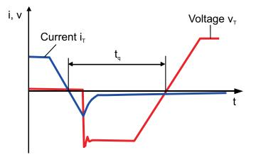
Figure 2.2.13 Current i<sub> $\tau$ </sub> and voltage v<sub> $\tau$ </sub> curves of a thyristor during turn-off and circuit commutated recovery time t<sub>a</sub>
