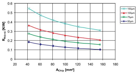
Figure 2.5.20 R<sub>th(c-s)</sub> of a base plate module in relation to a single chip as a function of the chip area and thickness of the thermal paste layer for undisturbed heat spreading
