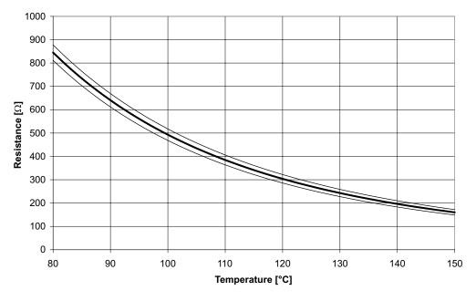
Figure 2.6.5 NTC sensor characteristic in its relevant temperature range incl. tolerance
