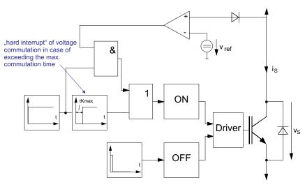
Figure 5.9.7 Modified ZVS: basic principle
