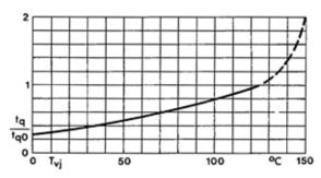
Figure 3.2.24 Typical characteristic of circuit commutated turn-off time  $t_q$  (where  $t_{q0}$  at  $T_j = 125^{\circ}$ C) over virtual junction temperature  $T_j$ .
