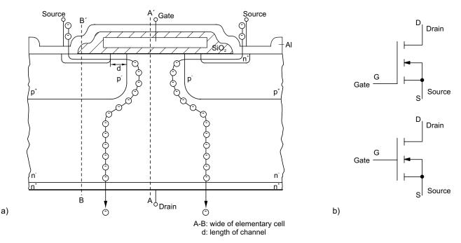
Figure 2.4.2 Power MOSFET with vertical structure and planar gate; a) Charge carrier flow in on-state; b) Circuit symbols
