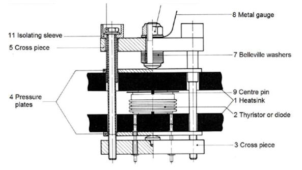
Figure 6.4.1 shows a diagram of a clamping fixture.
