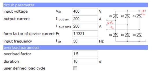
Figure 4.1.13 Example of parameter input for a rectifier bridge in SemiSel
