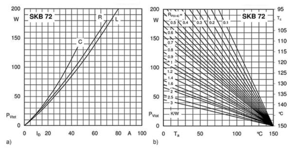
Figure 4.1.11 a) Power dissipation  $P_v$  of a silicon compact rectifier as a function of the rated DC current  $I_D$  for C, R and L load; b) Case temperature  $T_c$  over ambient temperature  $T_a$  for different  $R_{th(c-a)}$
