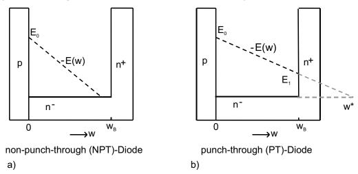
Figure 2.3.7 Diode dimensioning for triangular (a) and trapezoidal (b) field shape for  $0 \le w \le w_{_B}$
