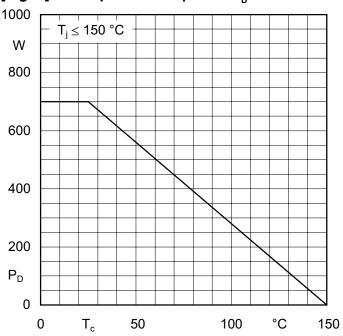
[Fig. 1] Rated power dissipation  $P_p$  as a function of case temperature  $T_c$
