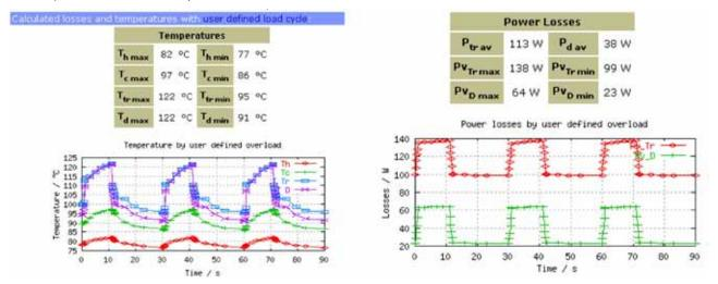
Figure 5.2.24 Presentation of results for temperatures and losses for a user-defined load cycle
