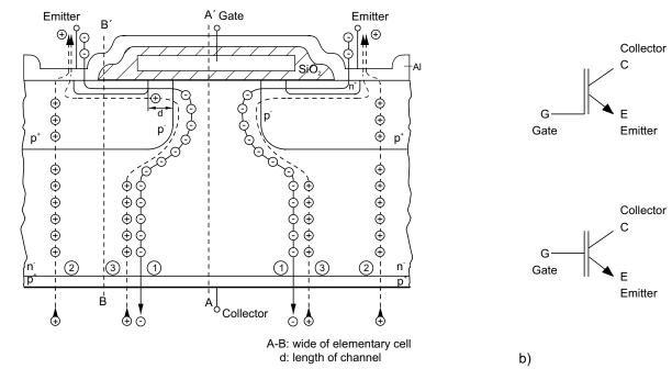
Figure 2.4.3 IGBT with vertical structure and planar gate;
