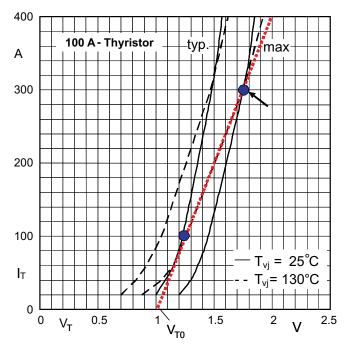
Figure 3.2.15 Thyristor on-state characteristics (typical and maximum) at two different virtual junction temperatures  $T_{vj}$ ; the arrow shows the test limit; dotted red line = on-state slope resistance used to determine  $V_{(T0)}$  and  $r_{f}$ ;  $r_{f}$  results from the straight line inclination
