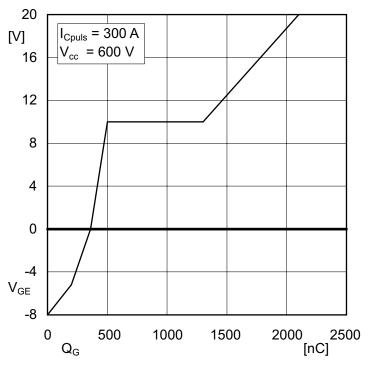
Figure 3.3.20 Gate charge characteristic of an IGBT
