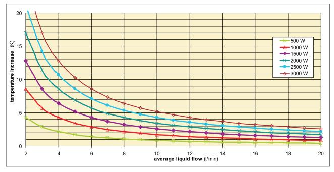
Figure 5.3.29 Temperature difference between water/glycol mixture flowing in/out as a function of the power dissipation and the volumetric flow rate,  $T_a = 25^{\circ}C$ , 50% glycol
