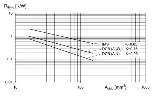
Figure 2.5.19 Dependency of thermal resistance  $R_{th(i-c)}$  on chip area  $A_{Chip}$  [37]
